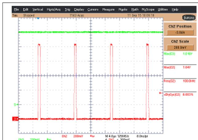
Figure 8-8. Supply Voltage 2.2 V, Peak Signal 1 V
