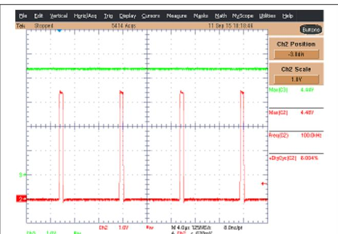
Figure 8-9. Supply Voltage 5 V Peak Signal 4.5 V
