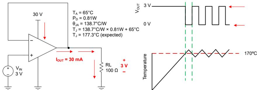
**Figure 7-4. Thermal Protection**
