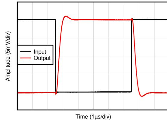
$C_L = 20\text{ pF}$ ,  $G = -1$ , 20-mV step response
