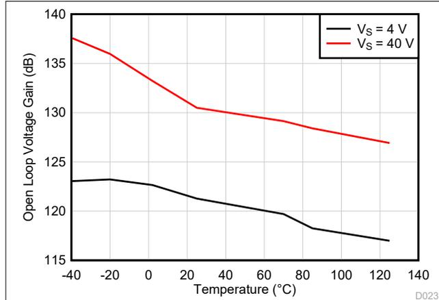
Figure 6-25. Open-Loop Voltage Gain vs Temperature (dB)
