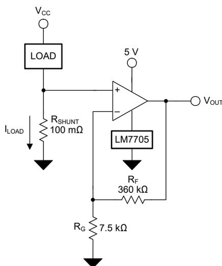
Figure 8-1. OPA4991-EP in a Low-Side, Current-Sensing Application
