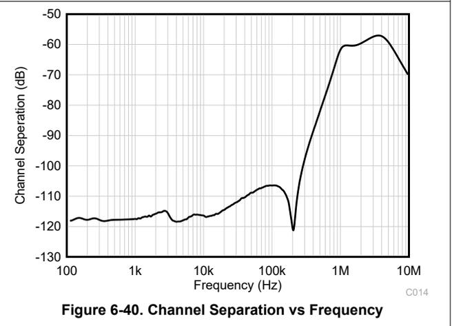
Figure 6-40. Channel Separation vs Frequency
