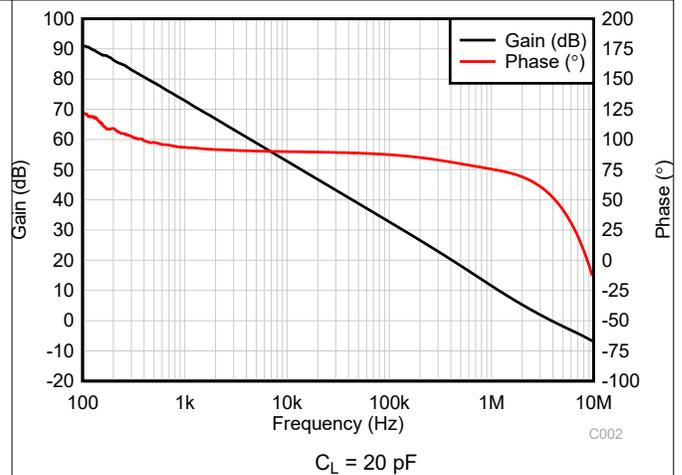
Figure 6-10. Open-Loop Gain and Phase vs Frequency
