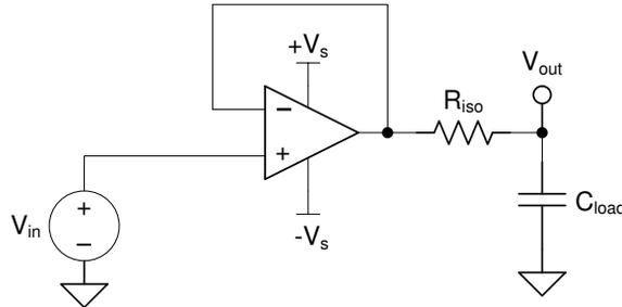
**Figure 7-7. Extending Capacitive Load Drive With the OPA4991-EP**
