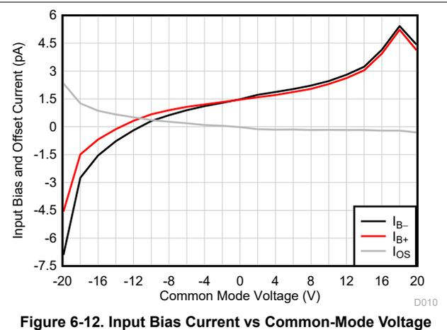
Figure 6-12. Input Bias Current vs Common-Mode Voltage
