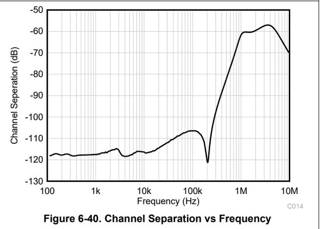
Figure 6-40. Channel Separation vs Frequency
