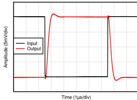
$C_L = 20\text{ pF}$ ,  $G = -1$ , 20-mV step response
