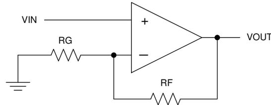
**Figure 8-3. Schematic Representation**
