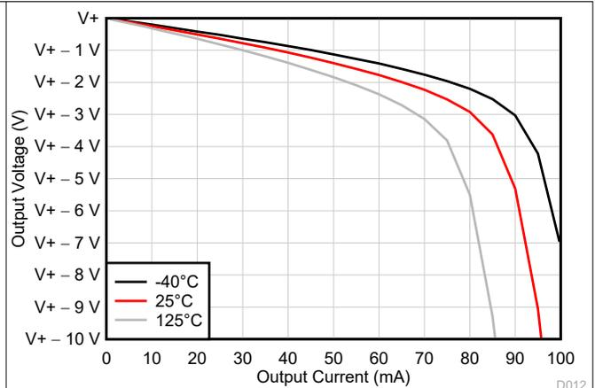
**Figure 6-14. Output Voltage Swing vs Output Current (Sourcing)**
