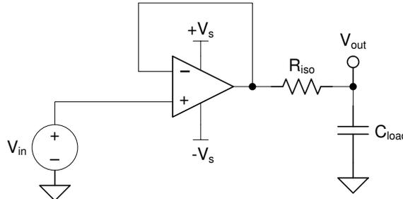
**Figure 7-7. Extending Capacitive Load Drive With the OPA4H199-SEP**
