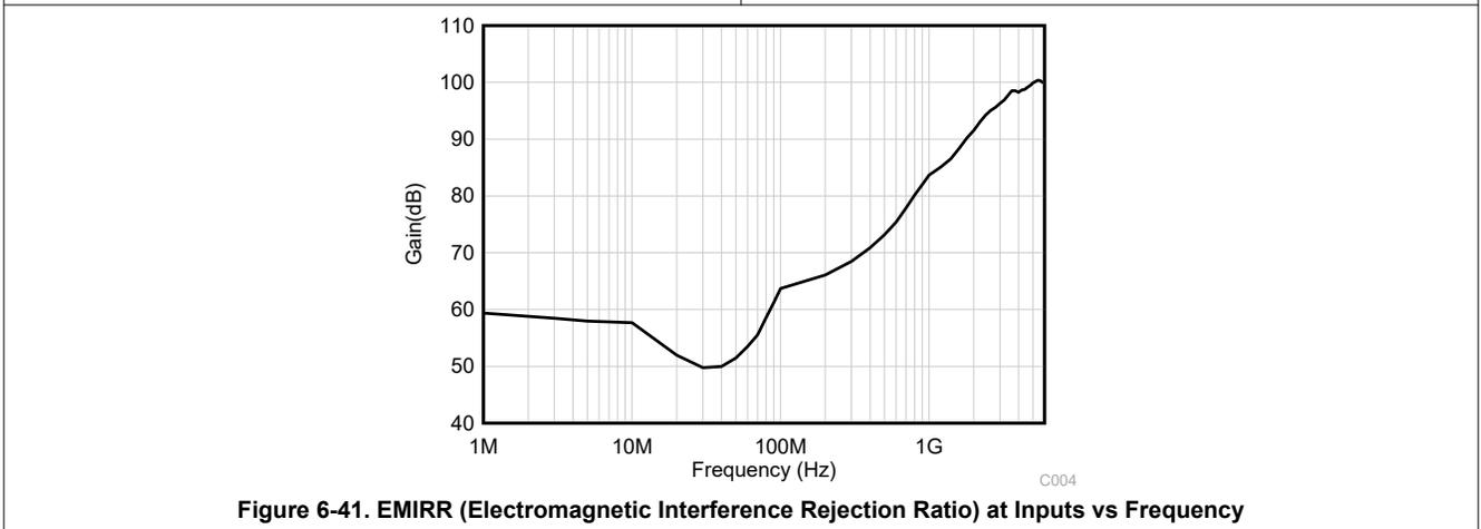
Figure 6-41. EMIRR (Electromagnetic Interference Rejection Ratio) at Inputs vs Frequency
