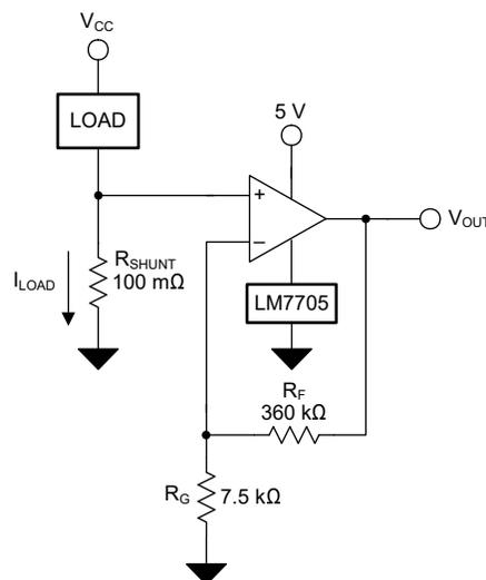
Figure 8-1. OPA4H199-SEP in a Low-Side, Current-Sensing Application
