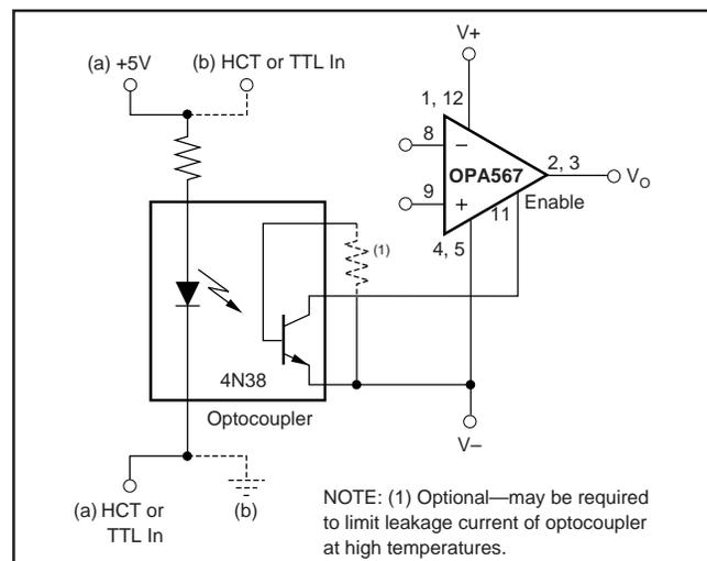
FIGURE 4. OPA567 Shutdown Configuration for Dual Supplies.
