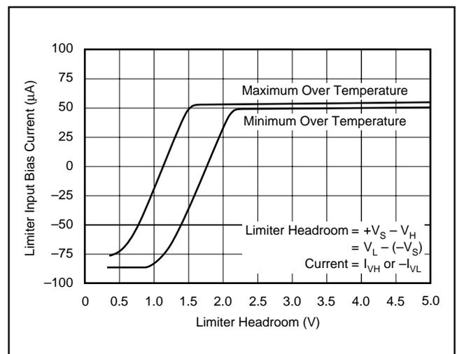
FIGURE 12. Limiter Bias Current vs Bias Voltage.
