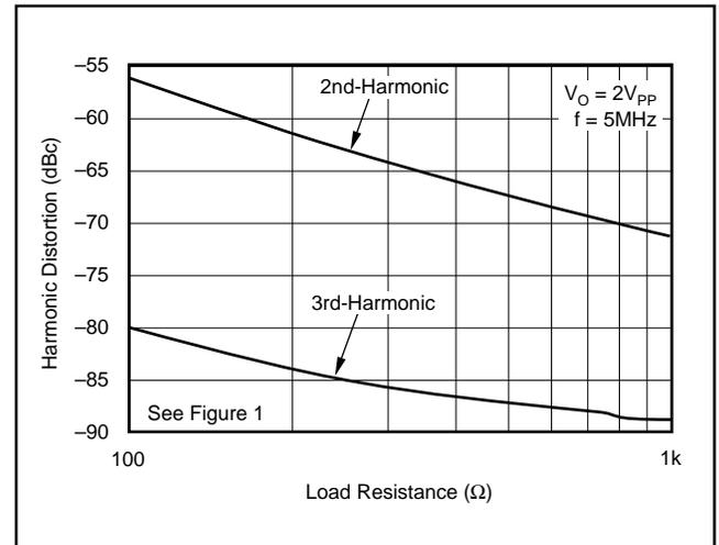
FIGURE 15. 5MHz Harmonic Distortion vs Load Resistance.
