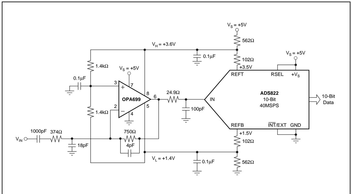
FIGURE 6. Single Supply, Limiting ADC Input Driver.
