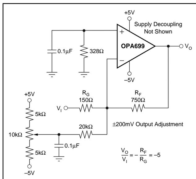
FIGURE 17. DC-Coupled, Inverting Gain of  $-5$ , with Offset Adjustment.
