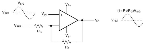
**Figure 8-1. Noninverting Amplifier**
