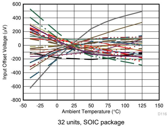
Figure 6-56. Input Offset Voltage vs Ambient Temperature
