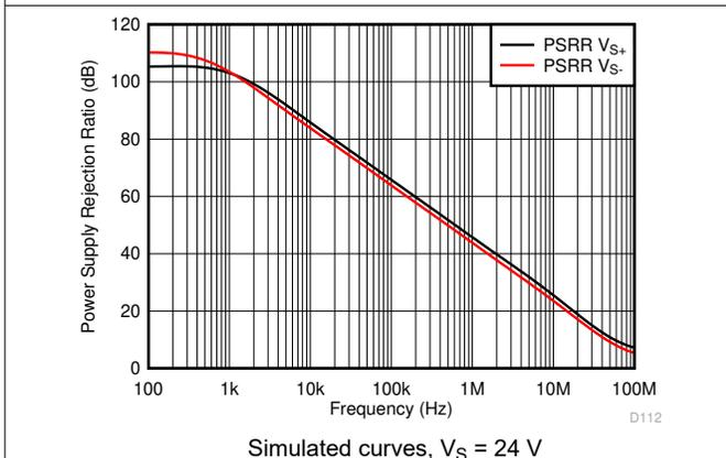
**Figure 6-52. Power Supply Rejection Ratio vs Frequency**
