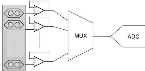
**Figure 8-16. Multichannel Sensor Interface Using Multiple Amplifiers**
