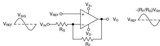
**Figure 8-4. Inverting Amplifier**
