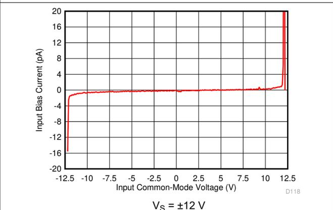
**Figure 6-53. Input Bias Current vs Input Common-Mode Voltage**
