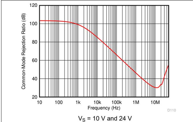
**Figure 6-50. Common-Mode Rejection Ratio vs Frequency**
