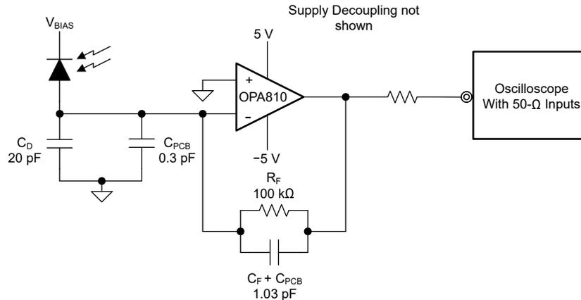
**Figure 8-12. Wideband, High-Sensitivity, Transimpedance Amplifier**
