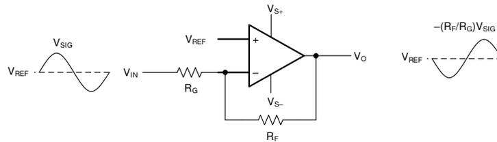
**Figure 8-2. Inverting Amplifier**
