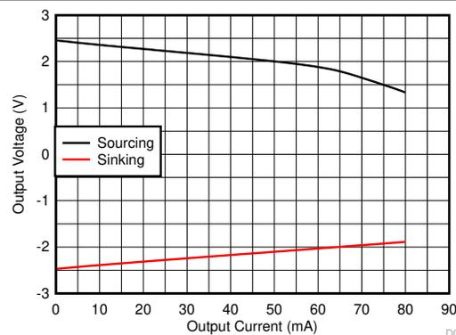
**Figure 6-39. Output Voltage Range vs Output Current**
