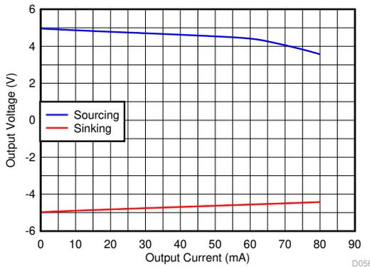
**Figure 6-15. Output Voltage vs Load Current**
