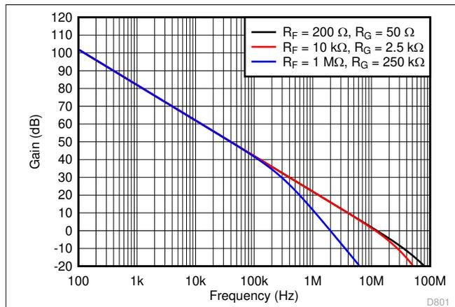
**Figure 8-6. Loop-Gain vs Frequency for Circuit of Figure 8-5**
