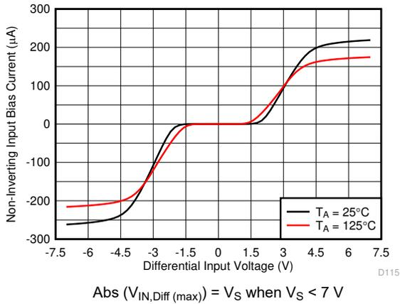
Figure 6-54. Input Bias Current vs Differential Input Voltage
