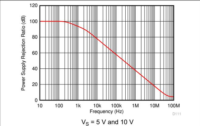
**Figure 6-51. Power Supply Rejection Ratio vs Frequency**
