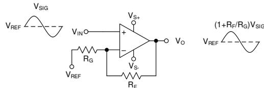
**Figure 8-3. Noninverting Amplifier**
