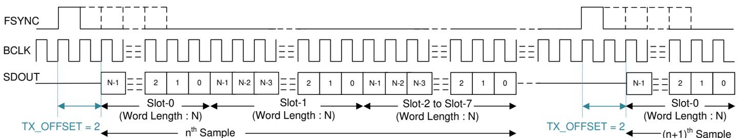
**Figure 7-2. TDM Mode Protocol Timing (TX\_OFFSET = 2)**
