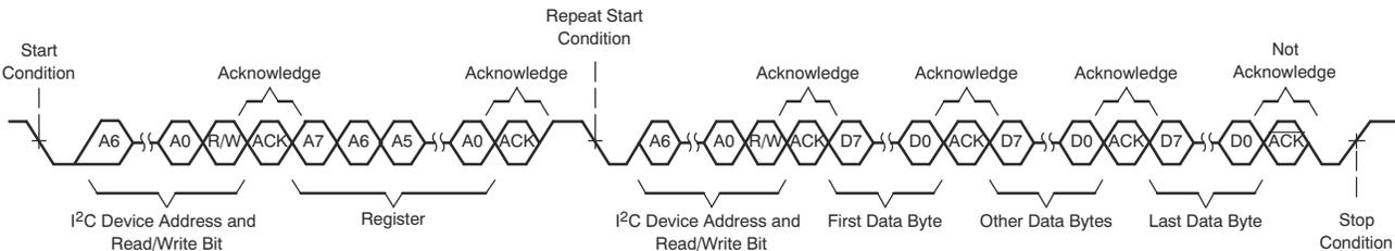
**Figure 7-70. I<sup>2</sup>C Multiple-Byte Read Transfer**
