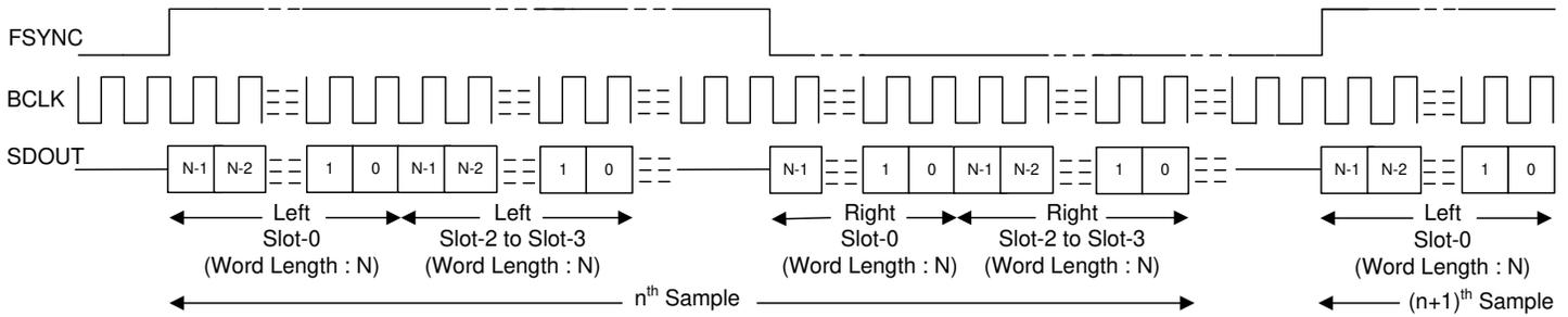
**Figure 7-9. LJ Mode Standard Protocol Timing (TX\_OFFSET = 0)**
