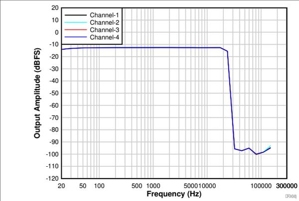
**Figure 6-12. Frequency Response With a -12-dBr Input**
