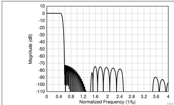
**Figure 7-19. Linear Phase Decimation Filter Magnitude Response**
