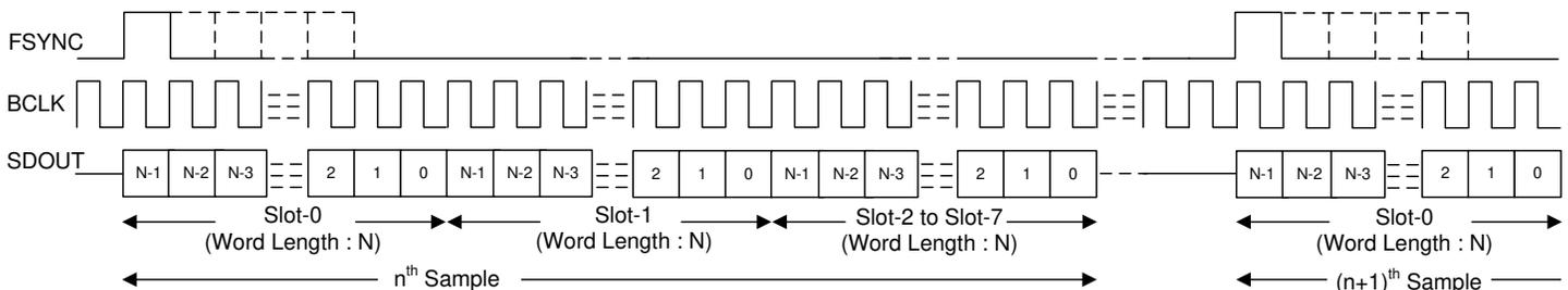
**Figure 7-1. TDM Mode Standard Protocol Timing (TX\_OFFSET = 0)**
