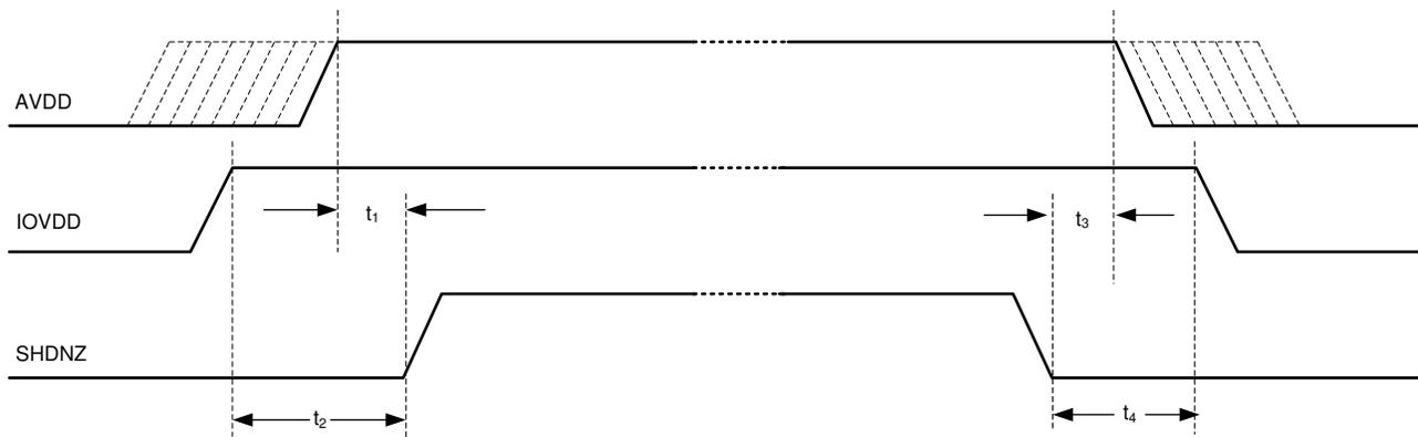
**Figure 9-5. Power-Supply Sequencing Requirement Timing Diagram**
