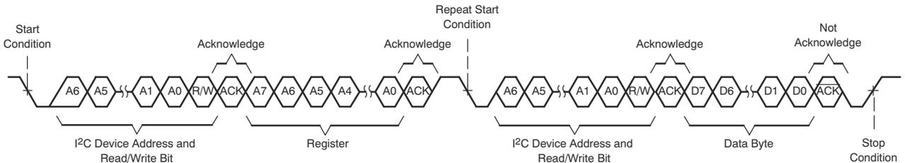
**Figure 7-69. I<sup>2</sup>C Single-Byte Read Transfer**
