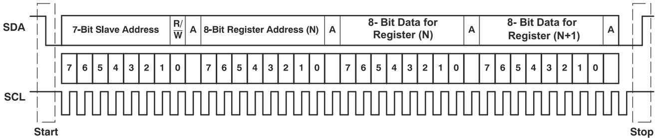
**Figure 7-66. Typical I<sup>2</sup>C Sequence**
