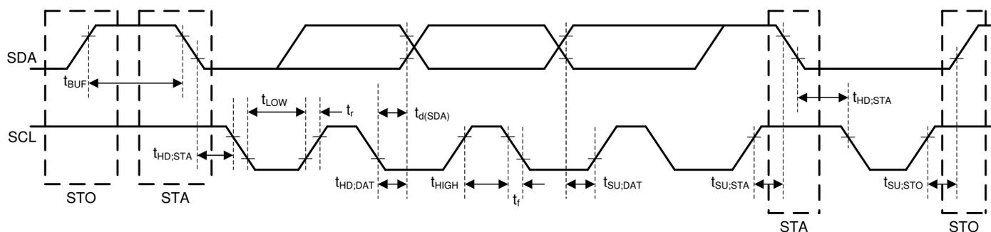
Figure 6-1. I<sup>2</sup>C Interface Timing Diagram
