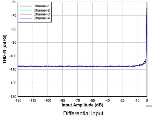
**Figure 6-5. THD+N vs Input Amplitude**
