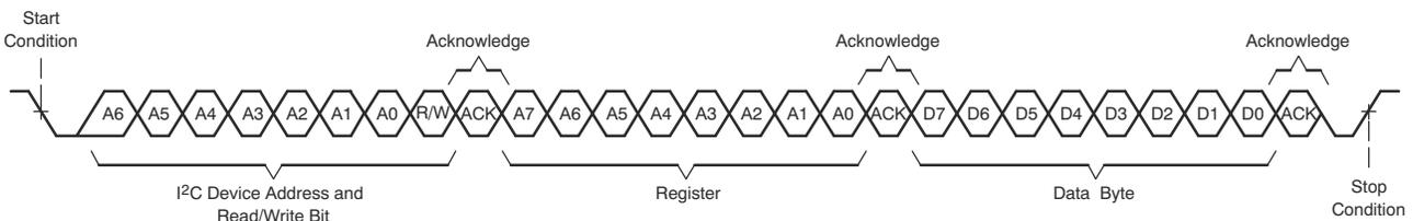
**Figure 7-67. I<sup>2</sup>C Single-Byte Write Transfer**
