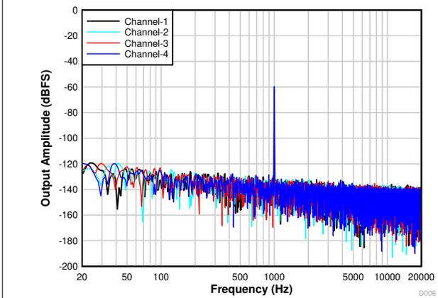
**Figure 6-15. FFT With a -60-dBr Input**
