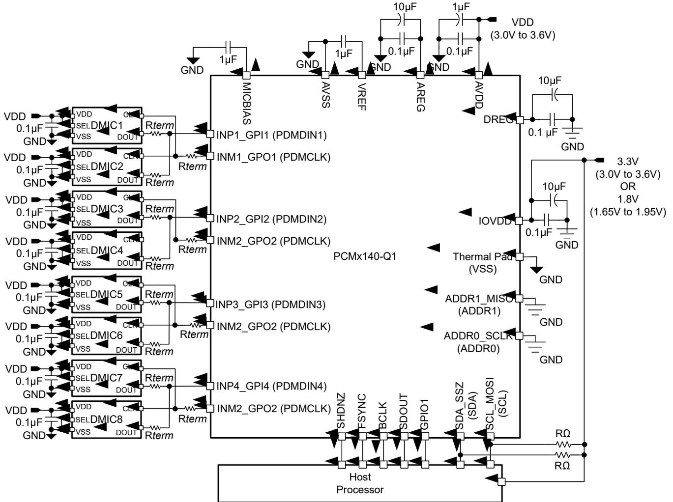
Figure 9-4. Eight-Channel Digital PDM Microphone Recording Diagram
