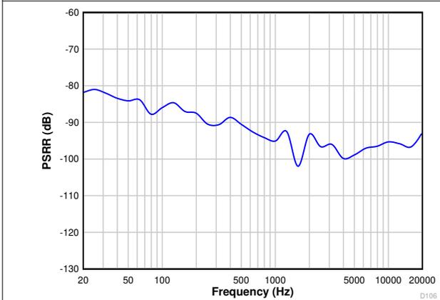
**Figure 6-13. Power-Supply Rejection Ratio vs Ripple Frequency With 100-mV<sub>PP</sub> Amplitude**
