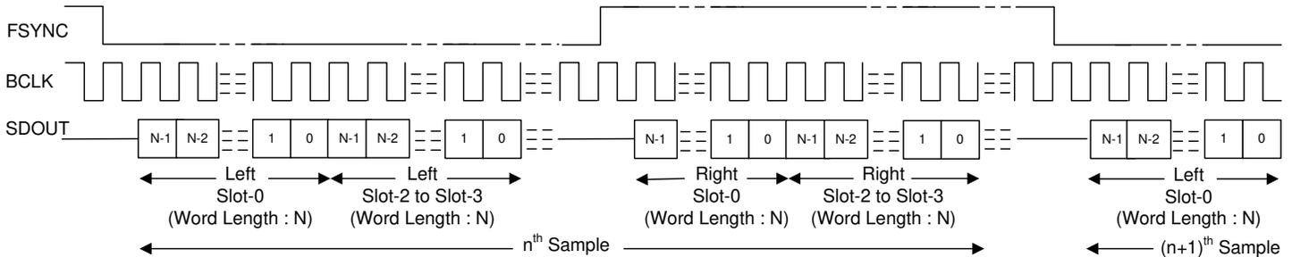
Figure 7-8. I²S Protocol Timing (TX\_OFFSET = 0 and BCLK\_POL = 1)
