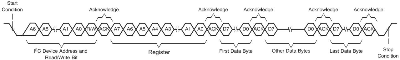
**Figure 7-68. I<sup>2</sup>C Multiple-Byte Write Transfer**
