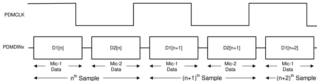
Figure 7-65. Digital PDM Microphone Protocol Timing Diagram
