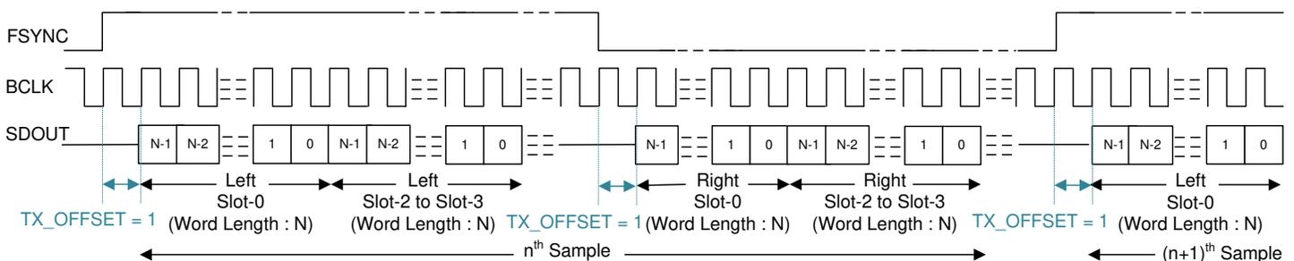
**Figure 7-12. LJ Protocol Timing (TX\_OFFSET = 1 and BCLK\_POL = 1)**
