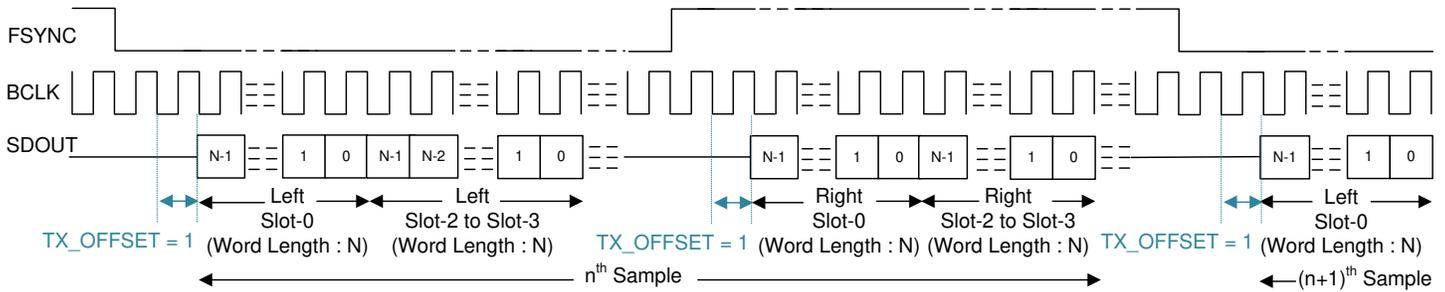
Figure 7-6. I²S Protocol Timing (TX\_OFFSET = 1)
