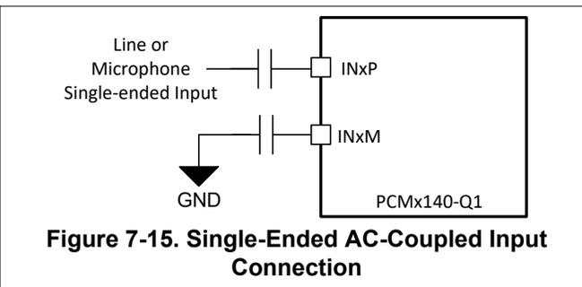
The device allows for flexibility in choosing the typical input impedance on INxP or INxM from 2.5 kΩ (default), 10 kΩ, and 20 kΩ based on the input source impedance. The higher input impedance results in slightly higher noise or lower dynamic range. Table 7-9 lists the configuration register settings for the input impedance for the record channel.
