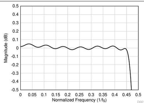
**Figure 7-20. Linear Phase Decimation Filter Pass-Band Ripple**
