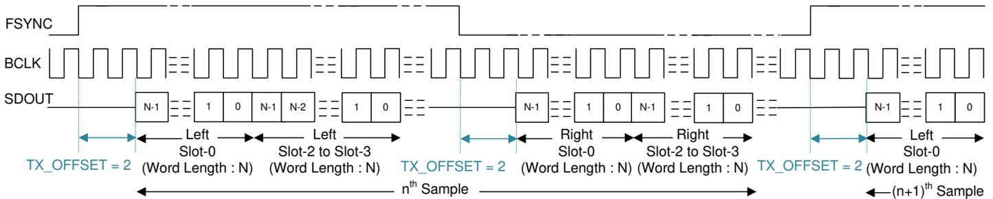
**Figure 7-10. LJ Protocol Timing (TX\_OFFSET = 2)**
