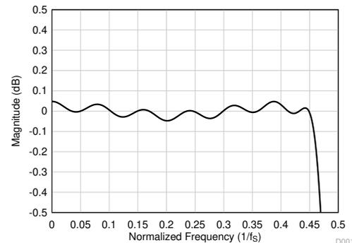
**Figure 8-26. Linear Phase Decimation Filter Pass-Band Ripple**
