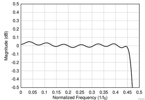
**Figure 8-22. Linear Phase Decimation Filter Pass-Band Ripple**
