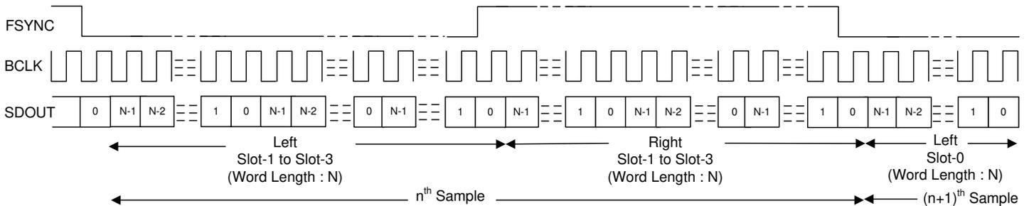
Figure 8-7. I<sup>2</sup>S Protocol Timing (No Idle BCLK Cycles, TX\_OFFSET = 0)
