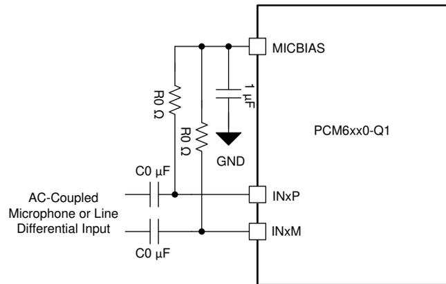
**Figure 8-16. AC-Coupled Microphone or Line Differential Input Connection**
