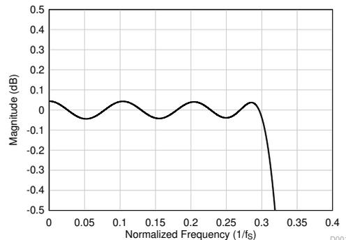
**Figure 8-34. Linear Phase Decimation Filter Pass-Band Ripple**
