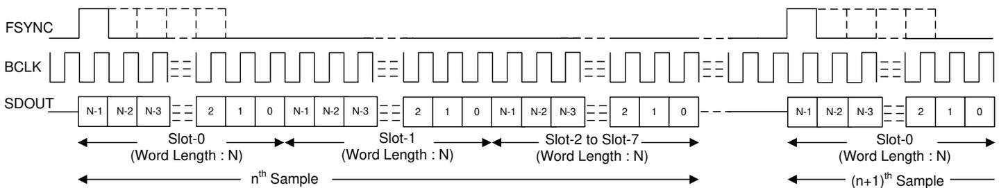
**Figure 8-4. TDM Mode Protocol Timing (TX\_OFFSET = 0 and BCLK\_POL = 1)**
