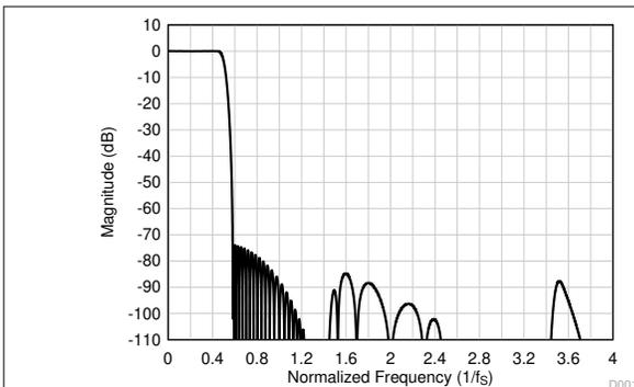
**Figure 8-29. Linear Phase Decimation Filter Magnitude Response**
