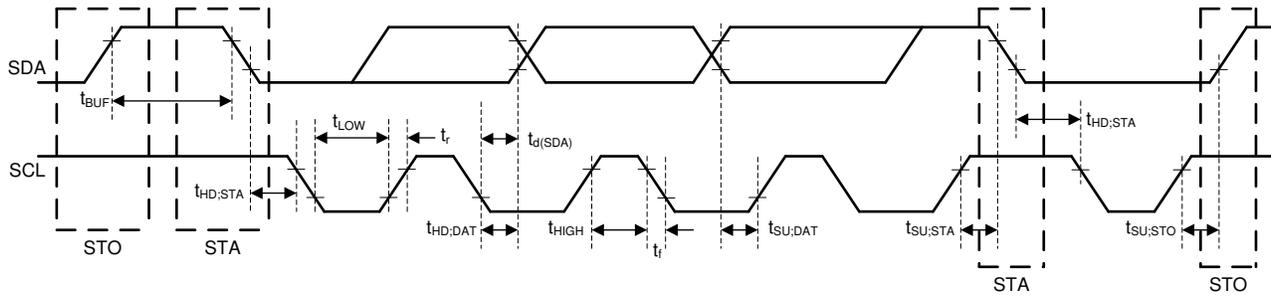
**Figure 7-1. I<sup>2</sup>C Interface Timing Diagram**
