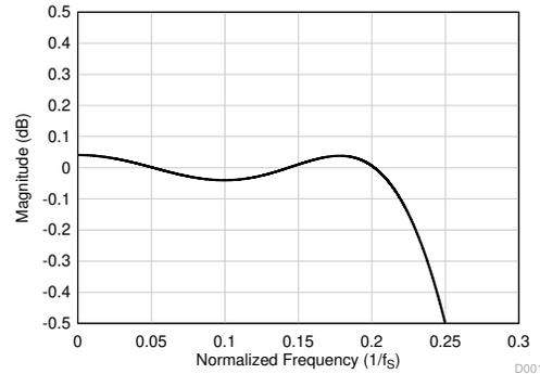
**Figure 8-36. Linear Phase Decimation Filter Pass-Band Ripple**
