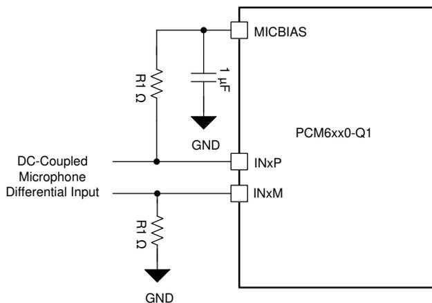
**Figure 8-14. DC-Coupled Microphone Differential Input Connection**
