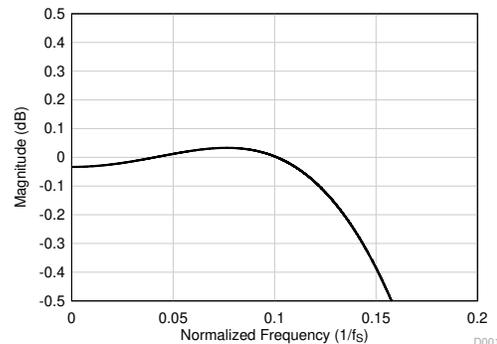
**Figure 8-38. Linear Phase Decimation Filter Pass-Band Ripple**
