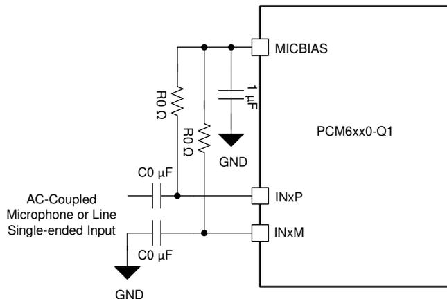
**Figure 8-17. AC-Coupled Microphone or Line Single-Ended Input Connection**
