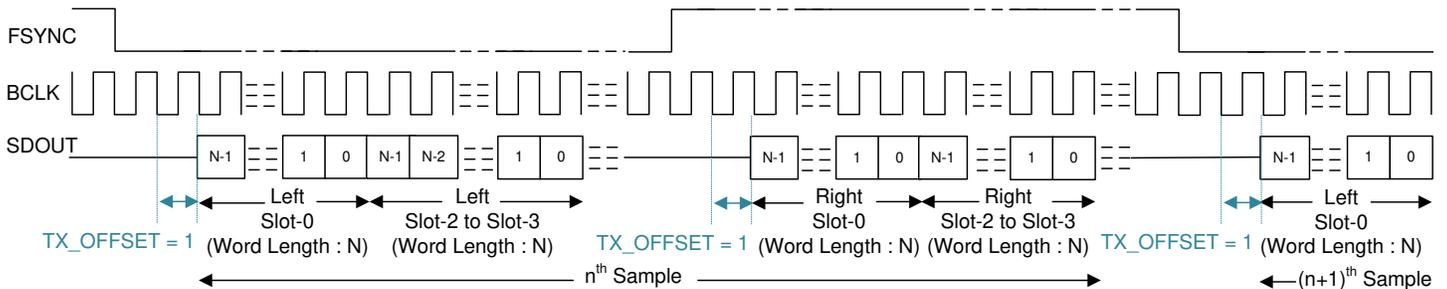
Figure 8-6. I<sup>2</sup>S Protocol Timing (TX\_OFFSET = 1)
