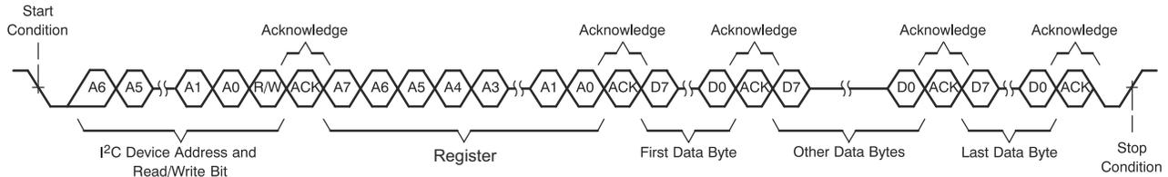
Figure 8-68. I<sup>2</sup>C Multiple-Byte Write Transfer
