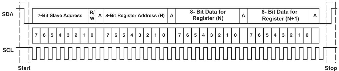
**Figure 8-66. Typical I<sup>2</sup>C Sequence**
