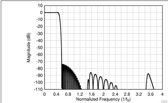
**Figure 8-31. Linear Phase Decimation Filter Magnitude Response**
