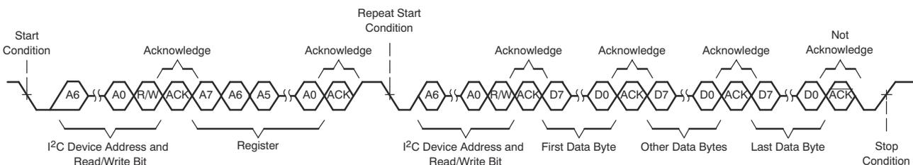
Figure 8-70. I<sup>2</sup>C Multiple-Byte Read Transfer
