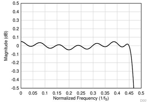
**Figure 8-32. Linear Phase Decimation Filter Pass-Band Ripple**
