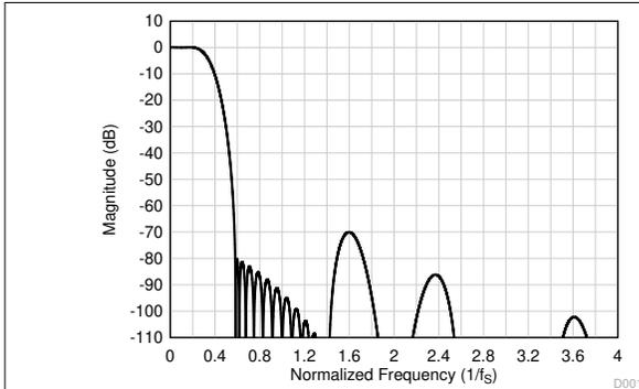
**Figure 8-35. Linear Phase Decimation Filter Magnitude Response**
