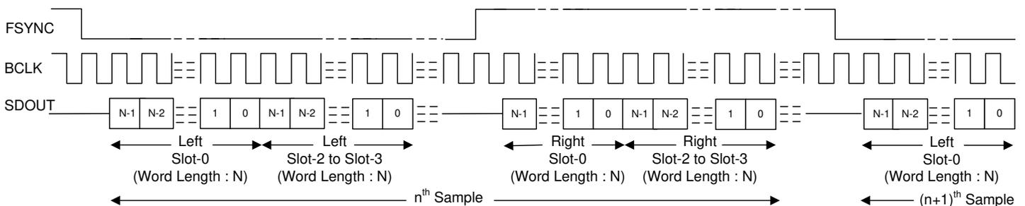
Figure 8-8. I<sup>2</sup>S Protocol Timing (TX\_OFFSET = 0 and BCLK\_POL = 1)
