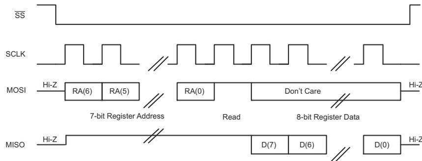
**Figure 8-72. SPI Single-Byte Read Transfer**
