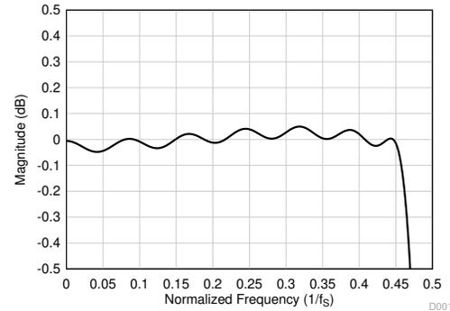
**Figure 8-24. Linear Phase Decimation Filter Pass-Band Ripple**
