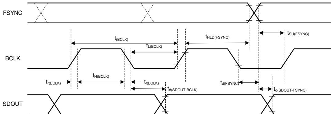
**Figure 7-3. TDM, I<sup>2</sup>S, LJ Interface Timing Diagram**
