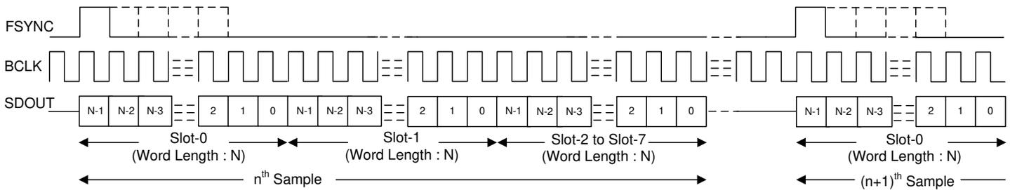
**Figure 8-1. TDM Mode Standard Protocol Timing (TX\_OFFSET = 0)**
