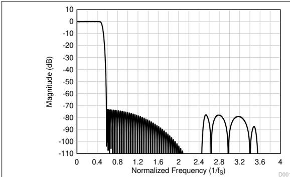
**Figure 8-23. Linear Phase Decimation Filter Magnitude Response**
