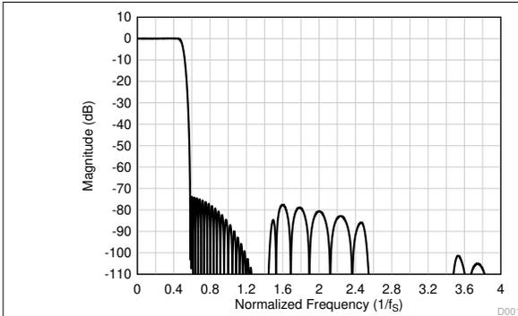
**Figure 8-27. Linear Phase Decimation Filter Magnitude Response**
