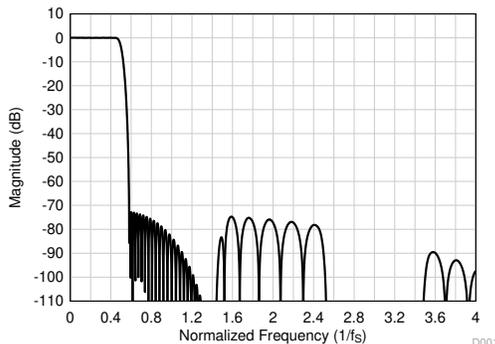
**Figure 8-21. Linear Phase Decimation Filter Magnitude Response**
