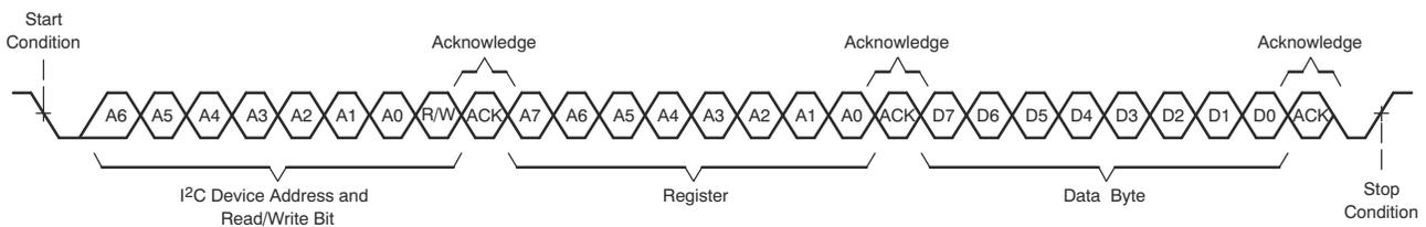
**Figure 8-67. I<sup>2</sup>C Single-Byte Write Transfer**
