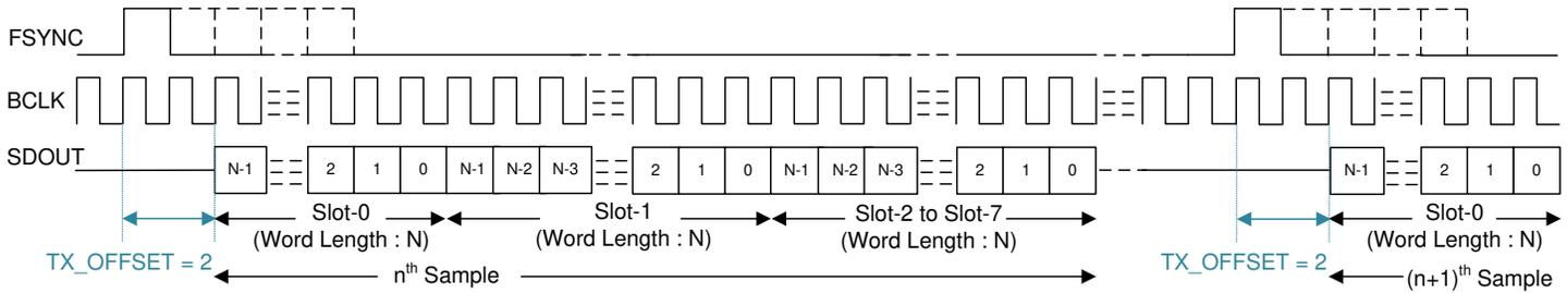
**Figure 8-2. TDM Mode Protocol Timing (TX\_OFFSET = 2)**
