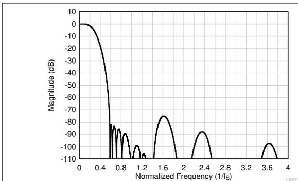
**Figure 8-37. Linear Phase Decimation Filter Magnitude Response**
