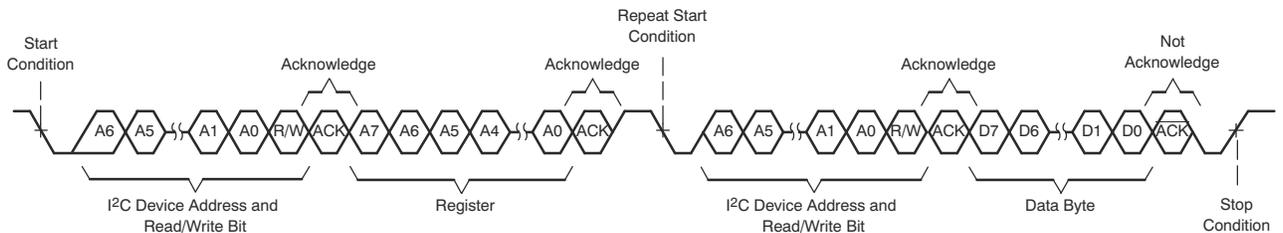
Figure 8-69. I<sup>2</sup>C Single-Byte Read Transfer
