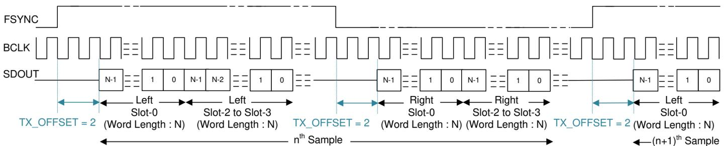
**Figure 8-10. LJ Protocol Timing (TX\_OFFSET = 2)**
