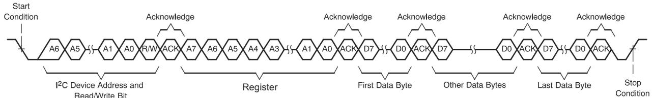
Figure 6-65. I<sup>2</sup>C Multiple-Byte Write Transfer
