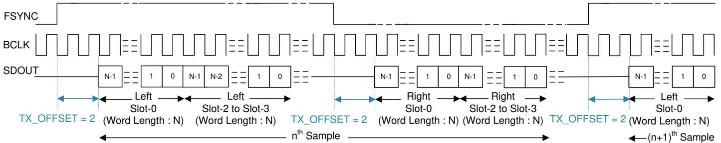
**Figure 6-10. LJ Protocol Timing (TX\_OFFSET = 2)**
