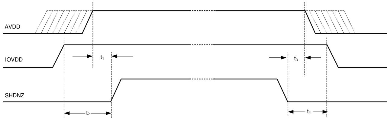
**Figure 9-1. Power-Supply Sequencing Requirement Timing Diagram**
