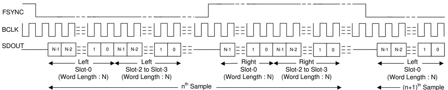
Figure 6-5. I<sup>2</sup>S Mode Standard Protocol Timing (TX\_OFFSET = 0)
