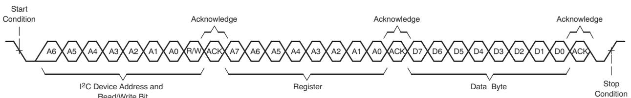
Figure 6-64. I<sup>2</sup>C Single-Byte Write Transfer
