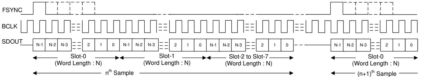
Figure 6-4. TDM Mode Protocol Timing (TX\_OFFSET = 0 and BCLK\_POL = 1)
