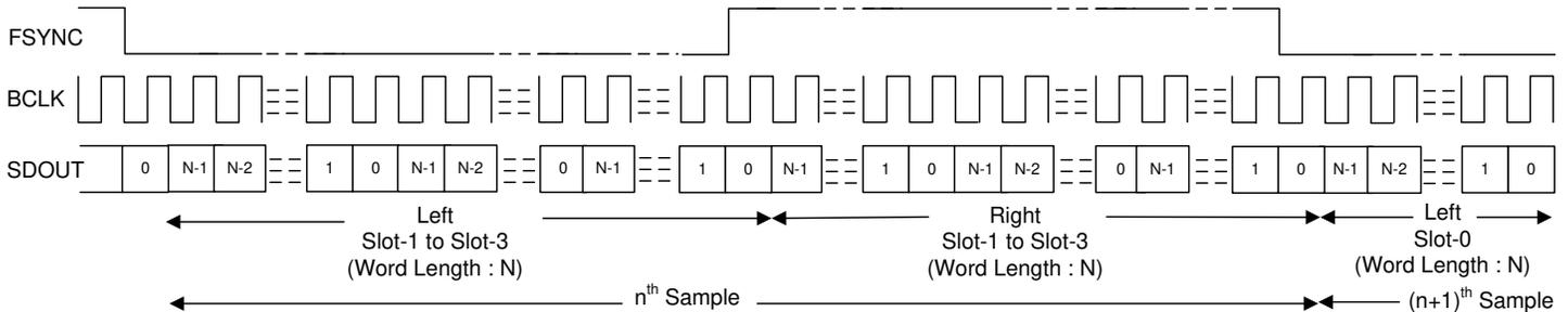
**Figure 6-7. I<sup>2</sup>S Protocol Timing (No Idle BCLK Cycles, TX\_OFFSET = 0)**
