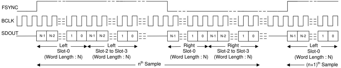
**Figure 6-9. LJ Mode Standard Protocol Timing (TX\_OFFSET = 0)**
