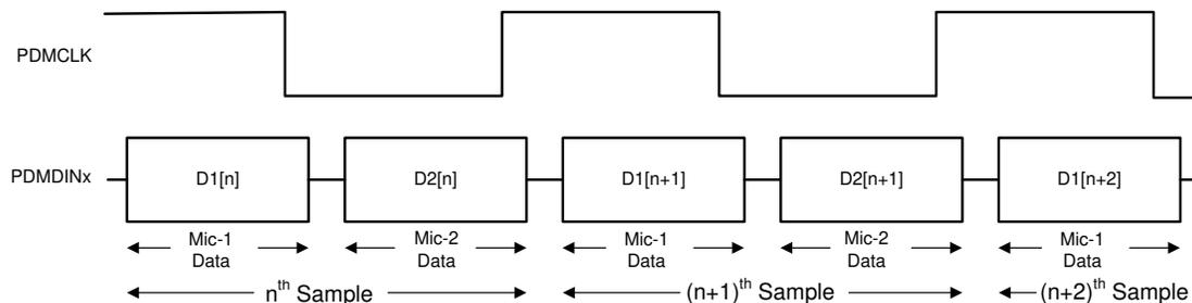
**Figure 6-15. Digital PDM Microphone Protocol Timing Diagram**
