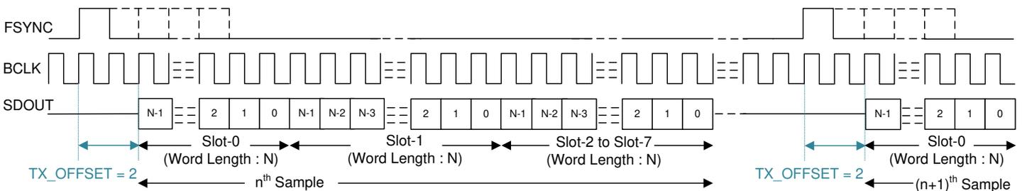
**Figure 6-2. TDM Mode Protocol Timing (TX\_OFFSET = 2)**
