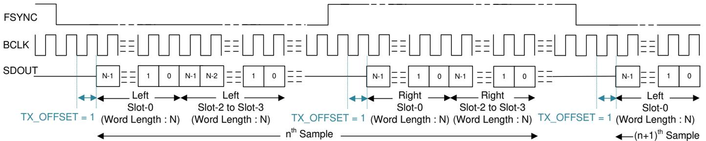
**Figure 6-6. I<sup>2</sup>S Protocol Timing (TX\_OFFSET = 1)**
