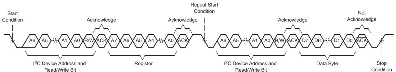
Figure 6-66. I<sup>2</sup>C Single-Byte Read Transfer
