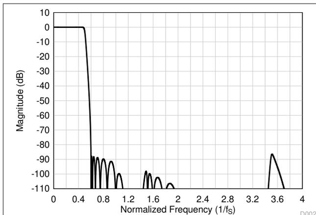
**Figure 6-43. Low-Latency Decimation Filter Magnitude Response**
