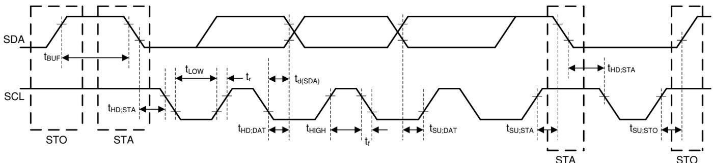
Figure 5-1. I<sup>2</sup>C Interface Timing Diagram
