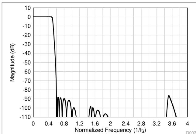
**Figure 6-55. Ultra-Low-Latency Decimation Filter Magnitude Response**
