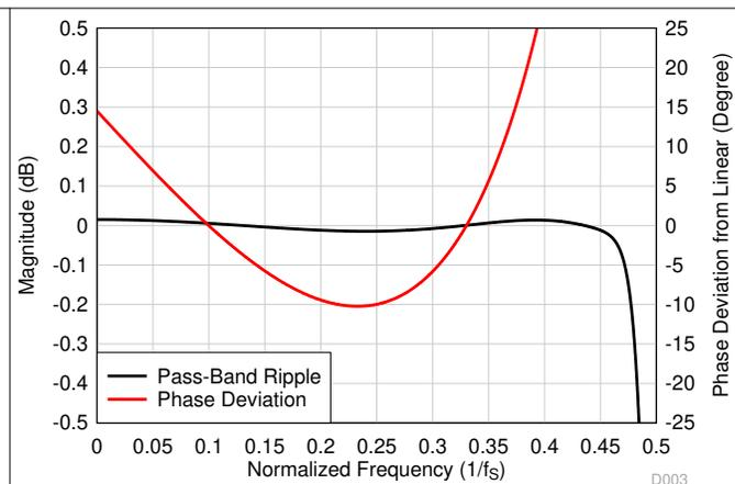
**Figure 6-56. Ultra-Low-Latency Decimation Filter Pass-Band Ripple and Phase Deviation****Table 6-37. Ultra-Low-Latency Decimation Filter Specifications**
