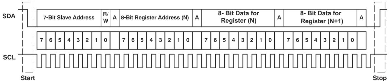
Figure 6-63. Typical I<sup>2</sup>C Sequence
