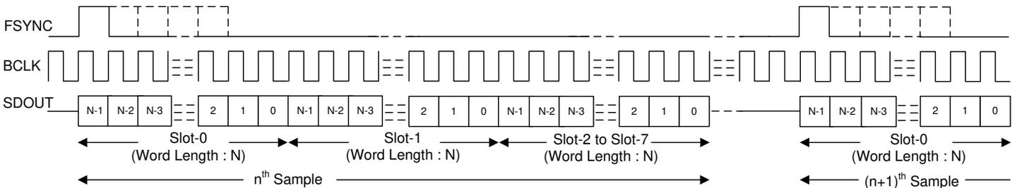
**Figure 6-1. TDM Mode Standard Protocol Timing (TX\_OFFSET = 0)**
