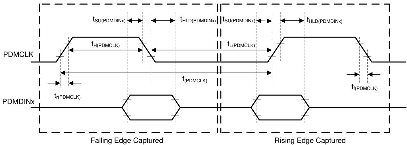
**Figure 5-4. PDM Digital Microphone Interface Timing Diagram**
