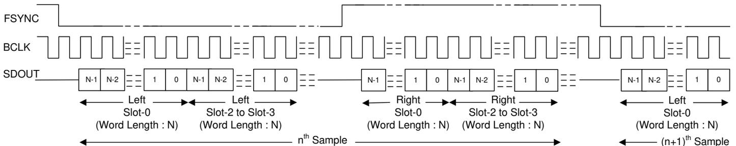
**Figure 6-8. I<sup>2</sup>S Protocol Timing (TX\_OFFSET = 0 and BCLK\_POL = 1)**
