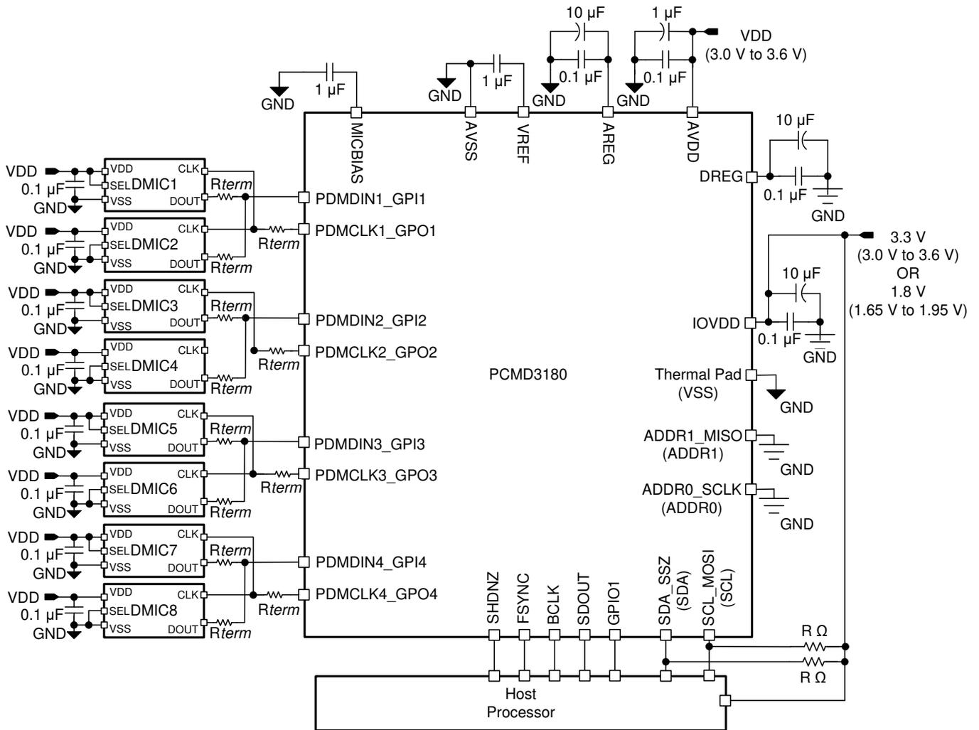
Figure 8-1. Eight-Channel Digital PDM Microphone Recording Diagram
