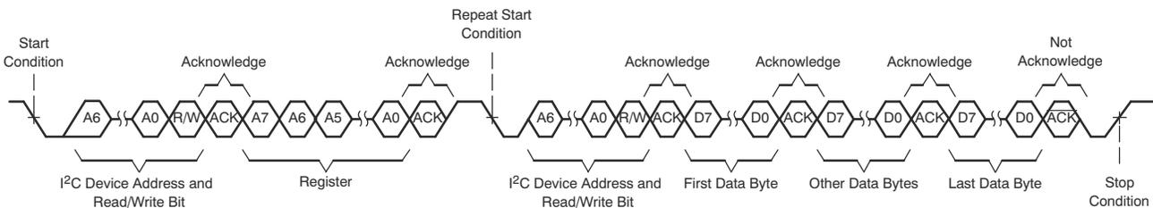
Figure 6-67. I<sup>2</sup>C Multiple-Byte Read Transfer
