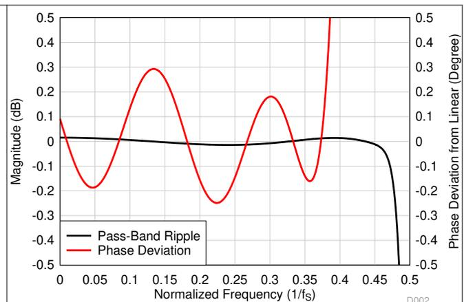
**Figure 6-44. Low-Latency Decimation Filter Pass-Band Ripple and Phase Deviation****Table 6-31. Low-Latency Decimation Filter Specifications**
