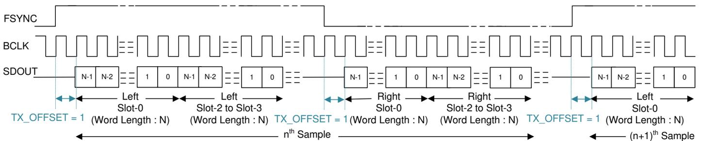
**Figure 6-12. LJ Protocol Timing (TX\_OFFSET = 1 and BCLK\_POL = 1)**
