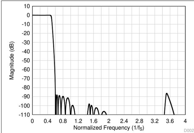
**Figure 6-45. Low-Latency Decimation Filter Magnitude Response**
