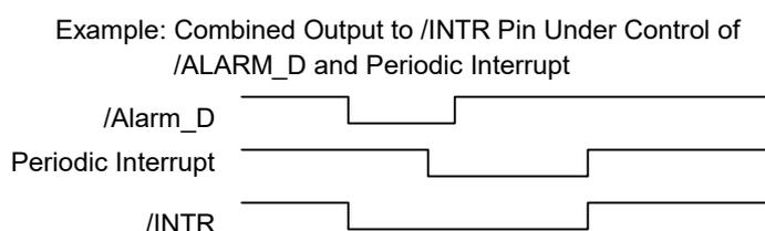
In this event, which type of interrupt signal is output from the /INTR pin can be confirmed by reading the DAFG, and CTFG bit settings in the Control Register 2.
