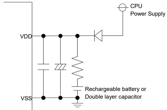
\*Set bypass capacitors as close as possible to the IC, use a capacitor for high frequency and another capacitor for low frequency in parallel.
