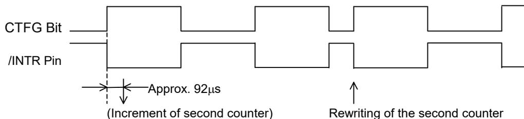
In the pulse mode, the increment of the second counter is delayed by approximately 92 µs from the falling edge of clock pulses. Consequently, time readings immediately after the falling edge of clock pulses may appear to lag behind the time counts of the real-time clocks by approximately 1 second. Rewriting the second counter will reset the other time counters of less than 1 second, driving the /INTR pin low.
