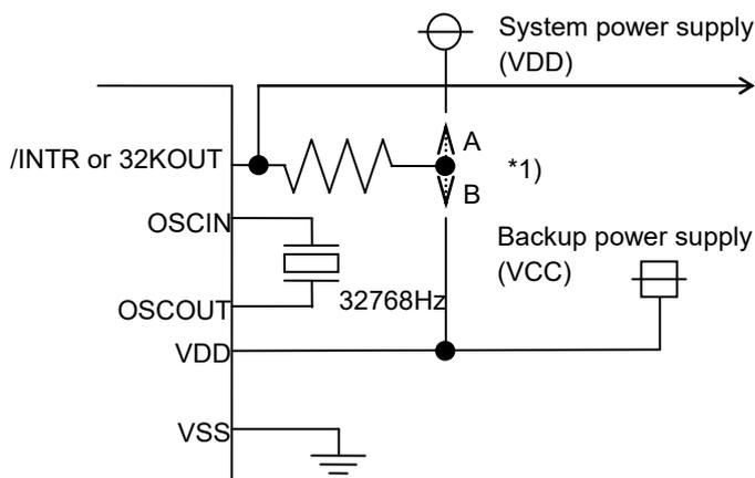
\*1) Depending on whether the /INTR or 32KOUT pins are to be used during battery backup, it should be connected to a pull-up resistor at the following different positions:
