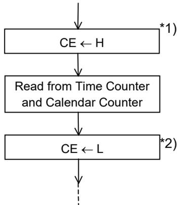
\*1) When writing to clock and calendar counters, do not insert Stop Condition until all times from second to year have been written to prevent error in writing time. (Detailed "P.26 Considerations in Reading and Writing Time Data under special condition".
