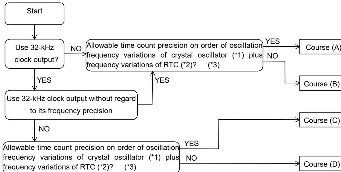
\* 1) Generally, crystal oscillators for commercial use are classified in terms of their center frequency depending on their load capacitance (CL) and further divided into ranks on the order of  $\pm 10$ ,  $\pm 20$ , and  $\pm 50$ ppm depending on the degree of their oscillation frequency variations.
