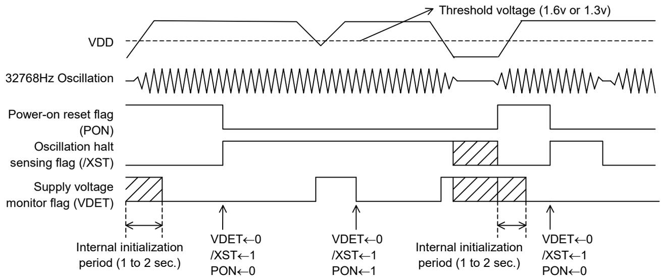
When the PON bit is set to 1 in the control register 2, the DEV, F6 to F0, WALE, DALE, /12-24, /CLEN2, TEST, CT2, CT1, CT0, VDSL, VDET, /CLEN1, CTFG, WAFG, and DAFG bits are reset to 0 in the oscillation adjustment register, the control register 1, and the control register 2. The PON bit is also set to 1 at power-on from 0v.
