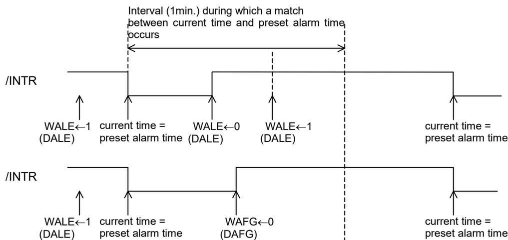
After setting WALE(DALW) to 0, Alarm registers is set to current time, and WALE(DALE) is set to 1, /INTR will be not driven to “L” immediately, /INTR will be driven to “L” at next alarm setting time.
