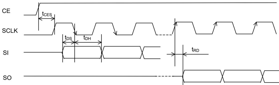
Conversely, when the SCLK pin is held high in the low to high transition of the CE pin, the models will select the timing with which the SO pin output is synchronized with the falling edge of the SCLK pin input, and the SI pin input is synchronized with the rising edge of the SCLK pin input, as illustrated in the timing chart below.
