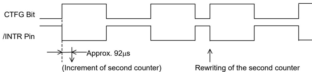
In the pulse mode, the increment of the second counter is delayed by approximately 92 µs from the falling edge of clock pulses. Consequently, time readings immediately after the falling edge of clock pulses may appear to lag behind the time counts of the real-time clocks by approximately 1 second. Rewriting the second counter will reset the other time counters of less than 1 second, driving the /INTR pin low.
