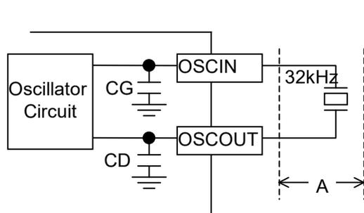
Typical externally-equipped element
