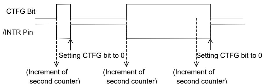
\*1), \*2) When the oscillation adjustment circuit is used, the interrupt cycle will fluctuate once per 20sec. as
