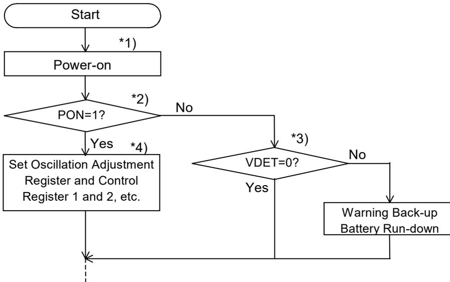
\*1) After power-on from 0 volt, the start of oscillation and the process of internal initialization require a time span on 1 to 2seconds, so that access should be done after the lapse of this time span or more.
