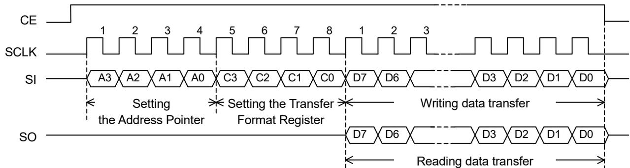
Two types of data transfer formats are available for reading data transfer and writing data transfer each.
