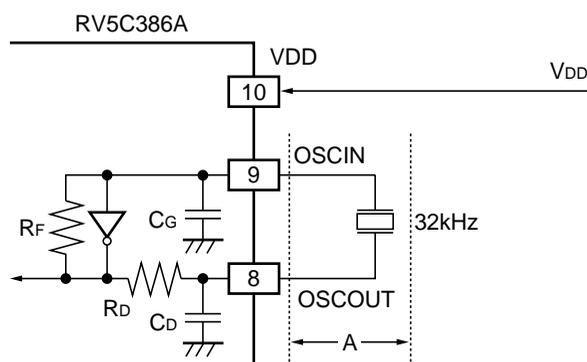
Typical externally-equipped element
