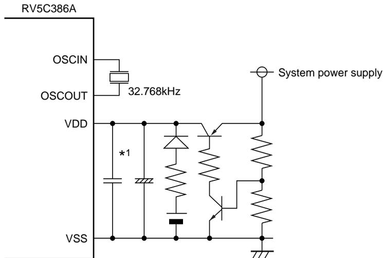
\*1) Install bypass capacitors for high-frequency and low-frequency applications in parallel in close vicinity to the RV5C386A .
