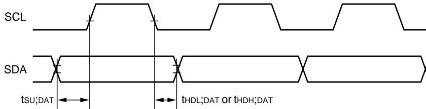
The SCL and SDA pins are at the “H” level when no data transmission is made. Changing the SDA from “H” to “L” when the SCL is “H” activates the start condition and access is started. Changing the SDA from “L” to “H” when the SCL is “H” activates stop condition and accessing stopped. Generation of start and stop conditions are always made by the master (see the figure below).
