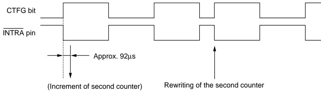
\*) In the pulse mode, the increment of the second counter is delayed by approximately 92μs from the falling edge of clock pulses. Consequently, time readings immediately after the falling edge of clock pulses may appear to lag behind the time counts of the real-time clocks by approximately 1 second. Rewriting the second counter will reset the other time counters of less than 1 second, driving the INTRA pin low.
