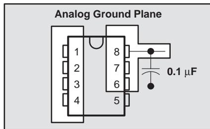
Figure 26. Power-Supply Bypassing
