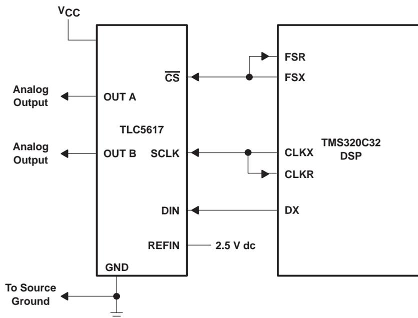
Figure 22. Interfacing The TLC5617 To TMS320C32 DSP
