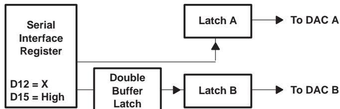
**Figure 19. Latch A Write, Latch B Update**
