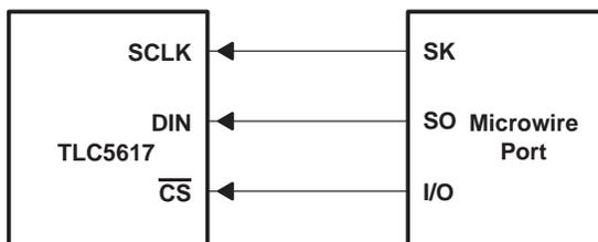
**Figure 23. Microwire Connection**
