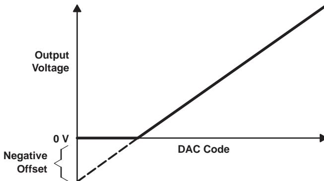
**Figure 25. Effect of Negative Offset (Single Supply)**
