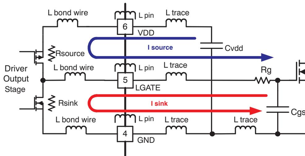
Figure 28. MOSFET Drive Paths and Main Circuit Parasitics
