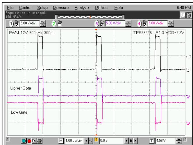
Figure 23. 12-V PWM Pulse at  $V_{DD} = 7.2\text{ V}$
