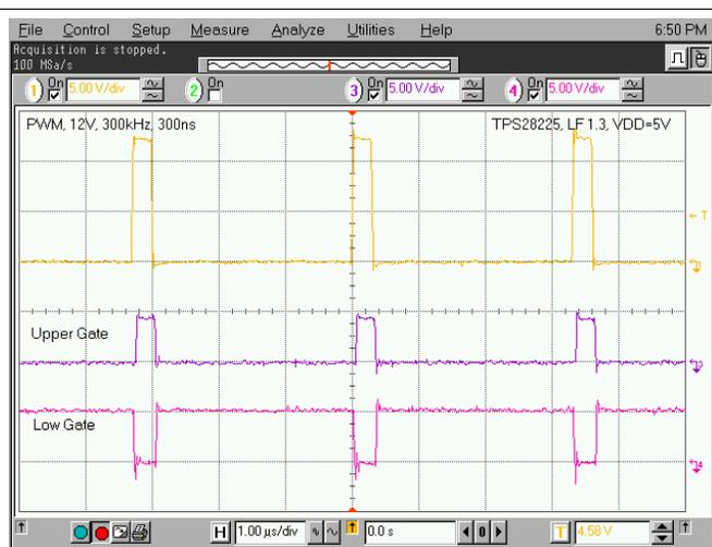
Figure 24. 12-V PWM Pulse at  $V_{DD} = 5\text{ V}$
