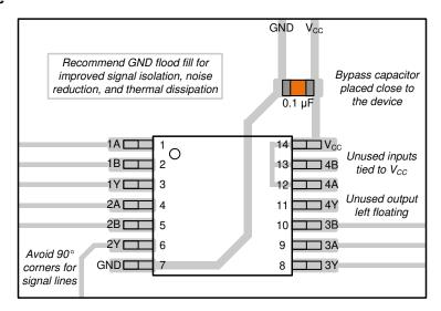
Figure 8-3. Example Layout for the SN74AHC32Q-Q1
