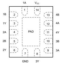
Figure 4-2. SN74AHC32 BQA Package, 14-Pin (Top View)
