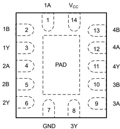
**Figure 4-1. BQA Package, 14-Pin WQFN (Top View)**
