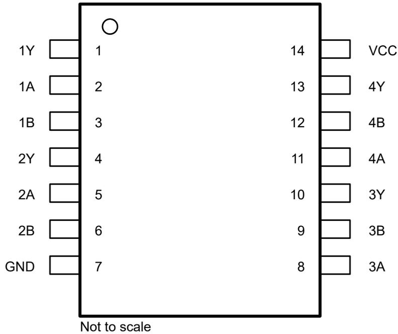
**Figure 4-1. PW Package, 14-Pin TSSOP (Top View)**
