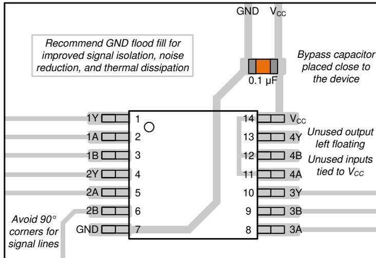
**Figure 8-3. Example Layout for the SN74LV4T02-EP**
