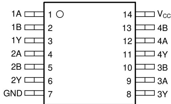
Figure 4-1. PW Package, 14-Pin TSSOP (Top View)
