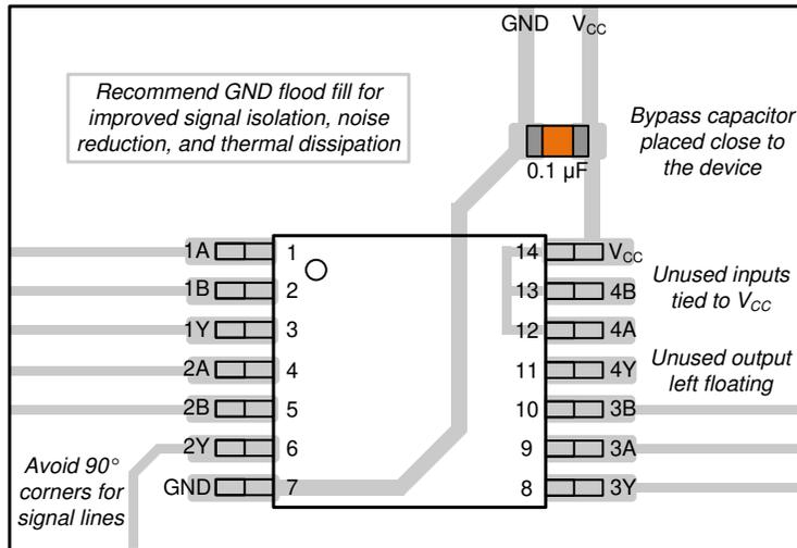
**Figure 8-3. Example Layout for the SN74LV4T32-EP**
