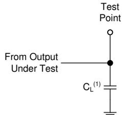
(1)  $C_L$  includes probe and test-fixture capacitance.
