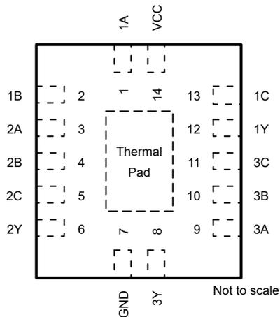
**Figure 4-1. SN74LVC11A-Q1 BQA Package, 14-Pin WQFN (Top View)**
