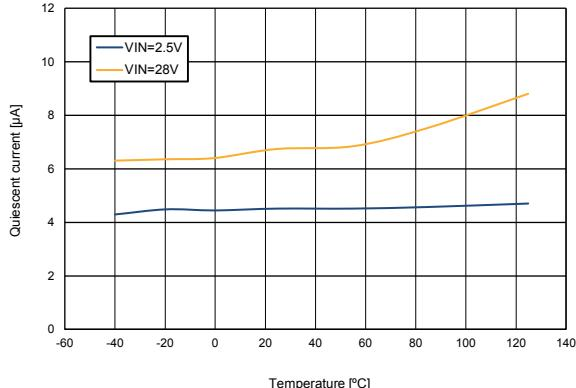
**Figure 15. Quiescent current vs. temperature ( $I_{OUT} = 300 \text{ mA}$ )**
