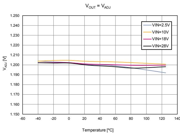
Figure 7. Reference voltage vs. load current and temperature
