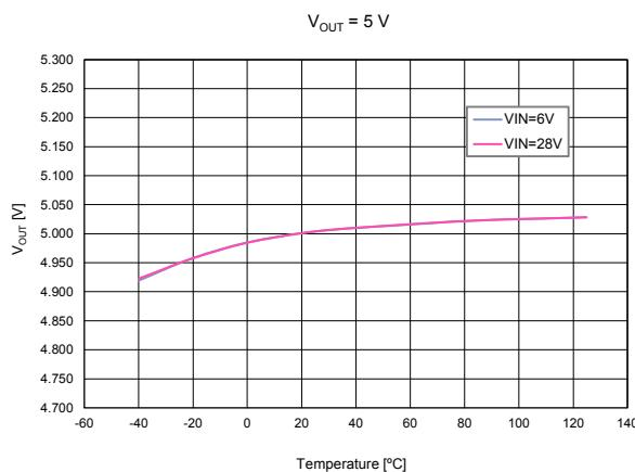
Figure 9. Output voltage vs. temperature ( $I_{OUT} = 300$  mA)
