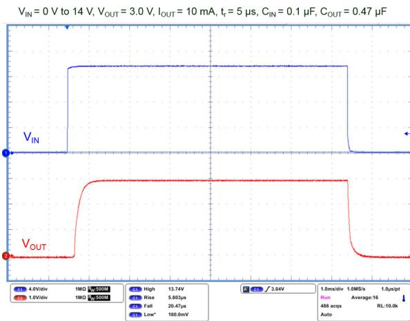
**Figure 25. Enable transient**
