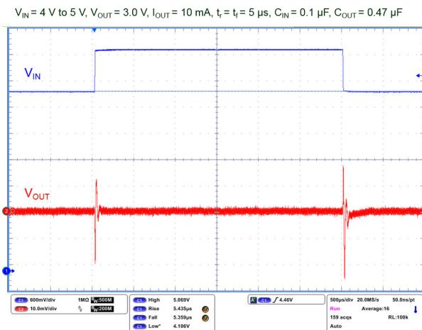
**Figure 23. Load transient**
