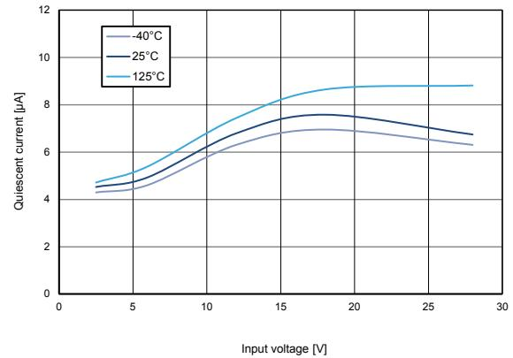
**Figure 14. Quiescent current vs. temperature ( $I_{OUT} = 0 \text{ mA}$ )**
