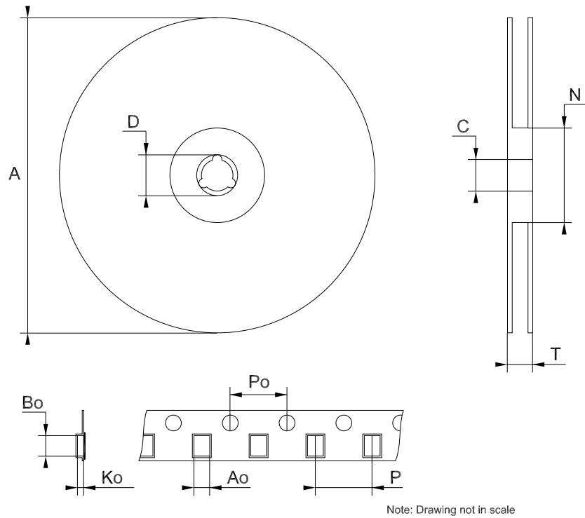
Table 8. SOT23-5L tape and reel mechanical data
