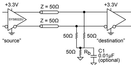
**Figure 5. Three-Resistor “Y-Termination”**
