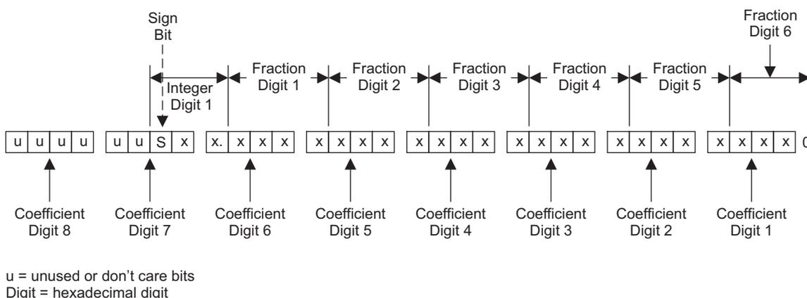
Figure 37. Alignment of 3.23 Coefficient in 32-Bit I2C Word
