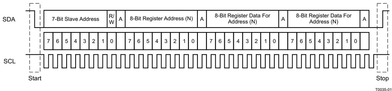
Figure 27. Typical I<sup>2</sup>C Sequence
