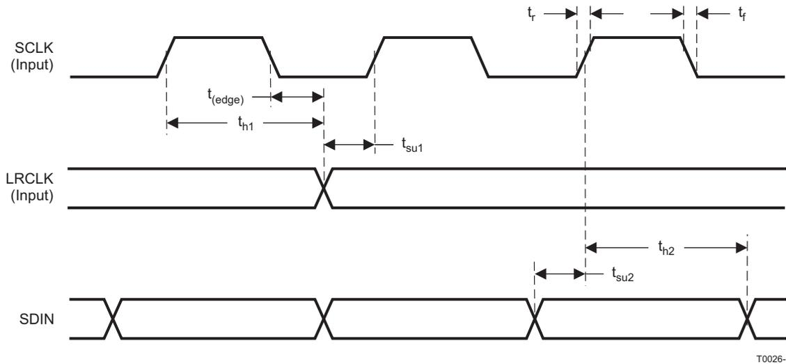
Figure 3. Slave Mode Serial Data Interface Timing
