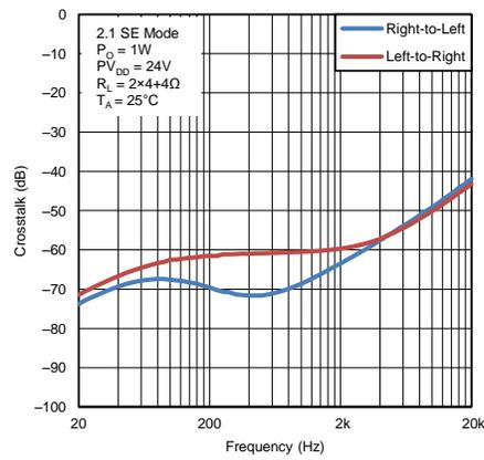
**Figure 17. Crosstalk vs Frequency (2.1 SE Mode)**
