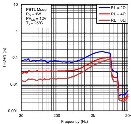
Figure 36. Total Harmonic Distortion vs Frequency (PBTL Mode)
