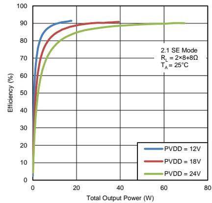
Figure 12. Efficiency vs Total Output Power (2.1 SE Mode)
