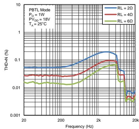
Figure 37. Total Harmonic Distortion vs Frequency (PBTL Mode)
