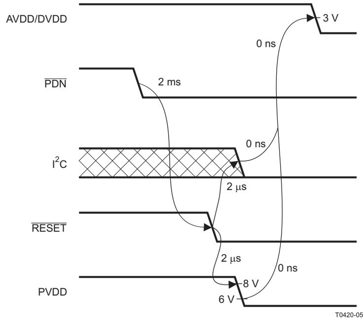
Figure 70. Power-Loss Sequence
