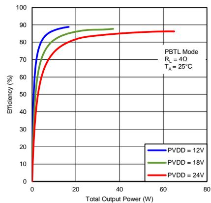
Figure 39. Efficiency vs Output Power (PBTL Mode)
