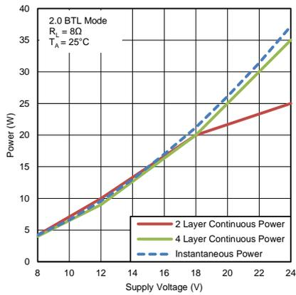
**Figure 30. Power vs Supply Voltage (2.0 BTL Mode)**
