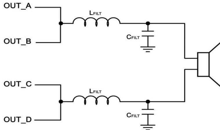
Figure 58. Post-Filter PBTL
