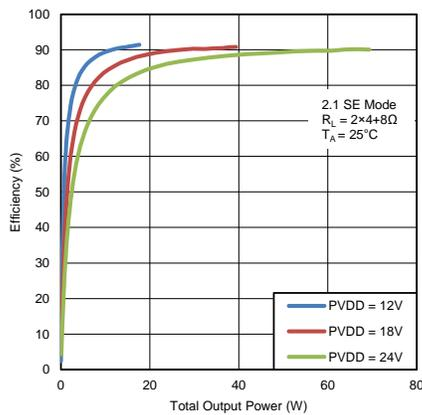
Figure 13. Efficiency vs Total Output Power (2.1 SE Mode)
