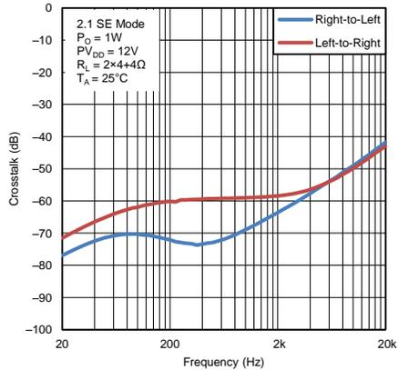
Figure 15. Crosstalk vs Frequency (2.1 SE Mode)
