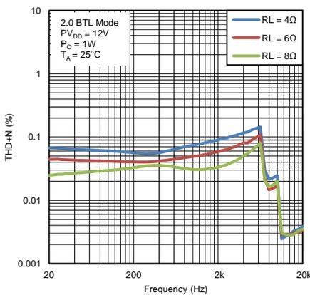
Figure 22. Total Harmonic Distortion vs Frequency (2.0 BTL Mode)
