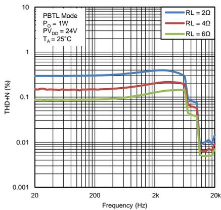
Figure 38. Total Harmonic Distortion vs Frequency (PBTL Mode)
