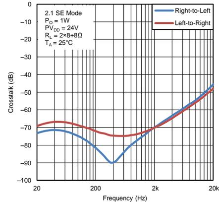
Figure 16. Crosstalk vs Frequency (2.1 SE Mode)
