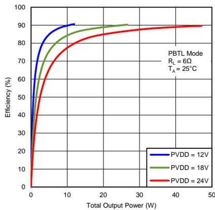
Figure 40. Efficiency vs Output Power (PBTL Mode)
