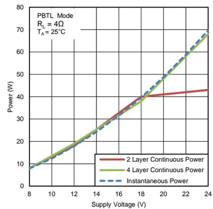
Figure 41. Power vs Supply Voltage (PBTL Mode)
