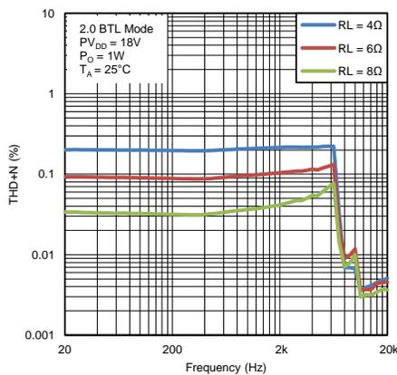
Figure 23. Total Harmonic Distortion vs Frequency (2.0 BTL Mode)
