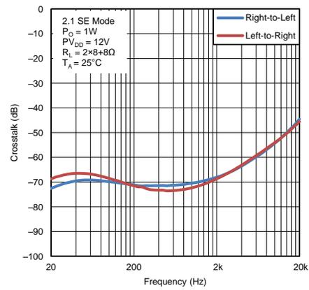
Figure 14. Crosstalk vs Frequency (2.1 SE Mode)
