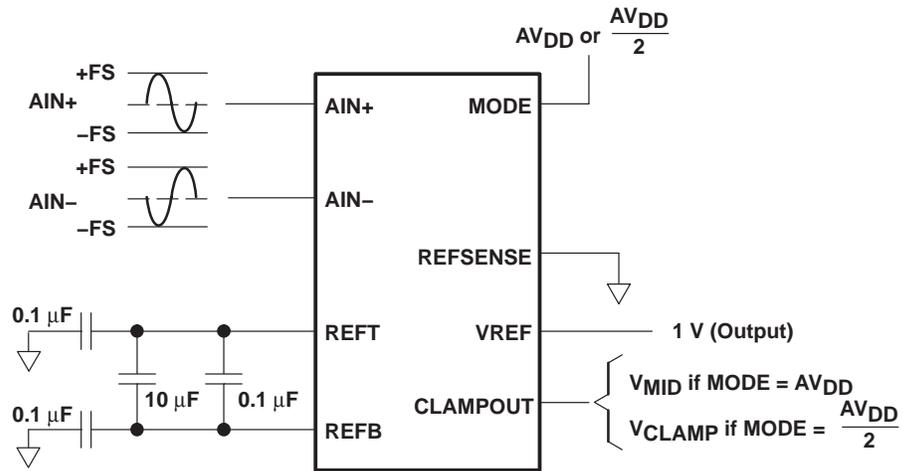
Figure 28. Internal Reference Mode, 1-V Reference Span
