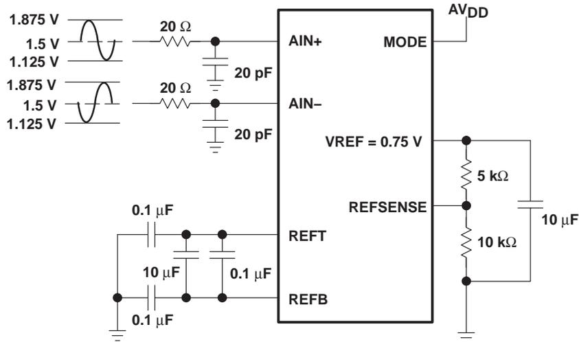
Figure 35. Operating Configuration: 1.5-V Differential Input, Internal ADC References
