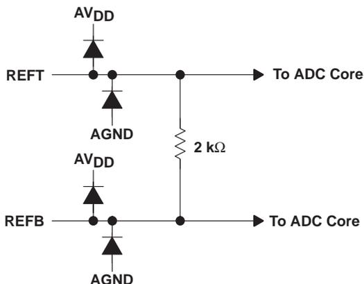
Figure 46. Equivalent Circuit of REFT and REFB Inputs
