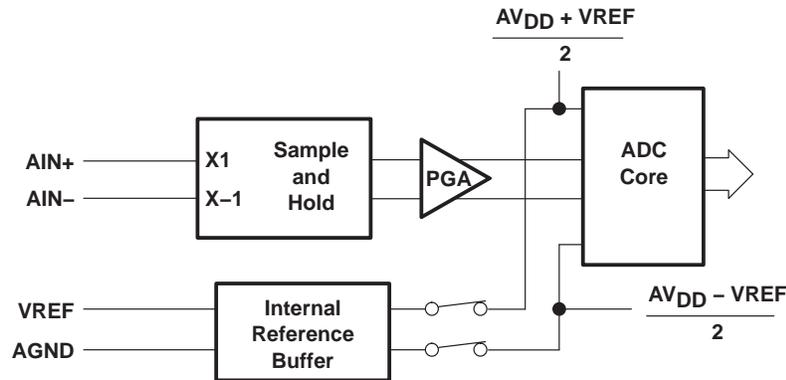
Figure 27. ADC Reference Generation, MODE = AV<sub>DD</sub>/2
