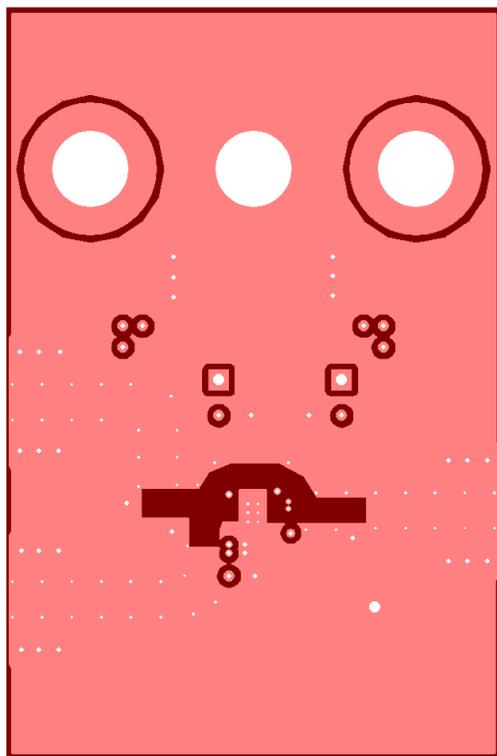
Figure 67. THS3201 EVM Board Layout (Second Layer, Ground)
