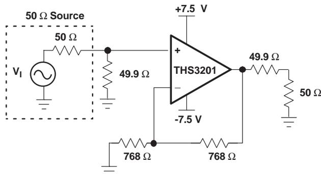
NOTE: Power supply decoupling capacitors not shown
