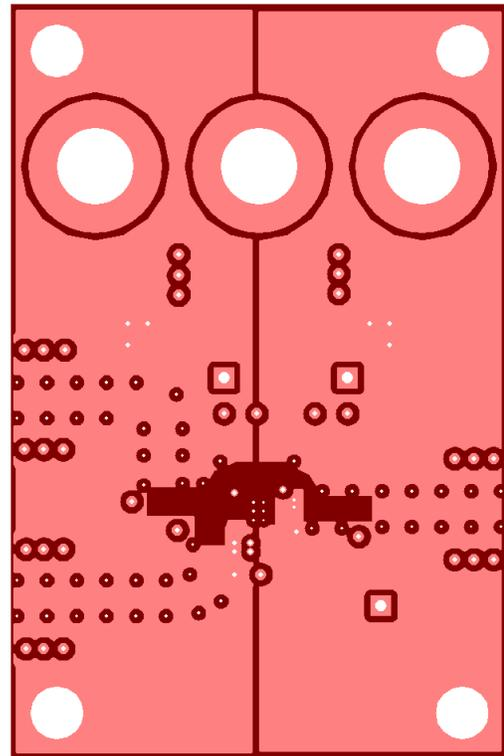
Figure 68. THS3201 EVM Board Layout (Third Layer, Power)
