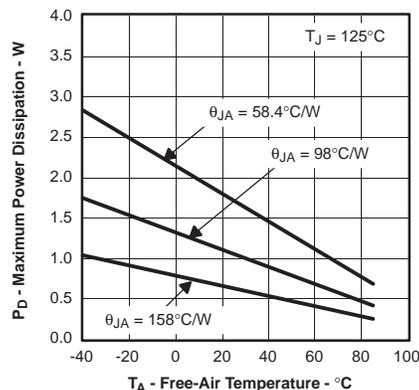
Results are With No Air Flow and PCB Size = 3"x3"
