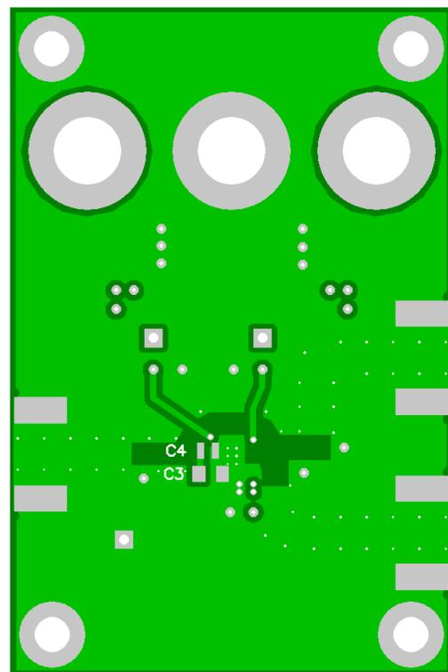
Figure 69. THS3201 EVM Board Layout (Bottom Layer)
