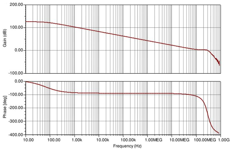
**Figure 12-2. Open-Loop Gain and Phase Simulation Result**
