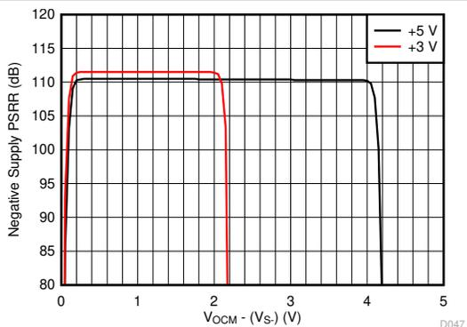
Simulated with single-ended to differential gain of 1, PSRR for negative supply to differential output
