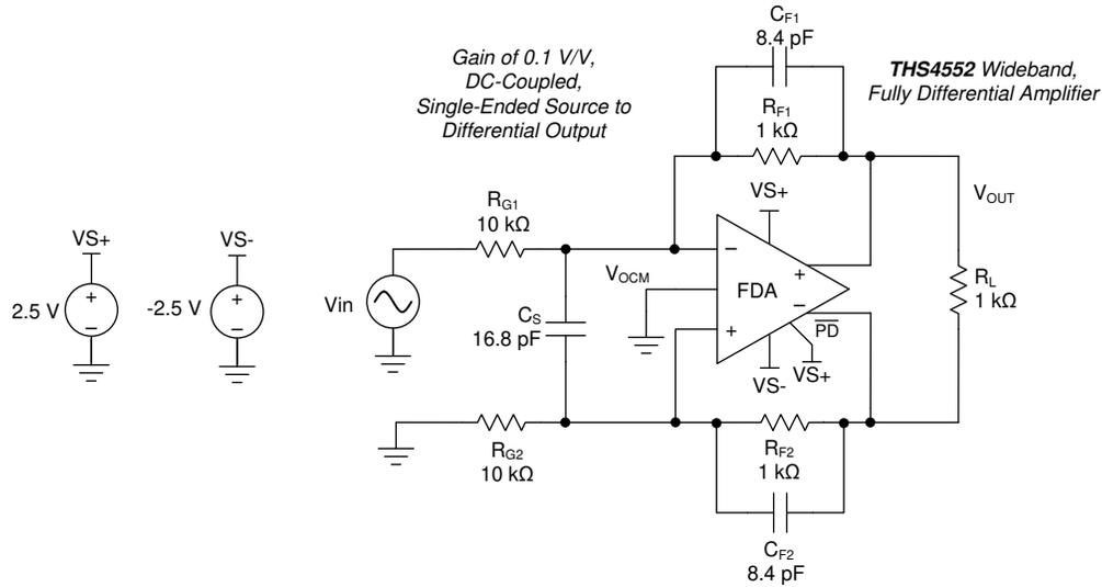
**Figure 9-8. Compensated Attenuator Circuit Using the THS4552**
