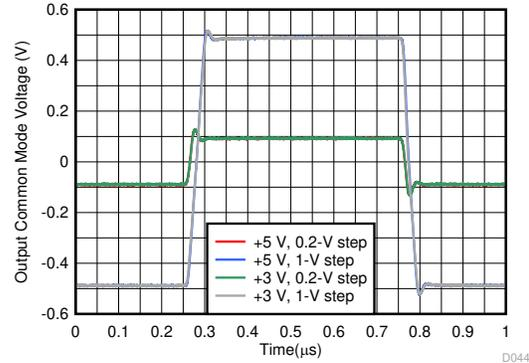
Figure 6-44. Common-Mode Voltage, Small- and Large-Step Response (VOCM Pin Driven)
