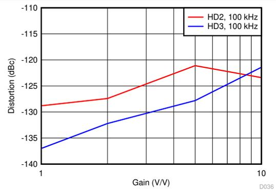
Figure 6-36. Harmonic Distortion vs Gain
