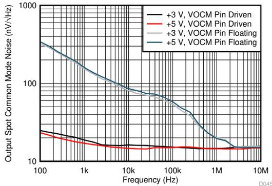
The VOCM pin is either driven to mid-supply by low-impedance source or allowed to float and default to mid-supply
