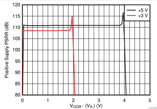
Simulated with single-ended to differential gain of 1, PSRR for positive supply to differential output
