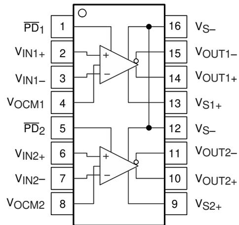
Figure 5-2. PW Package 16-Pin VSSOP Top View
