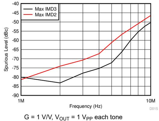
**Figure 6-15. Intermodulation Distortion (IMD2 and IMD3) vs Frequency**
