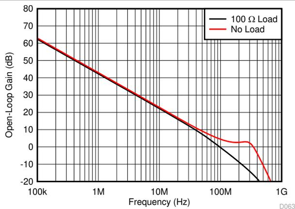
**Figure 8-1. No-Load and 100  $\Omega$  Loaded  $A_{OL}$  Gain**
