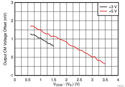
Average  $V_{\text{OCM}}$  output offset of 39 units, standard deviation  $< 2\text{ mV}$
