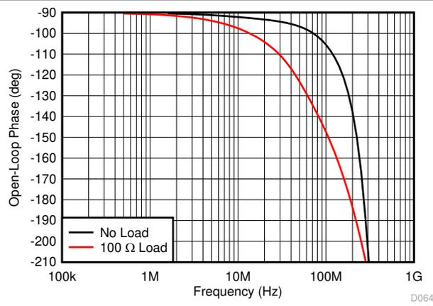
**Figure 8-2. No-Load and 100  $\Omega$   $A_{OL}$  Phase**
