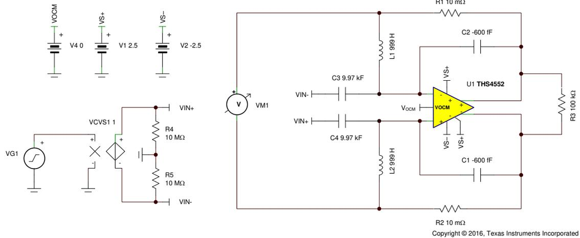
**Figure 12-1. Open-Loop Gain and Phase TINA-TI™ Simulation Setup**
