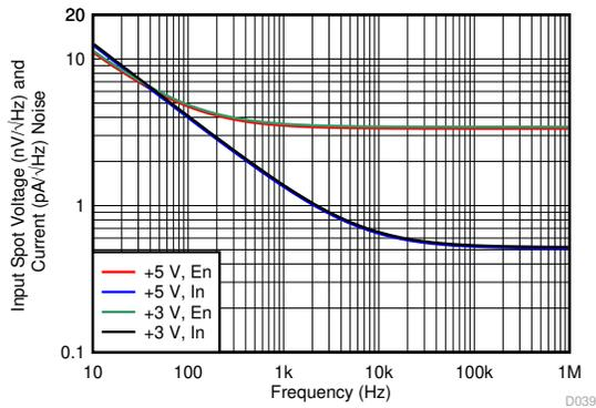
**Figure 6-39. Input Spot Noise vs Frequency**
