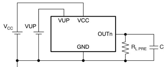
Figure 8. Delay Time Test Circuit for Pre-Charge FET
