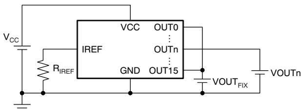
Figure 9. Constant Current Test Circuit for OUTn
