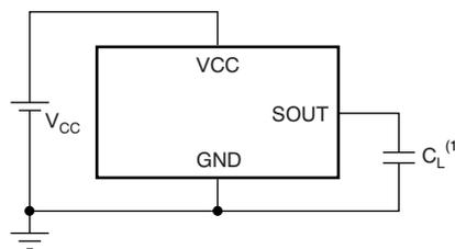
(1)  $C_L$  includes measurement probe and jig capacitance.
