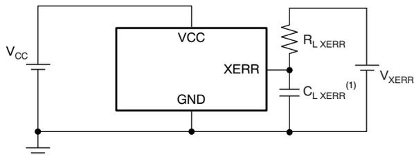
(1)  $C_{L\_XERR}$  includes measurement probe and jig capacitance.
