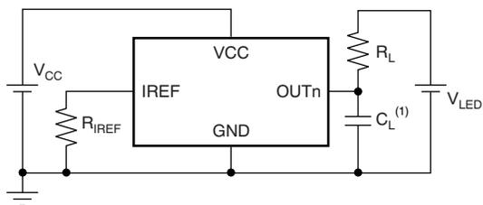
(1)  $C_L$  includes measurement probe and jig capacitance.
