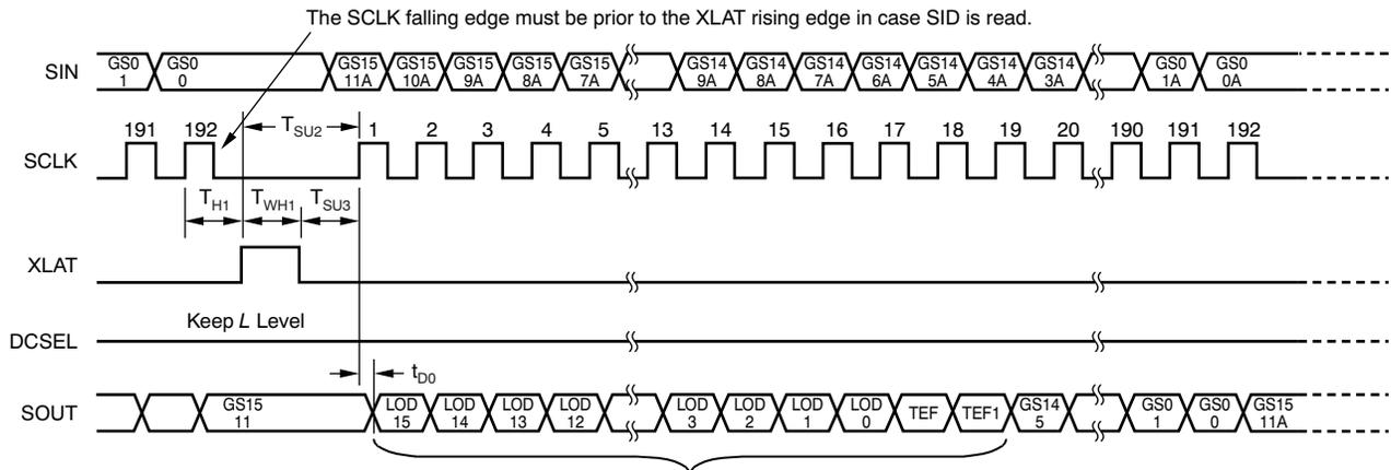
SID are entered in GS shift register at the first rising edge of SCLK with low level of DCSEL after XLAT. The SID readout consists of the saved LOD result at the 33rd GSCLK rising edge in the previous display period and the saved TEF data and TEF1 at the rising edge of the first of SCLK after XLAT goes low.
