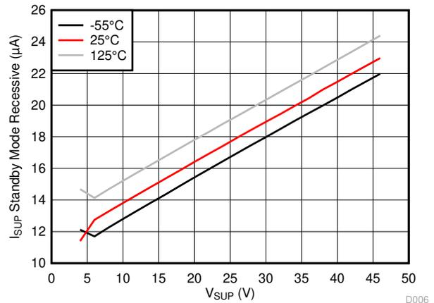
Figure 6-6. Standby Mode Recessive vs V<sub>SUP</sub>
