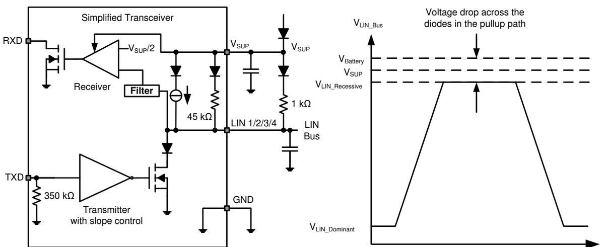
**Figure 7-1. Commander Node Configuration with Voltage Levels**
