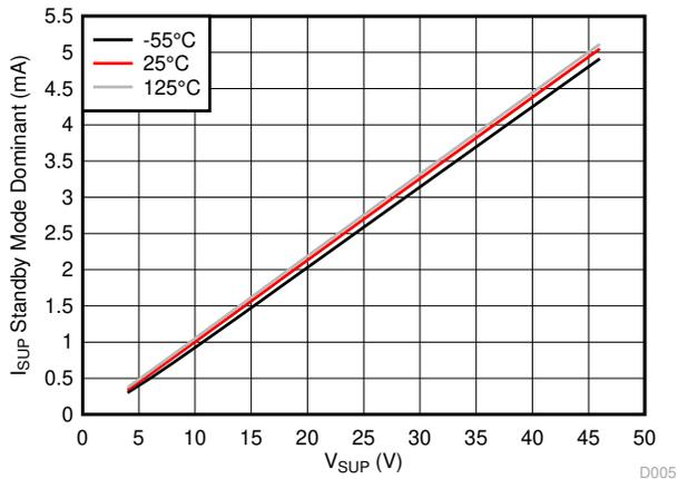
Figure 6-5. Standby Mode Dominant vs V<sub>SUP</sub>
