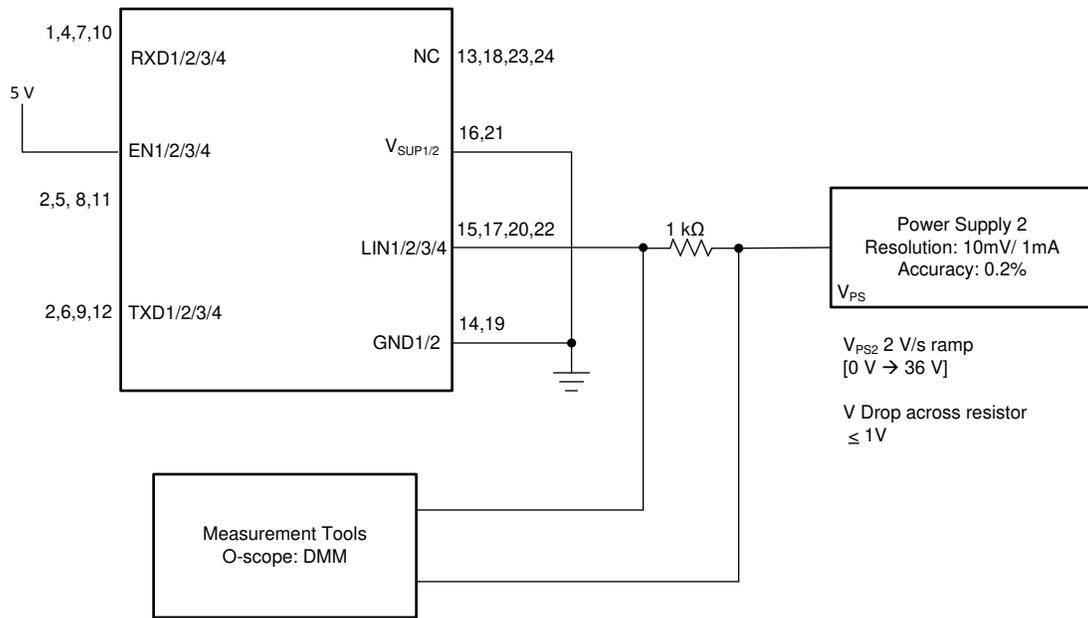
**Figure 7-10. Test Circuit for I<sub>BUS\_NO\_BAT</sub> Loss of Battery**
