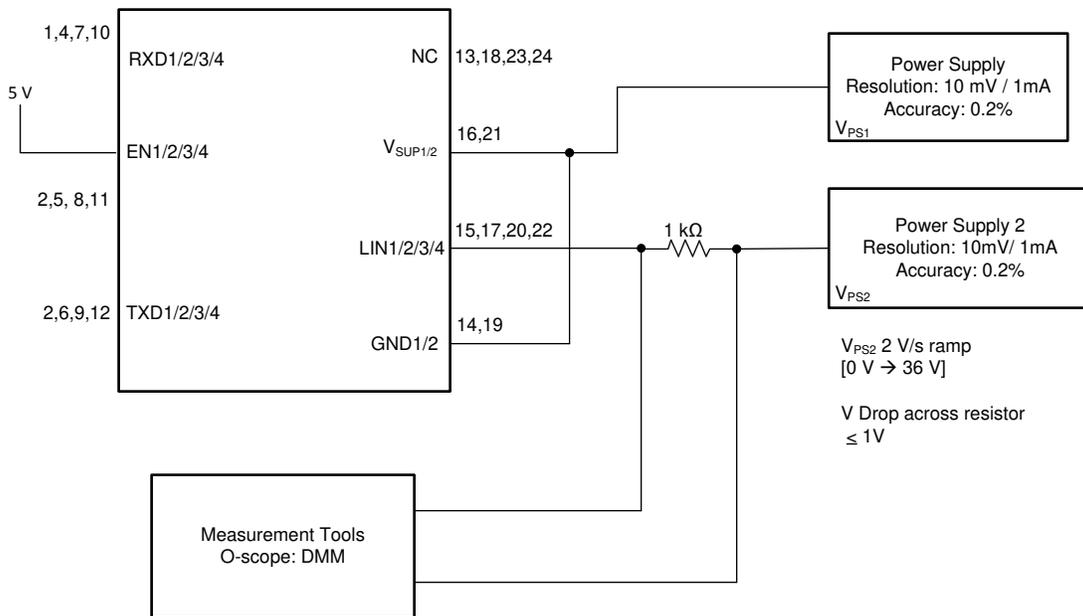
**Figure 7-9. Test Circuit for  $I_{BUS\_NO\_GND}$  Loss of GND**
