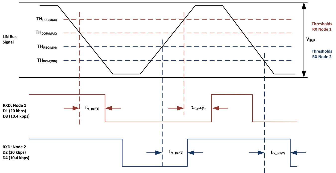
Figure 7-14. Propagation Delay
