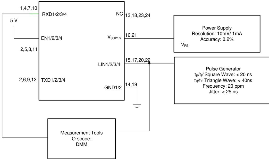
**Figure 7-4. LIN Receiver Test with RX Access**
