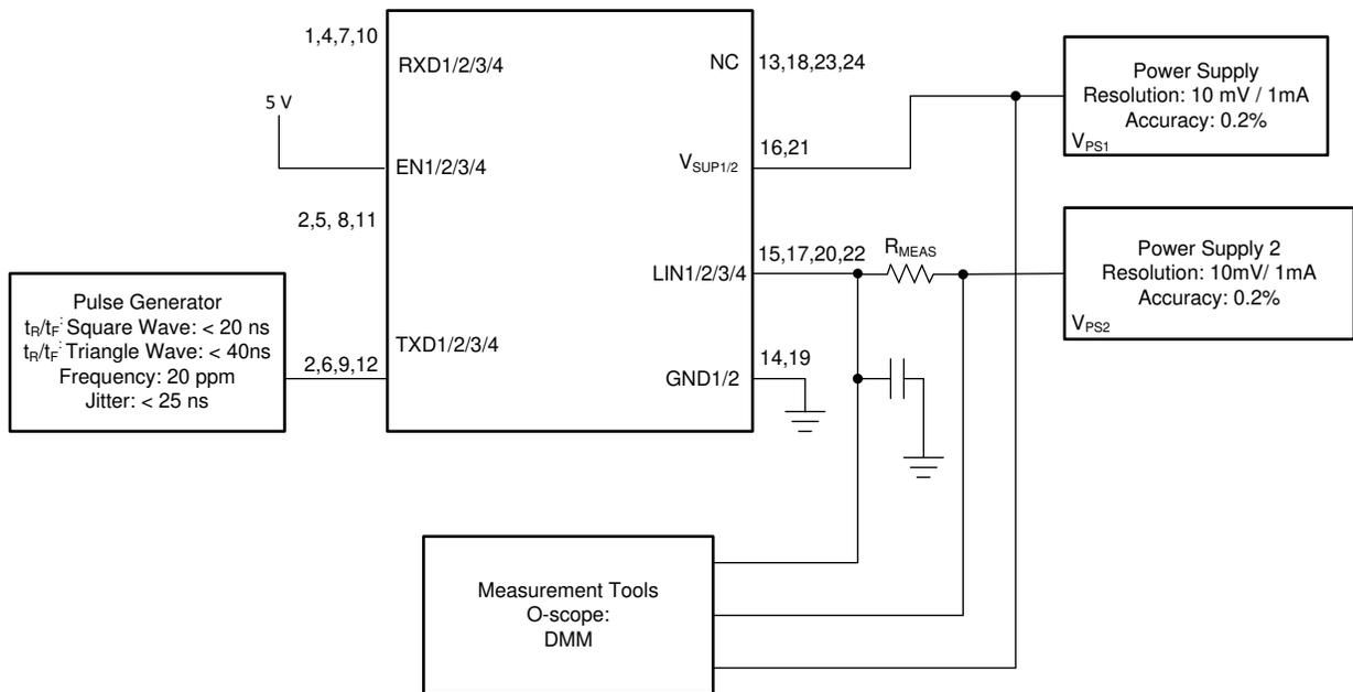
**Figure 7-11. Test Circuit Slope Control and Duty Cycle**
