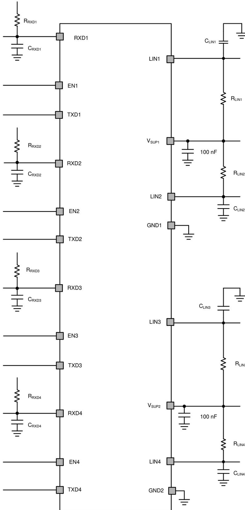
**Figure 7-18. Test Circuit for AC Characteristics**
