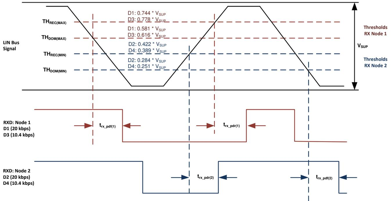
**Figure 8-13. Propagation Delay**
