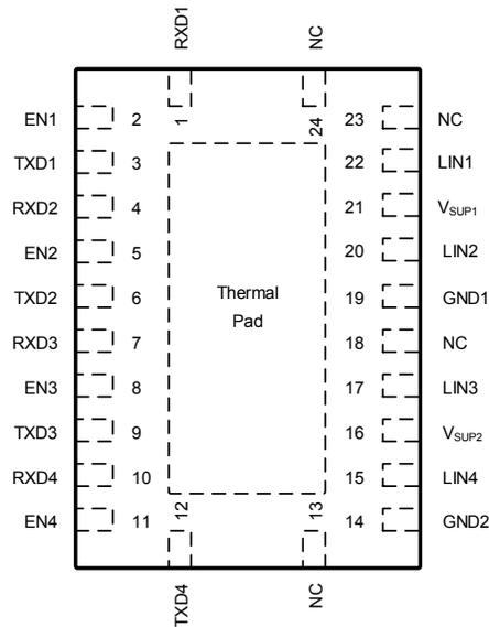
**Figure 6-1. RGY Package, 24-Pin RGY (VQFN), Top View**
