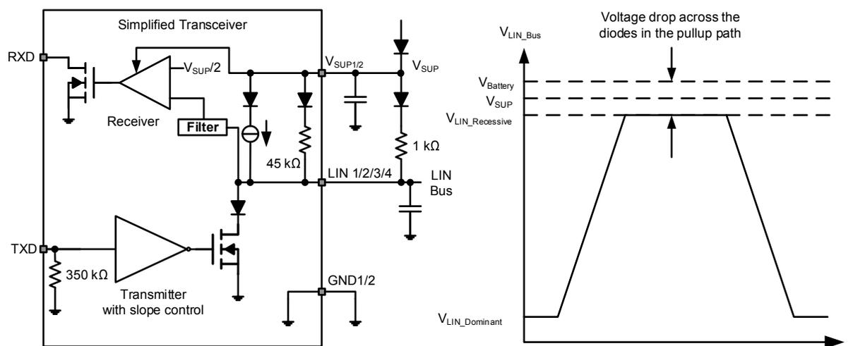
**Figure 9-1. Commander Node Configuration with Voltage Levels**
