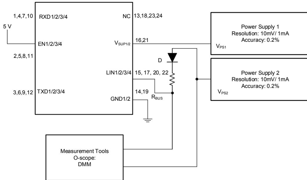
**Figure 8-5.  $V_{SUP\_NON\_OP}$**
