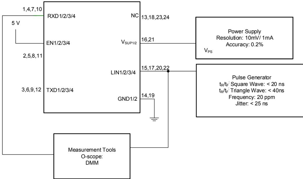
**Figure 8-4. LIN Receiver Test with RX Access**
