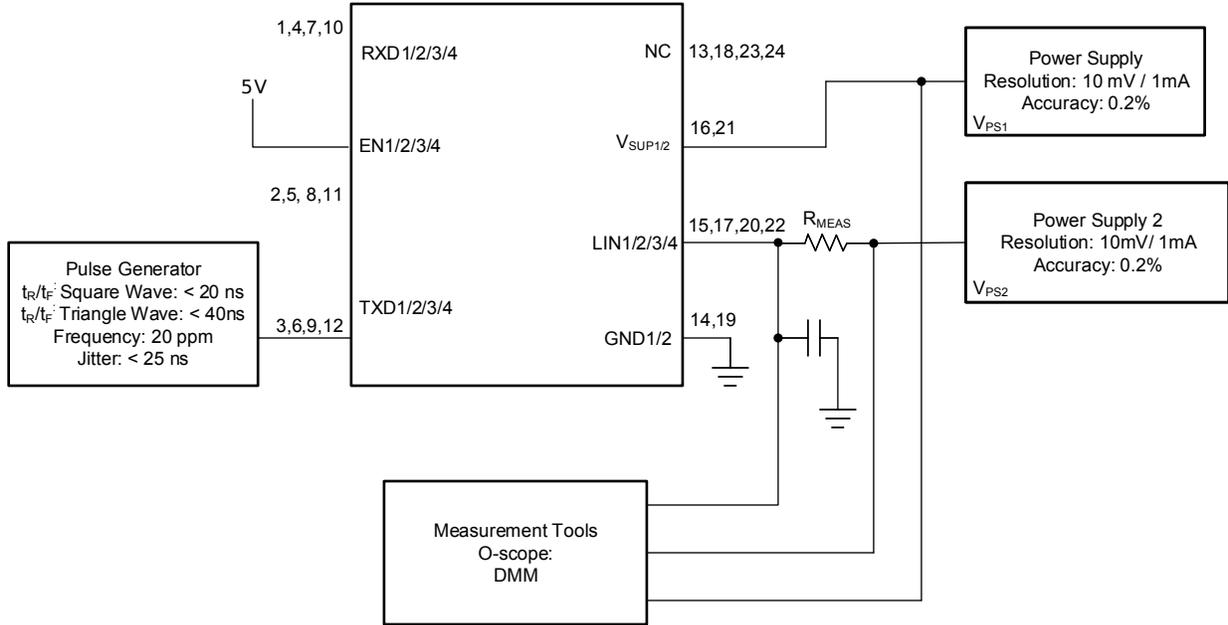
Figure 8-10. Test Circuit Slope Control and Duty Cycle
