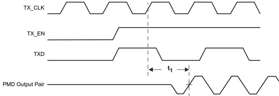
**Figure 9-13. 10Base-T Transmit Timing (Start of Packet)**
