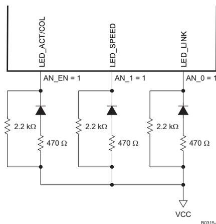
**Figure 3-6. AN Pin Configuration and LED Loading Example**
