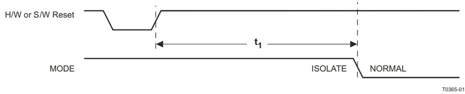
Figure 9-25. Isolation Timing
