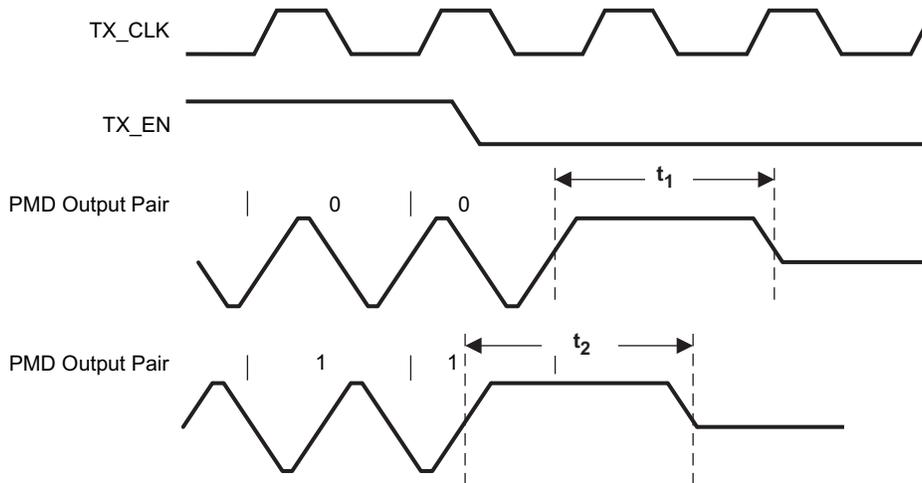
**Figure 9-14. 10Base-T Transmit Timing (End of Packet)**
