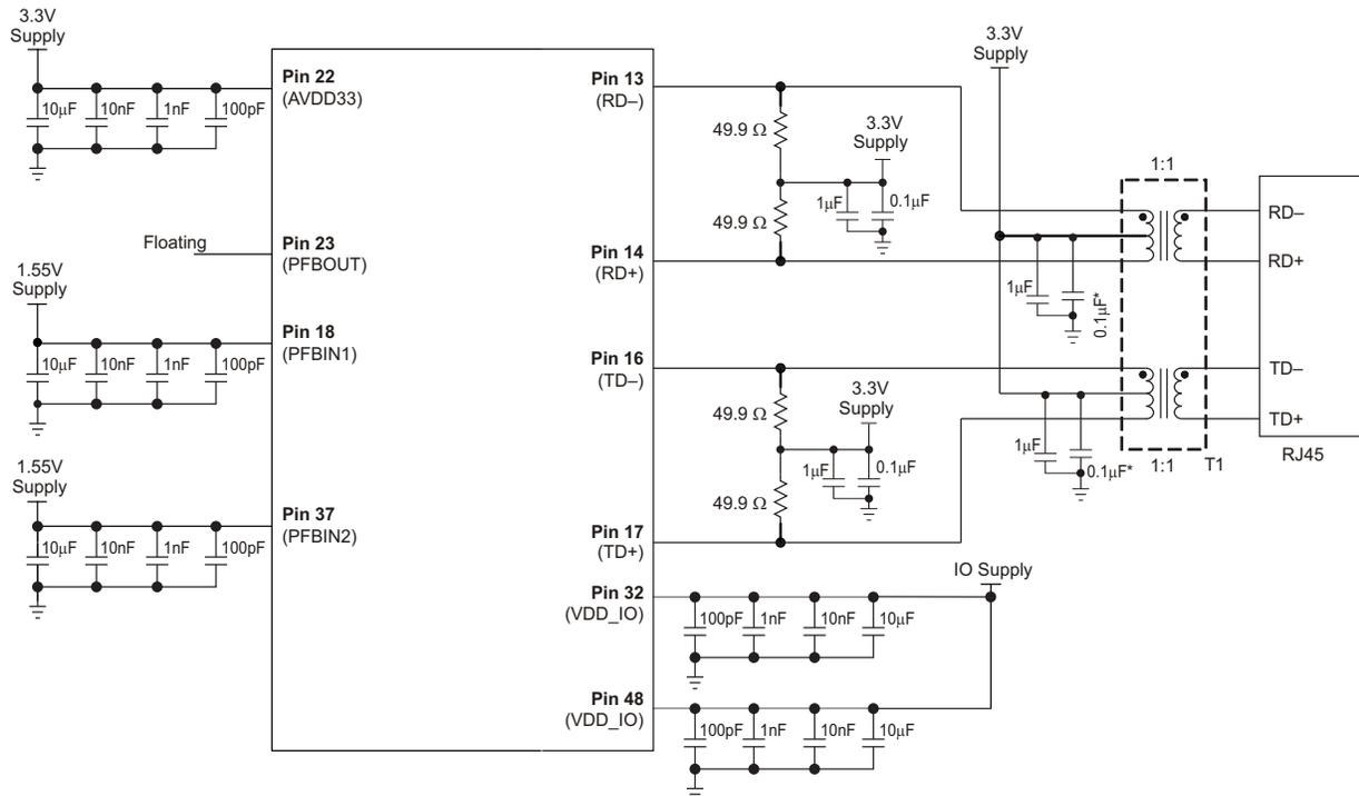
**Figure 3-2. Power Connections for Dual Supply Operation**
