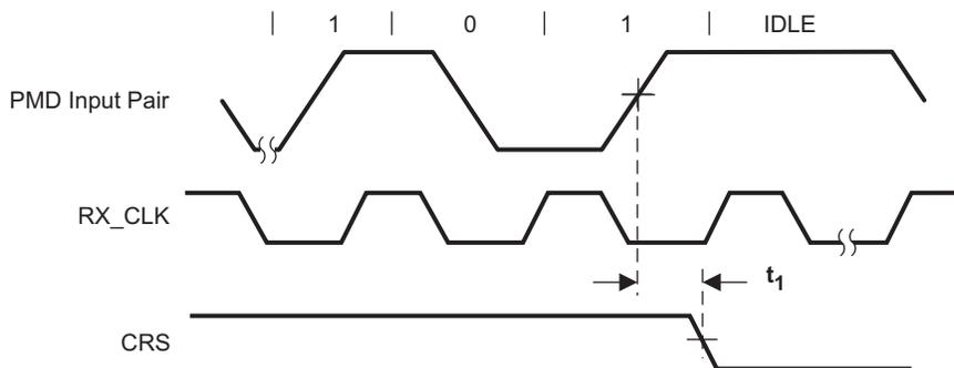
Figure 9-16. 10Base-T Receive Timing (End of Packet)
