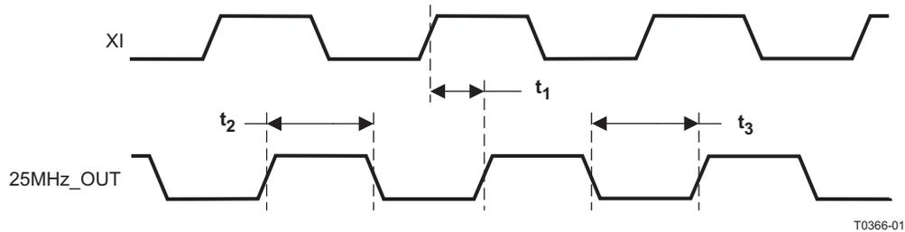
Figure 9-26. 25MHz\_OUT Timing
