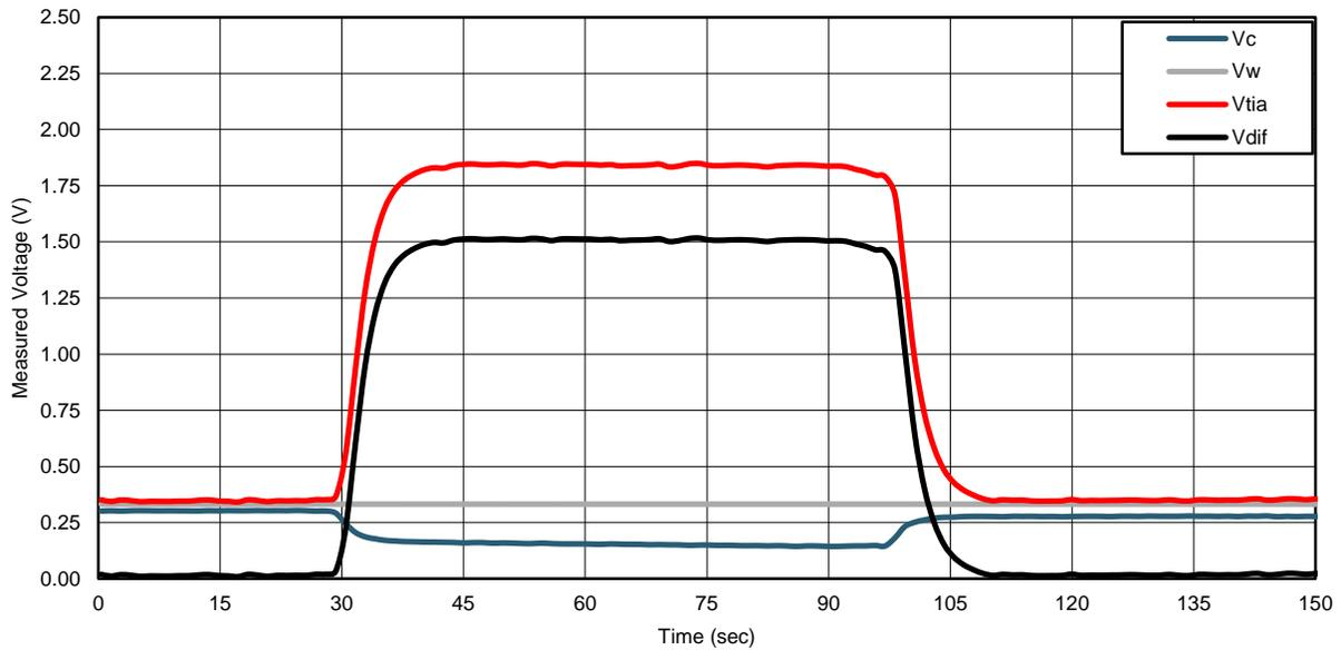
**Figure 39. Monitored Voltages when Exposed to 200ppm CO**
