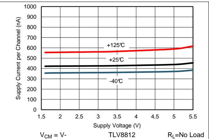
Figure 2. Supply Current vs. Supply Voltage, TLV8812
