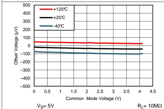
Figure 5. Typical Offset Voltage vs. Common Mode Voltage
