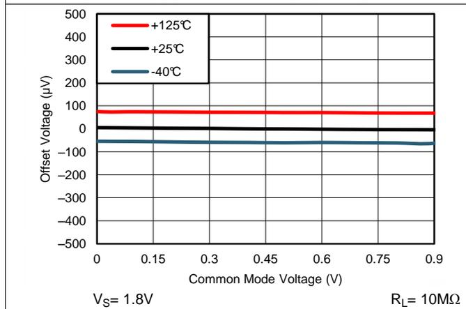
Figure 3. Typical Offset Voltage vs. Common Mode Voltage
