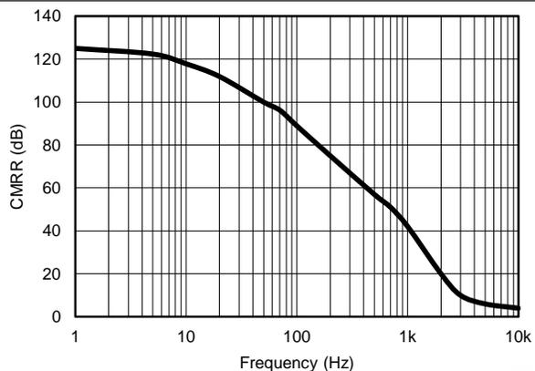
$T_A = 25$        $R_L = 10\text{M}\Omega$        $\Delta V_{CM} = 0.5\text{Vpp}$
