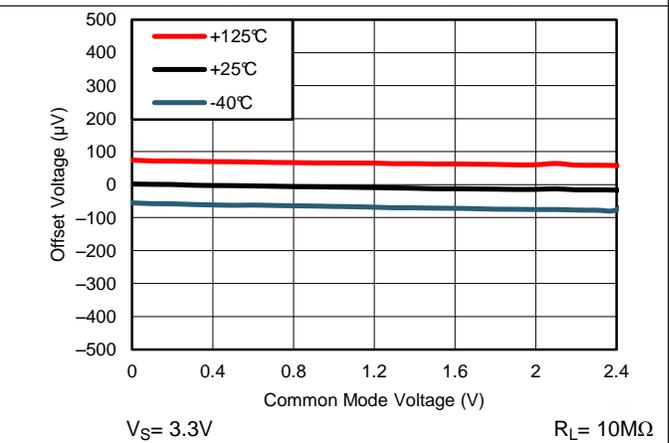
Figure 4. Typical Offset Voltage vs. Common Mode Voltage
