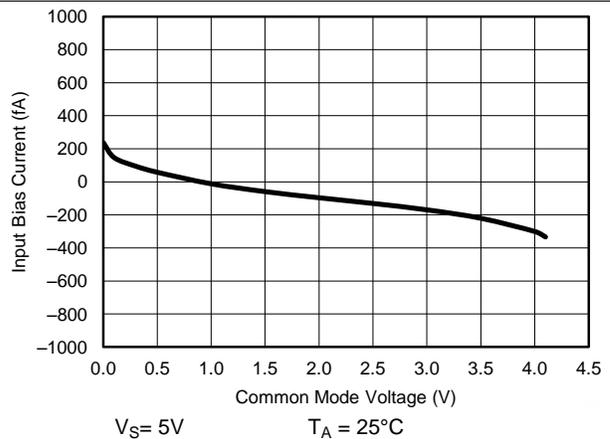
**Figure 10. Input Bias Current vs. Common Mode Voltage**
