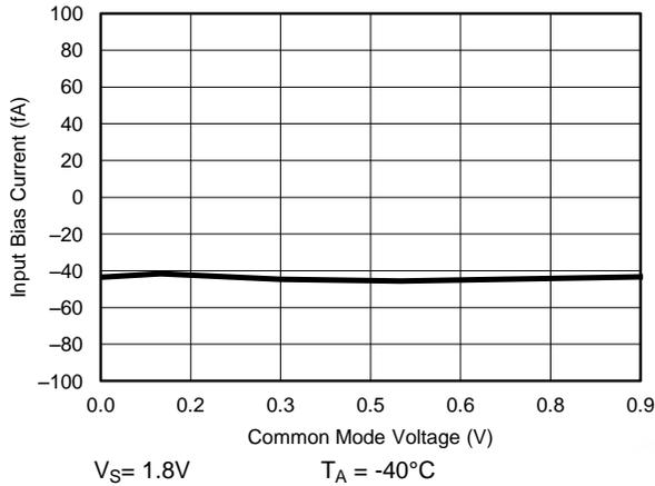
**Figure 7. Input Bias Current vs. Common Mode Voltage**
