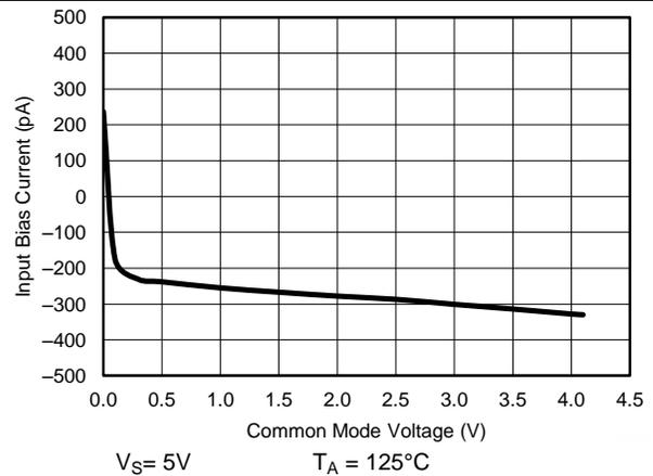
**Figure 12. Input Bias Current vs. Common Mode Voltage**
