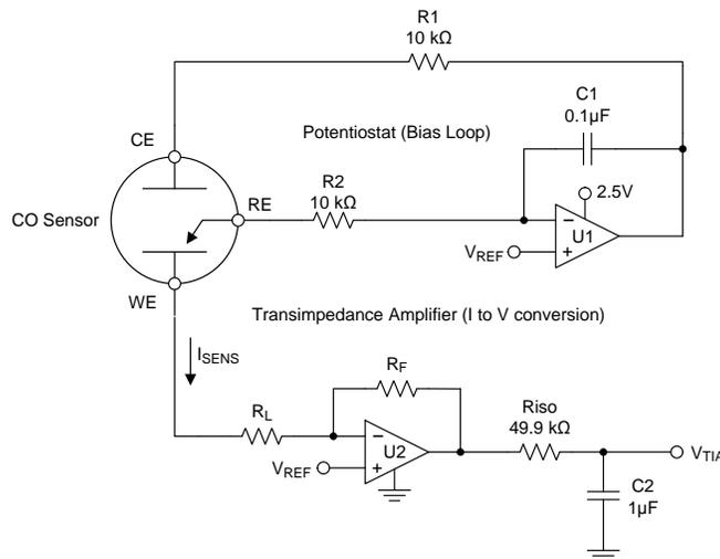
Figure 38. Three Terminal Gas Sensor Amplifier Schematic
