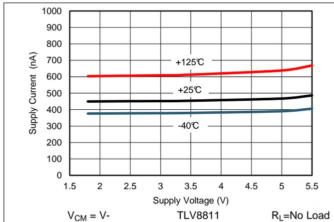
Figure 1. Supply Current vs. Supply Voltage, TLV8811
