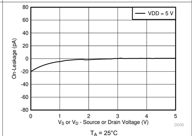
Figure 6-6. On-Leakage vs Source or Drain Voltage
