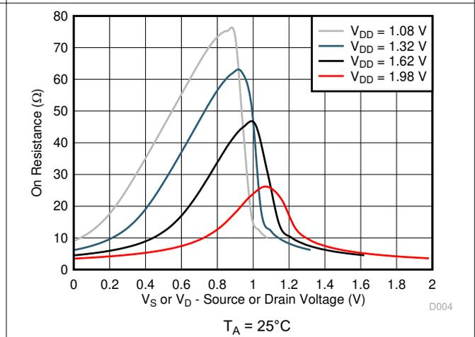
Figure 6-4. On-Resistance vs Source or Drain Voltage
