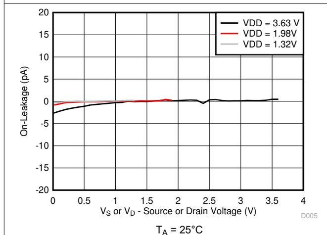
Figure 6-5. On-Leakage vs Source or Drain Voltage
