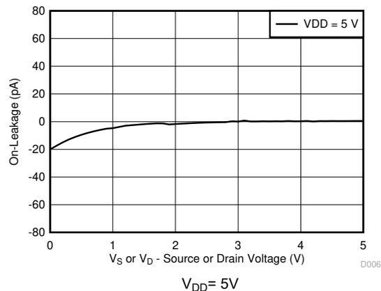
Figure 9-4. On-Leakage vs Source or Drain Voltage
