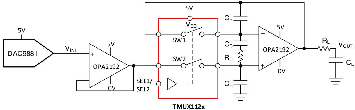
**Figure 9-2. 2-Channel Sample-and-Hold Circuit with Pedestal Error Compensation**
