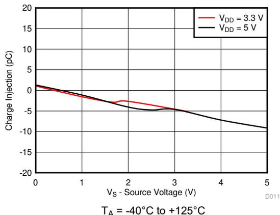
Figure 9-3. Charge Injection vs Source Voltage
