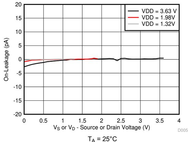
**Figure 9-6. On-Leakage vs Source or Drain Voltage**
