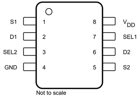
**Figure 5-1. DGK Package, 8-Pin VSSOP (Top View)**
