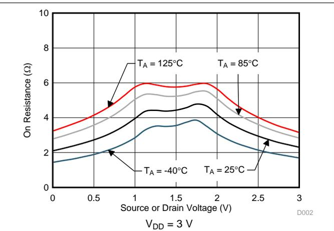
Figure 2. On-Resistance vs Source or Drain Voltage
