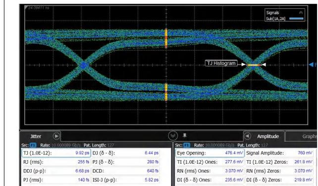
Figure 5-3. Eye Diagram at 10Gbps Through Baseline Setup (Cal-Trace, no DUT)
