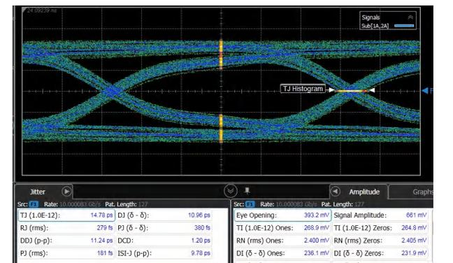
Figure 5-4. Eye Diagram at 10Gbps Through TMUXHS4446 (Cal-Trace + DUT)
