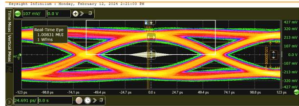
**Figure 7-8. 8.1Gbps DP Compliance Eye Diagram - with TMUXHS4446**
