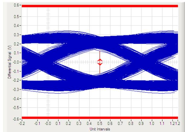
**Figure 7-12. 10Gbps USB Compliance Eye Diagram - with TMUXHS4446**
