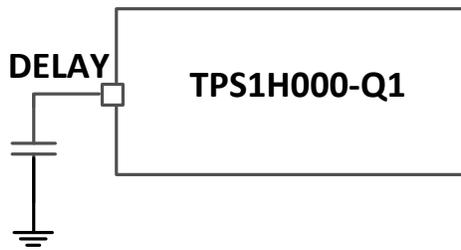
Figure 6-4. Latch-Off-Mode Connection
