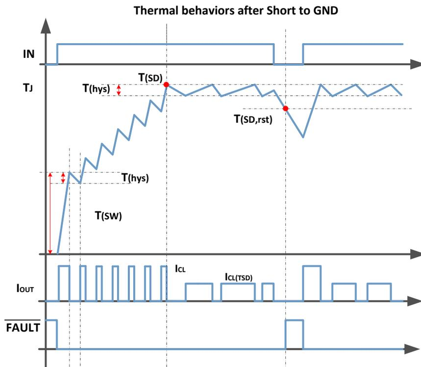
**Figure 6-11. Thermal Behavior Diagram**
