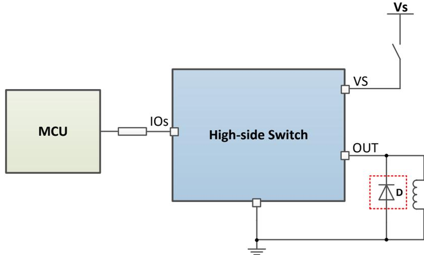
**Figure 6-16. Protection for Loss of Power Supply**
