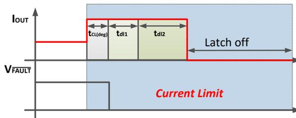
Figure 6-5. Latch-Off-Mode Example
