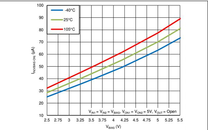
Figure 2. Quiescent Current vs.  $V_{BIAS}$  (Single Channel)
