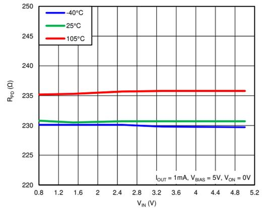
Figure 10. R<sub>PD</sub> vs. V<sub>IN</sub> (V<sub>BIAS</sub> = 5 V, Single Channel)
