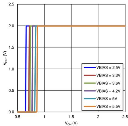
Figure 11. V<sub>OUT</sub> vs. V<sub>ON</sub> (T<sub>A</sub> = 25°C, Single Channel)
