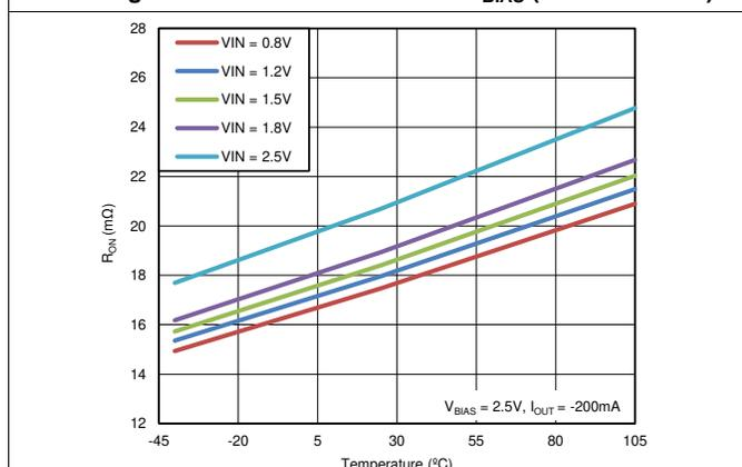
Figure 5.  $R_{ON}$  vs. Temperature ( $V_{BIAS} = 2.5$  V, Single Channel)
