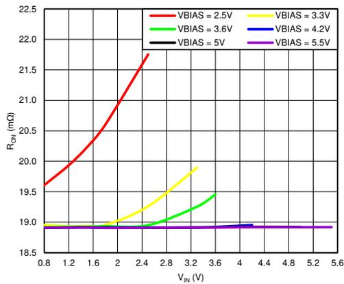
Figure 9. R<sub>ON</sub> vs. V<sub>IN</sub> (T<sub>A</sub> = 25°C, Single Channel)
