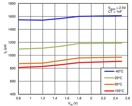
Figure 12. t<sub>D</sub> vs. V<sub>IN</sub> (V<sub>BIAS</sub> = 2.5 V, CT = 1 nF)
