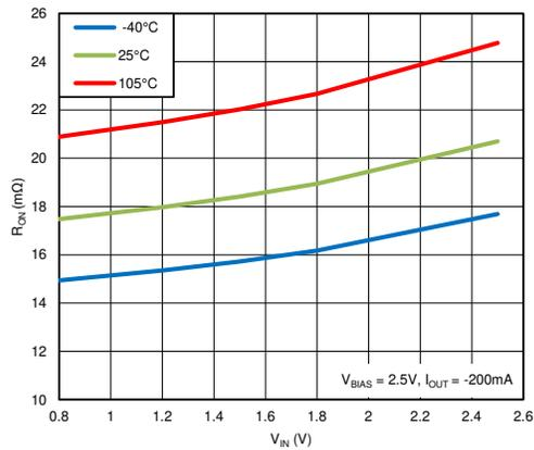
Figure 7. R<sub>ON</sub> vs. V<sub>IN</sub> (V<sub>BIAS</sub> = 2.5 V, Single Channel)
