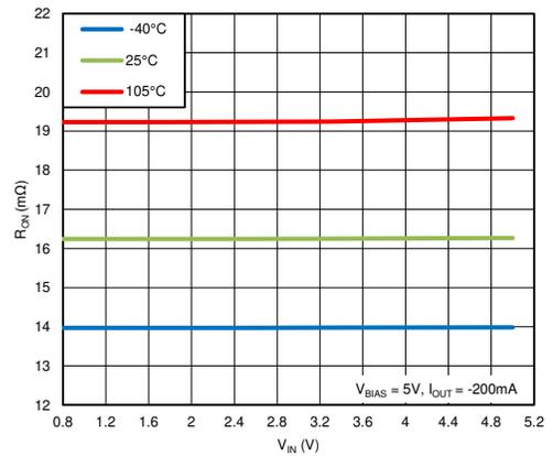
Figure 8. R<sub>ON</sub> vs. V<sub>IN</sub> (V<sub>BIAS</sub> = 5 V, Single Channel)
