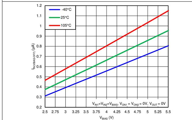
Figure 3. Shutdown Current vs.  $V_{BIAS}$  (Both Channels)
