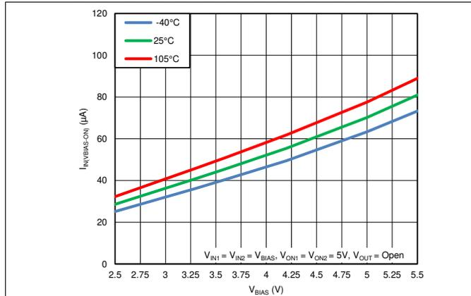
Figure 1. Quiescent Current vs.  $V_{BIAS}$  (Both Channels)
