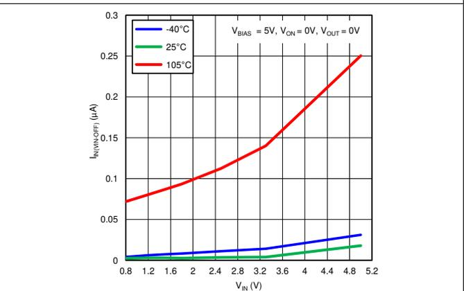
Figure 4. Off-State  $V_{IN}$  Current vs.  $V_{IN}$  (Single Channel)
