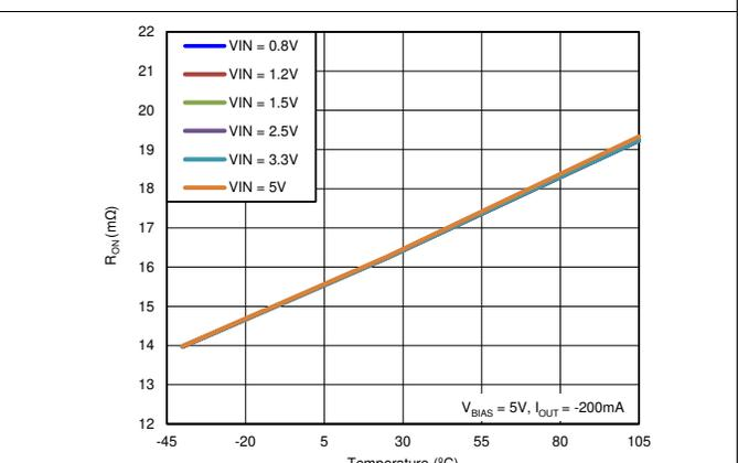
Figure 6.  $R_{ON}$  vs. Temperature ( $V_{BIAS} = 5$  V, Single Channel)
