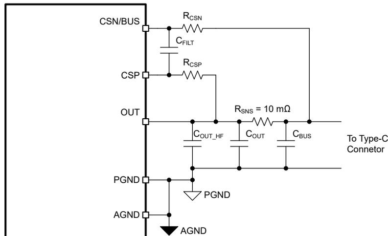
**Figure 9-5. Current Sense Amplifier: RC Filter Components**
