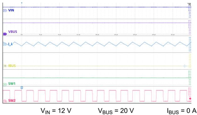
**Figure 9-18. Boost Mode: Nominal  $V_{IN}$ , No Load**
