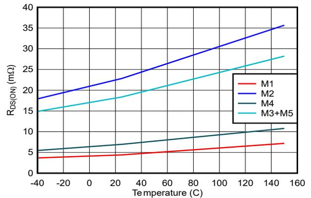
Figure 6-16. Buck-Boost Power FET  $R_{DS(ON)}$  vs Temperature
