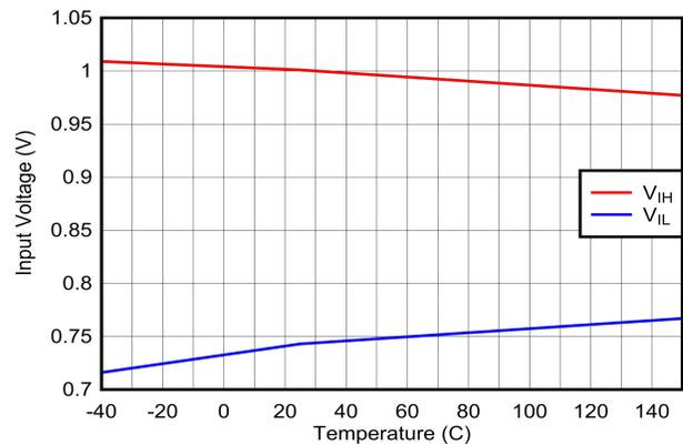
Figure 6-48. GPIO: Input Voltage Thresholds vs Temperature
