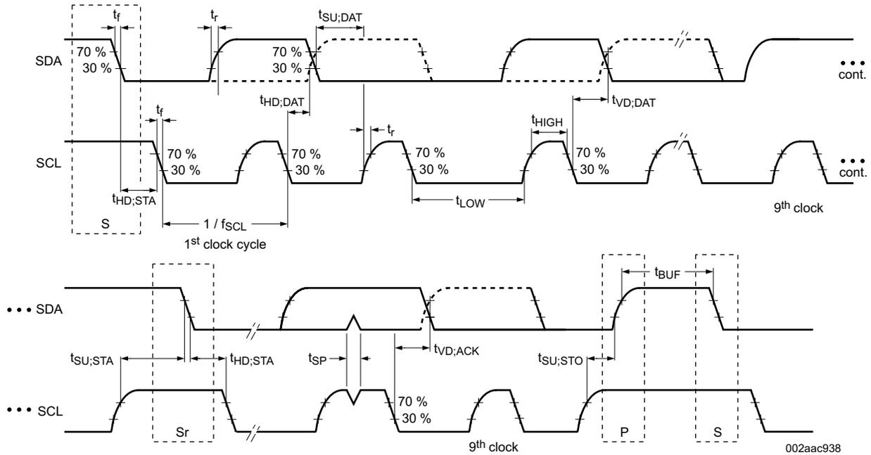
Figure 7-1. I<sup>2</sup>C Target Interface Timing
