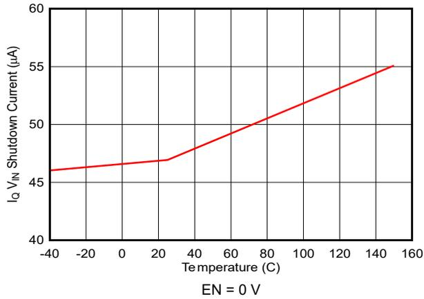
Figure 6-1.  $I_{Q\ V_{IN}}$  Shutdown Current vs Temperature
