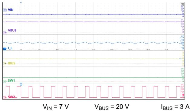
**Figure 9-16. Boost Mode: Low  $V_{IN}$ , 3 A Load**
