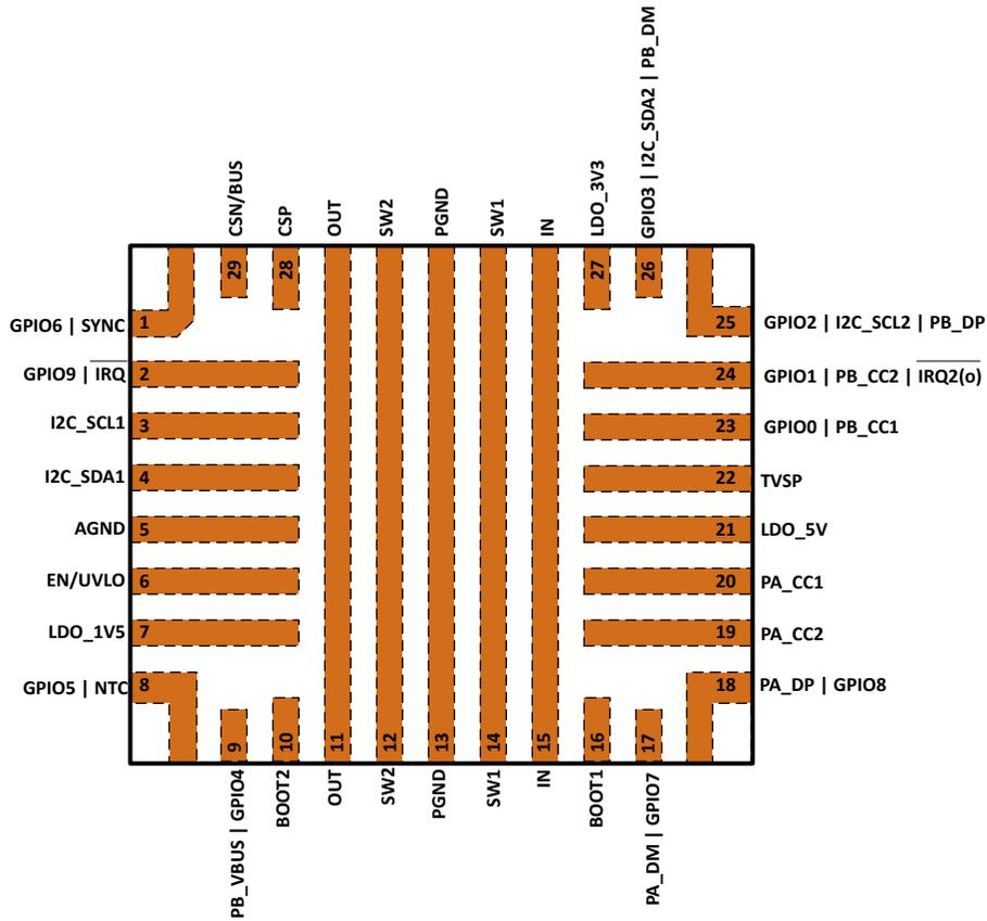
Figure 5-1. RQL Package 29-Pin (VQFN) Top View
