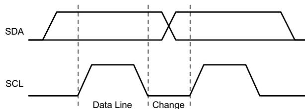
**Figure 8-36. I<sup>2</sup>C Bit Transfer**
