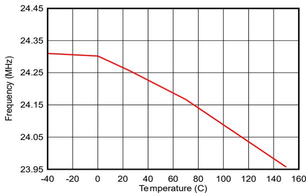
Figure 6-35. (M0) 24 MHz Oscillator vs Temperature
