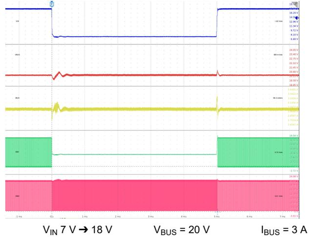
Figure 9-35. Line Transient:  $V_{BUS} = 20\text{ V}$
