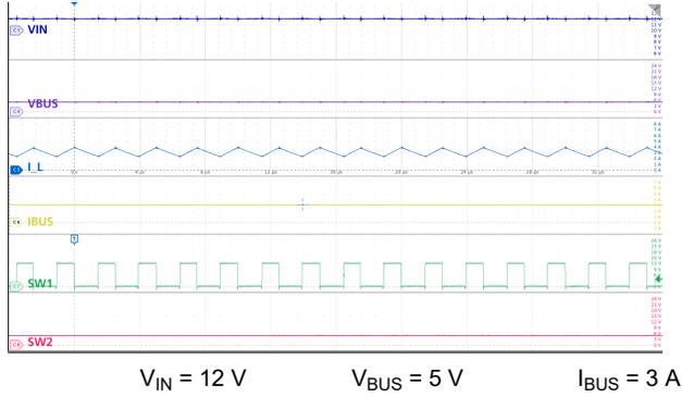
**Figure 9-20. Buck Mode: nominal  $V_{IN}$ , 3 A Load**
