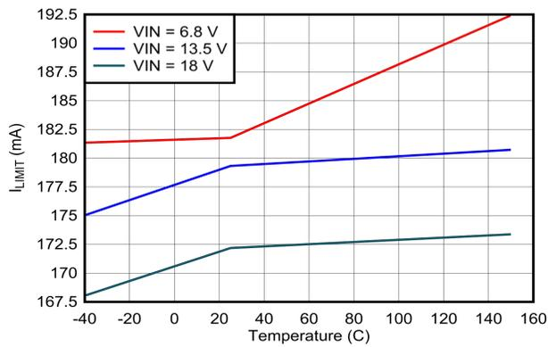
Figure 6-9. LDO\_5V Current Limit vs  $V_{IN}$  and Temperature
