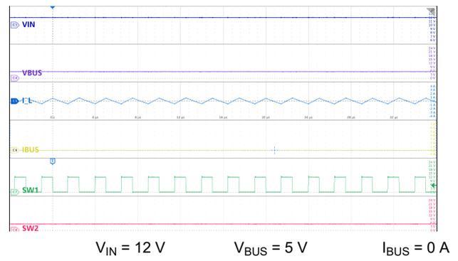
**Figure 9-19. Buck Mode: Nominal  $V_{IN}$ , No Load**
