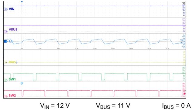
**Figure 9-23. Buck-Boost Mode:  $V_{IN} \neq V_{BUS}$ , No Load**
