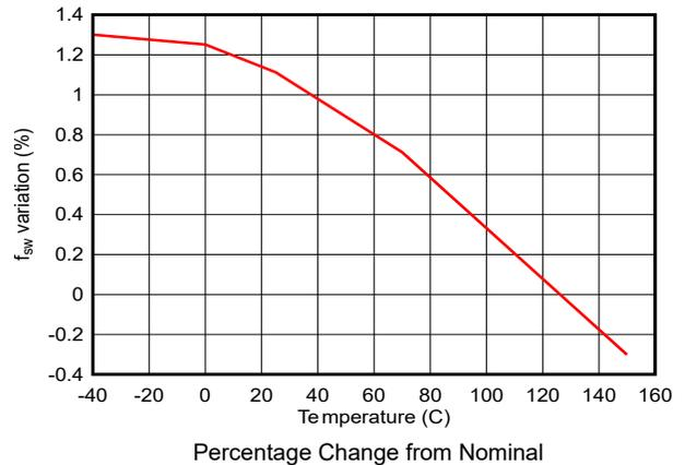
Figure 6-24. Buck-Boost Switching Frequency Variation vs Temperature
