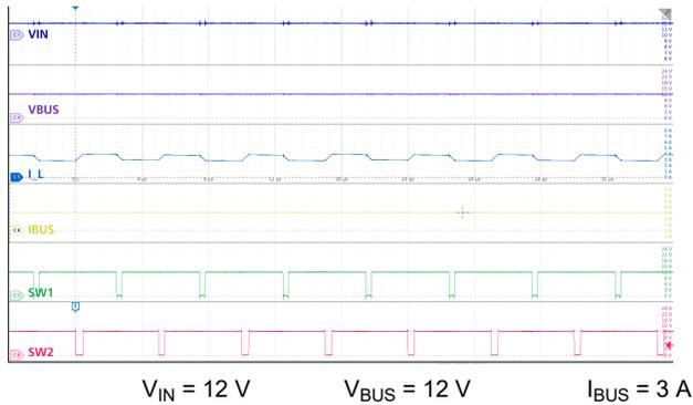
**Figure 9-24. Buck-Boost Mode:  $V_{IN} = V_{BUS}$ , 3 A Load**
