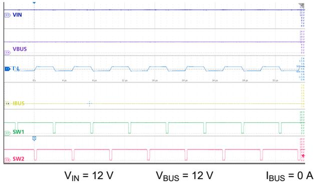
**Figure 9-22. Buck-Boost Mode:  $V_{IN} = V_{BUS}$ , No Load**
