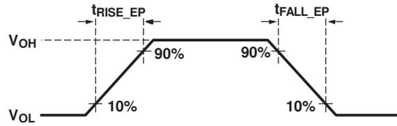
**Figure 7-3. USB Endpoint Transmitter Rise and Fall Time**
