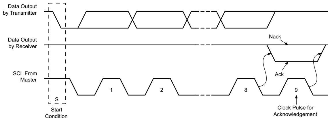
**Figure 8-37. I<sup>2</sup>C Acknowledgment**
