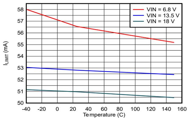
Figure 6-11. LDO\_3V3 Current Limit vs  $V_{IN}$  and Temperature
