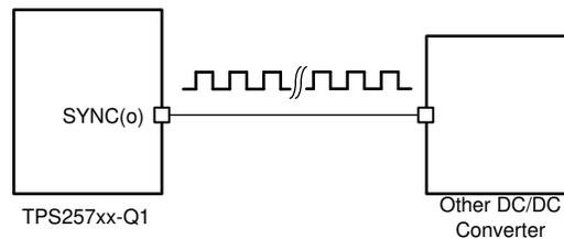
**Figure 8-15. Using SYNC(o) to drive external DC/DC Converter**
