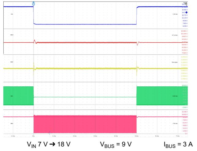
Figure 9-37. Line Transient:  $V_{BUS} = 9\text{ V}$
