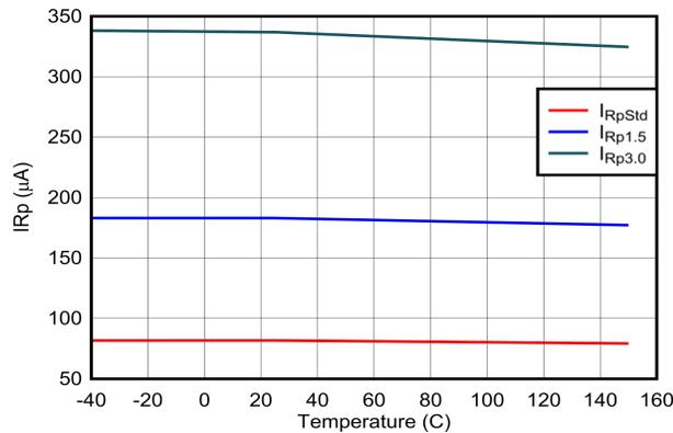
Figure 6-37. Type-C Cable Detect:  $I_{Rp}$  vs Temperature
