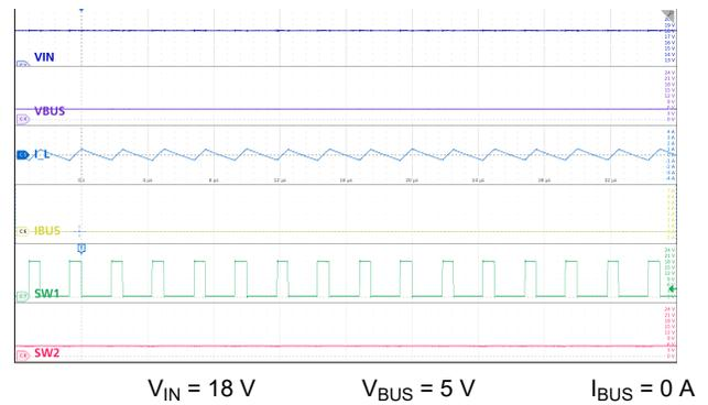
**Figure 9-15. Buck Mode: High  $V_{IN}$ , No Load**
