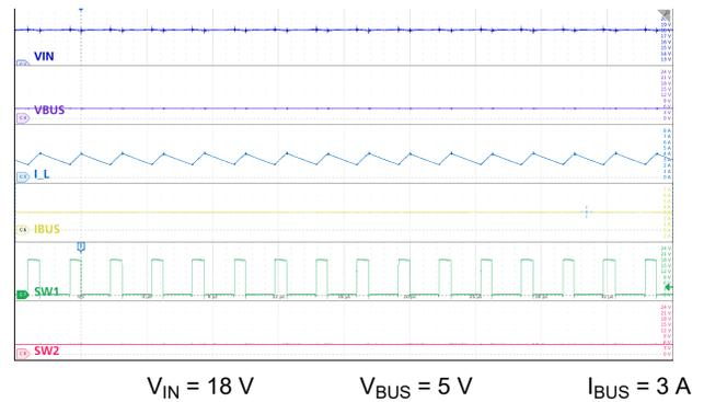
**Figure 9-17. Buck Mode: High  $V_{IN}$ , 3 A load**
