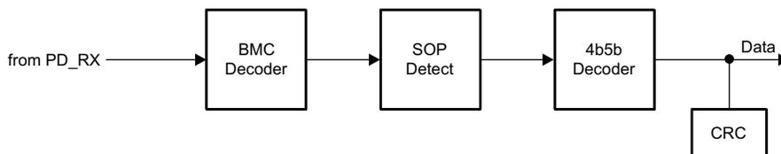
**Figure 8-20. USB-PD Baseband Receiver Block Diagram**
