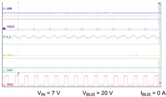
**Figure 9-14. Boost Mode: Low  $V_{IN}$ , No Load**
