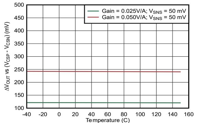
Figure 6-30. Cable Voltage Droop Compensation vs Temperature
