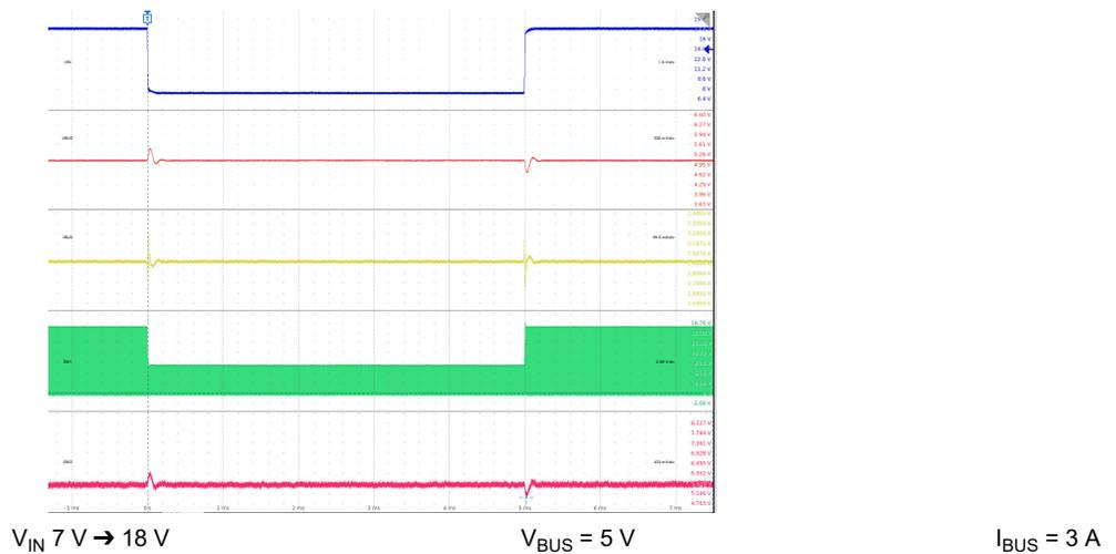
Figure 9-38. Line Transient:  $V_{BUS} = 5\text{ V}$
