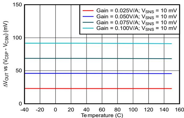
Figure 6-29. Cable Voltage Droop Compensation vs Temperature
