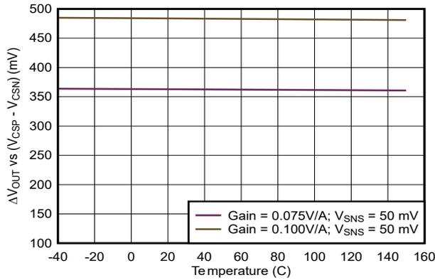
Figure 6-31. Cable Voltage Droop Compensation vs Temperature
