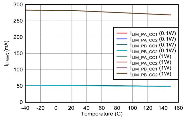
Figure 6-40.  $V_{CONN}$  Power Path: Current Limit vs Temperature
