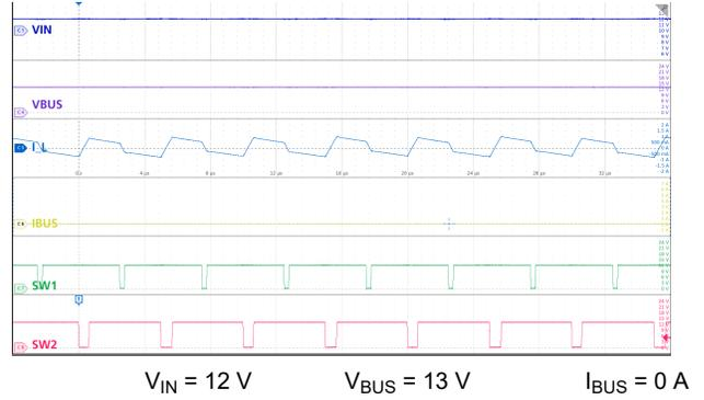
**Figure 9-21. Buck-Boost Mode:  $V_{IN} \neq V_{BUS}$ , No Load**
