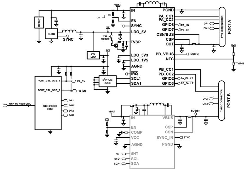
Figure 9-2. Simplified Dual USB PD with HUB
