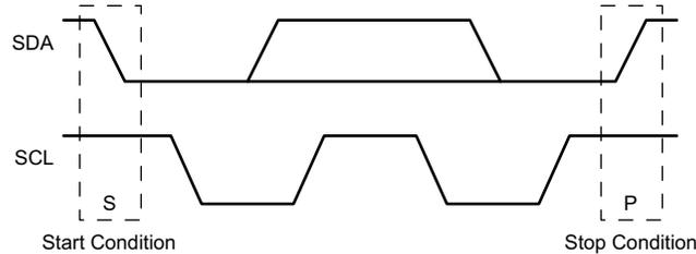
**Figure 8-35. I<sup>2</sup>C Definition of Start and Stop Conditions**
