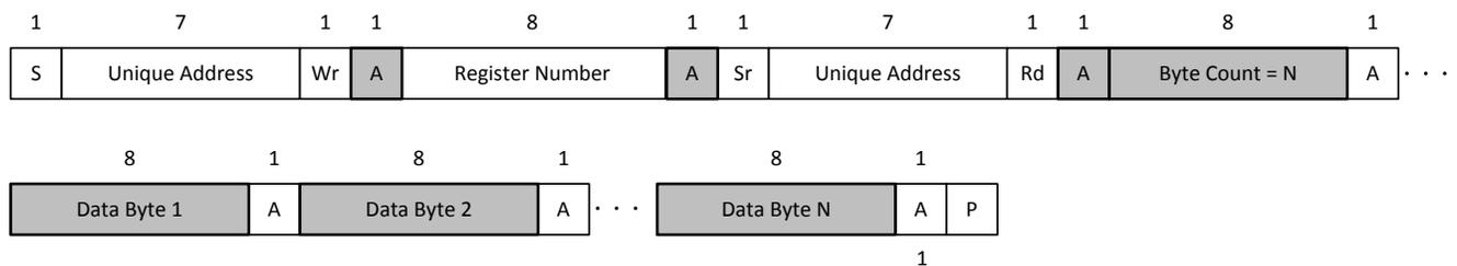
**Figure 8-39. I<sup>2</sup>C Unique Address Read Register Protocol**
