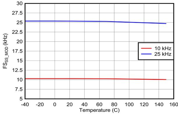
Figure 6-25.  $f_{sw}$  Dither Modulation Frequency vs Temperature
