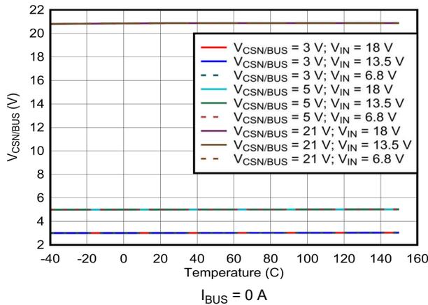
Figure 6-33. Buck-boost Output Voltage Regulation vs Temperature
