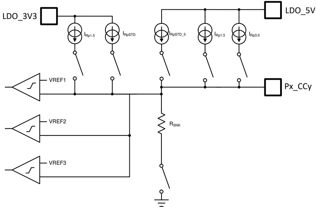
Figure 8-27. Plug and Orientation Detection Block
