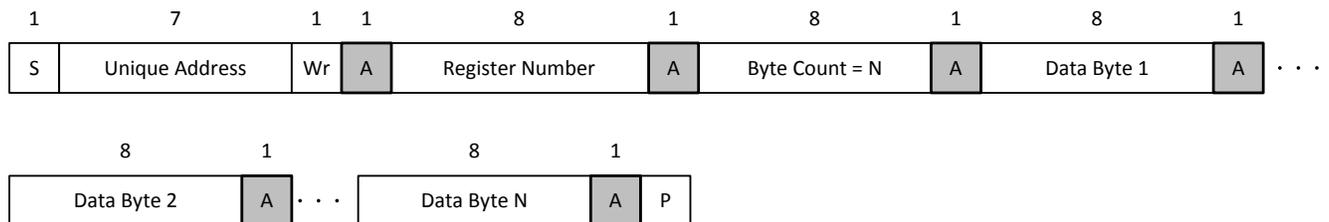
**Figure 8-38. I<sup>2</sup>C Unique Address Write Register Protocol**
