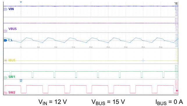
**Figure 9-25. Buck-Boost Mode: Nominal  $V_{IN}$ , No Load**
