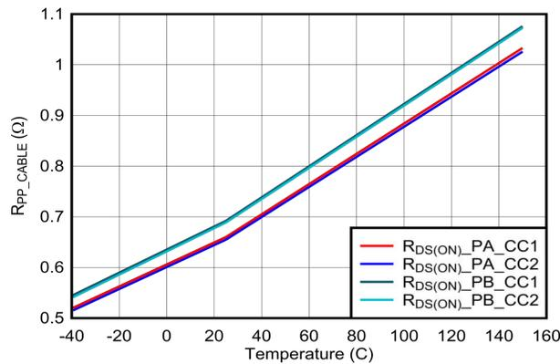
Figure 6-39.  $V_{CONN}$  Power Path:  $R_{DS(ON)}$  vs Temperature
