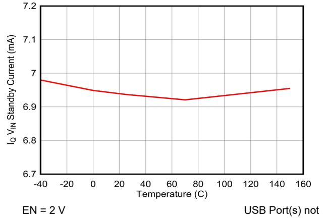
Figure 6-2.  $I_{Q\ V_{IN}}$  Standby Current vs Temperature
