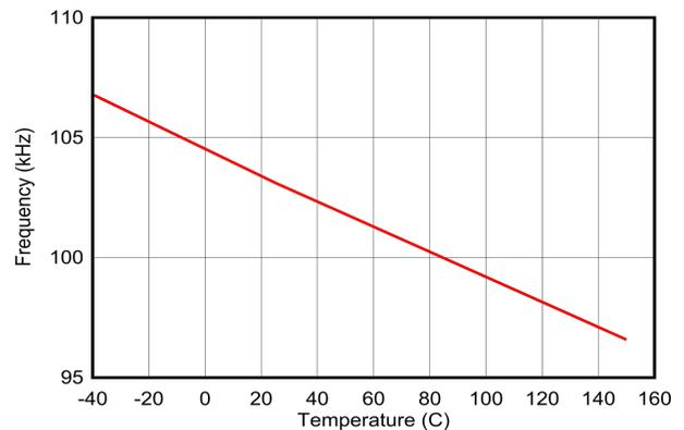
Figure 6-36. (M0) 100 kHz Oscillator vs Temperature
