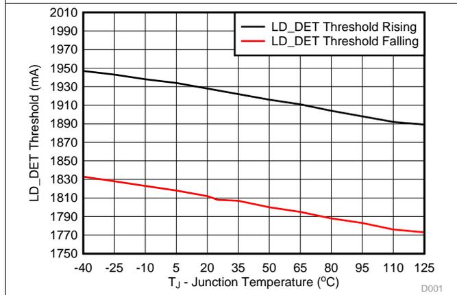
Figure 6. LD\_DET Threshold vs Temperature
