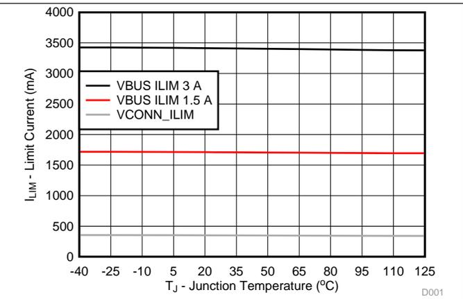
Figure 5.  $I_{LIM}$  for  $V_{BUS}$  and  $V_{CONN}$  vs Temperature
