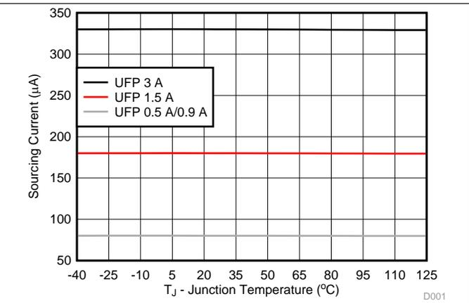
Figure 7. CC Sourcing Current to UFP vs Temperature
