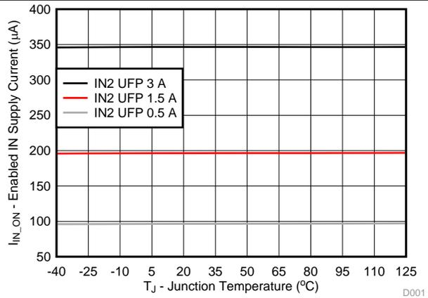
Figure 9. IN2 Current With UFP vs Temperature
