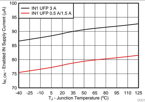
Figure 8. IN1 Current With UFP vs Temperature
