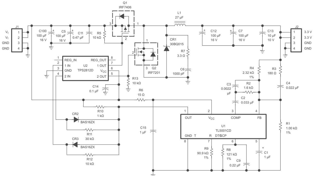
NOTE: If the parasitics of the external circuit cause the voltage to violate the Absolute Maximum Rating for the Output pins, Schottky diodes should be added from ground to output and from output to  $V_{CC}$ .
