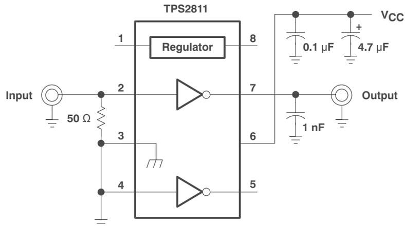
Figure 1. Test Circuit For Measurement of Switching Characteristics
