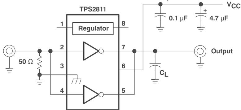
**Figure 27. Test Circuit for Measuring Paralleled Switching Characteristics**
