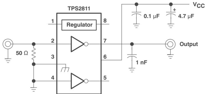
**Figure 19. Test Circuit for Measuring Switching Characteristics**
