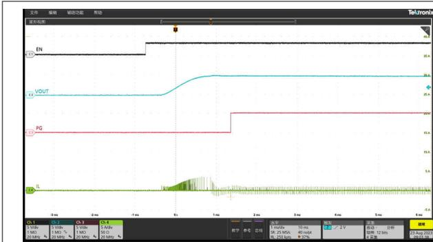
Figure 8-8. Start-Up Relative to EN Rising,  $I_{out} = 0A$ , OOA Mode
