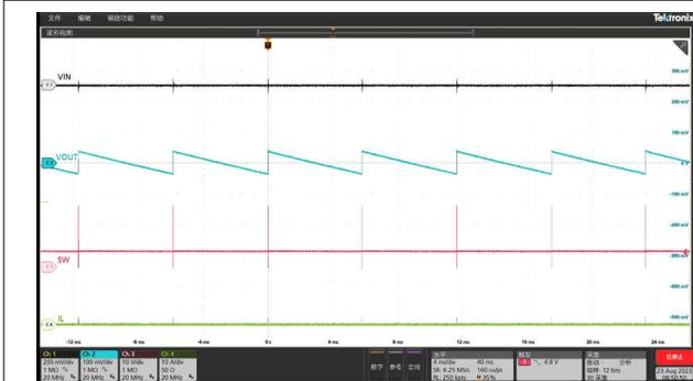
Figure 8-12. Output Voltage Ripple,  $I_{out} = 0A$ , PSM Mode
