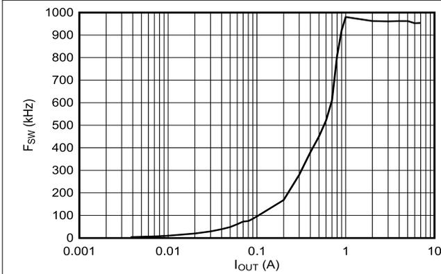
**Figure 8-4. Switching Frequency, PSM Mode**
