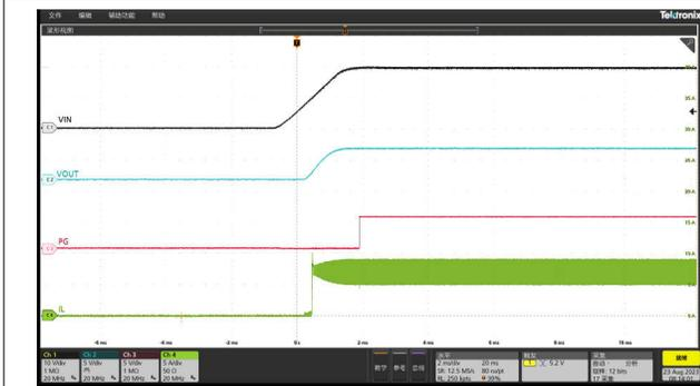
Figure 8-10. Start-Up Relative to  $V_{in}$  Rising,  $I_{out} = 7A$
