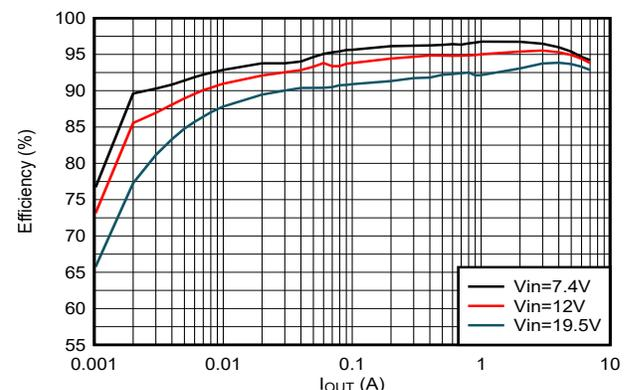
Efficiency Curve,  $V_{OUT} = 5.1$  V, PSM Mode
