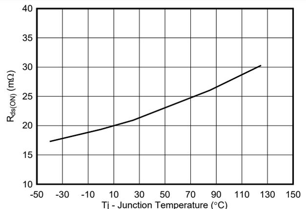
Figure 6-6. High-side R<sub>DS(on)</sub> vs Temperature
