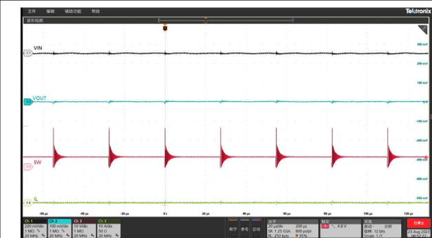
Figure 8-13. Output Voltage Ripple,  $I_{out} = 0A$ , OOA Mode
