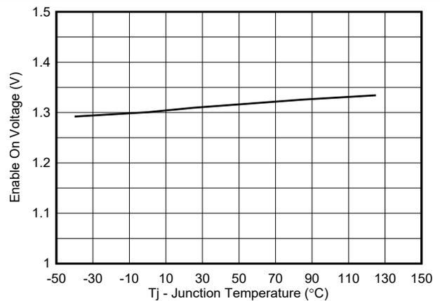
Figure 6-4. Enable On Voltage vs Temperature
