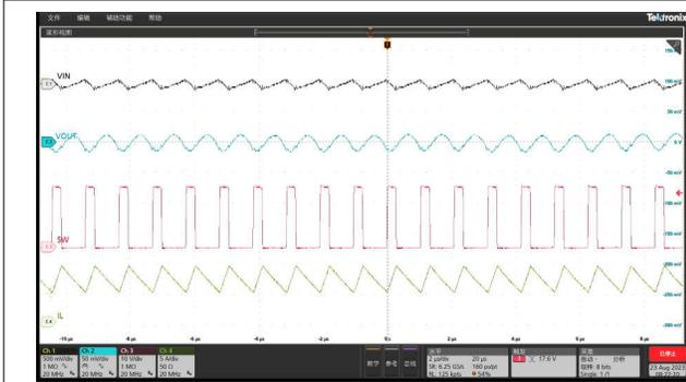
**Figure 8-14. Output Voltage Ripple, Iout = 7 A**
