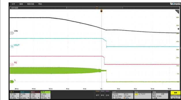
Figure 8-11. Shutdown Relative to  $V_{in}$  Falling,  $I_{out} = 7A$
