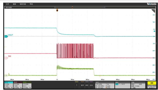
**Figure 8-17. Normal Operation to Output Hard Short**
