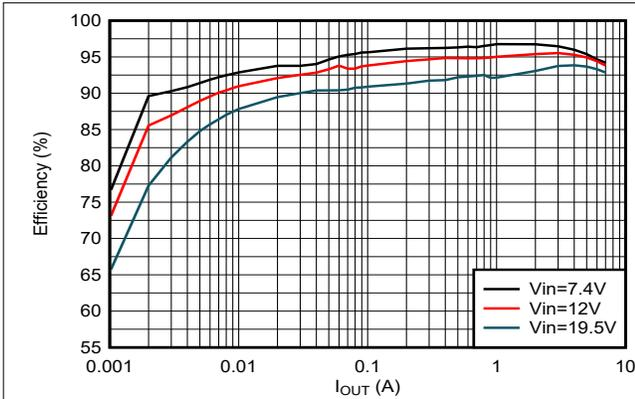
**Figure 8-2. Efficiency, PSM Mode**
