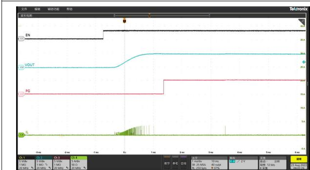
**Figure 8-6. Start-Up Relative to EN Rising, Iout = 0A, PSM Mode**
