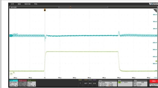
**Figure 8-16. Transient Response, 0.7 A to 6.3 A with 2.5 A/us SR**
