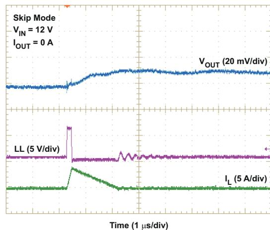
**Figure 6-18. 1.1-V Output Skip Mode Steady-State Operation**
