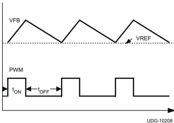
**Figure 7-2. On-Time Control Without Ramp Compensation**
