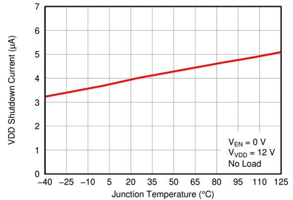
**Figure 6-2. VDD Shutdown Current vs. Junction Temperature**
