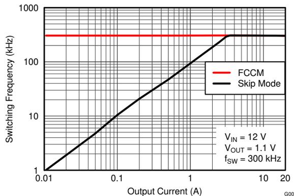
**Figure 6-5. Switching Frequency vs. Output Current**
