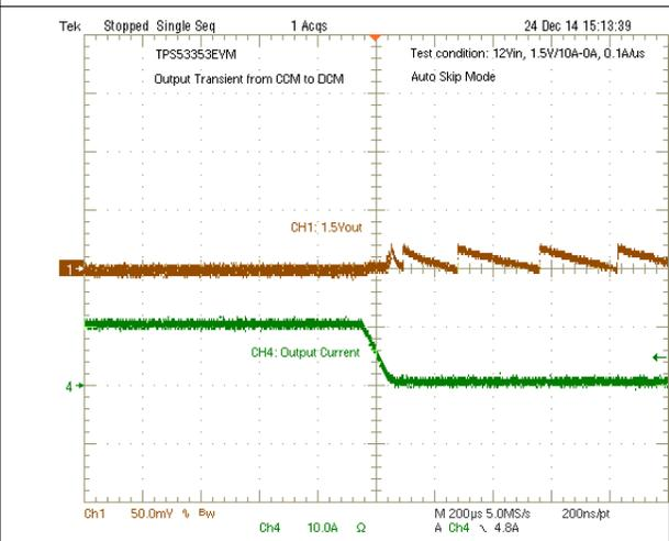
**Figure 8-8. Output Transient from DCM to DCM**
