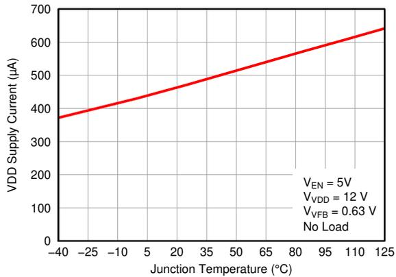
**Figure 6-1. VDD Supply Current vs. Junction Temperature**
