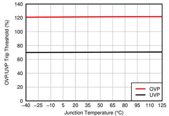
**Figure 6-4. OVP/UVP Trip Threshold vs. Junction Temperature**
