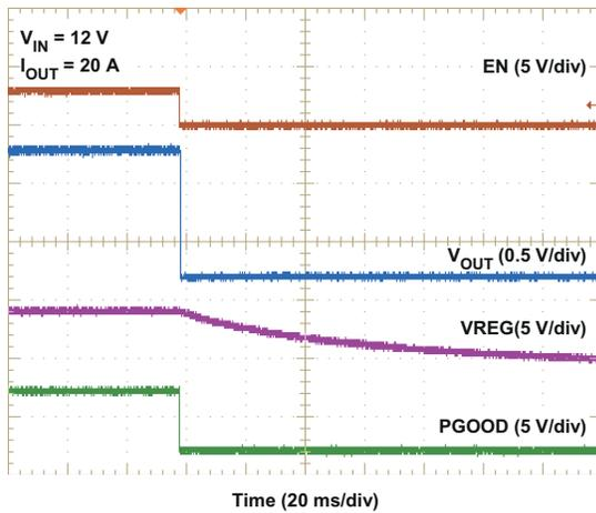
**Figure 6-15. Shutdown Waveforms**
