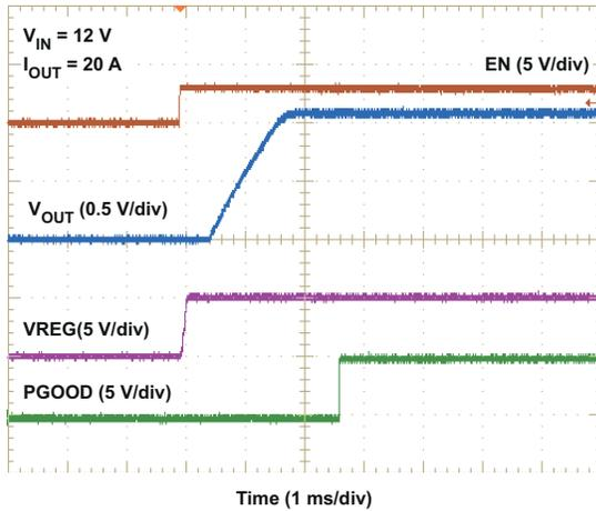
**Figure 6-13. Start-Up Waveforms**
