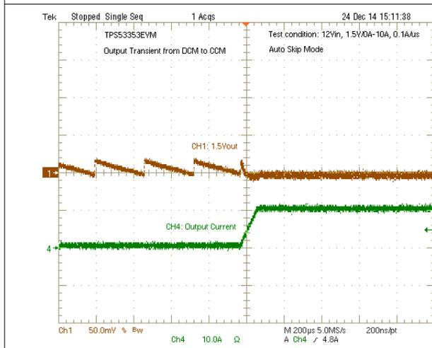
**Figure 8-7. Output Transient from DCM to CCM**
