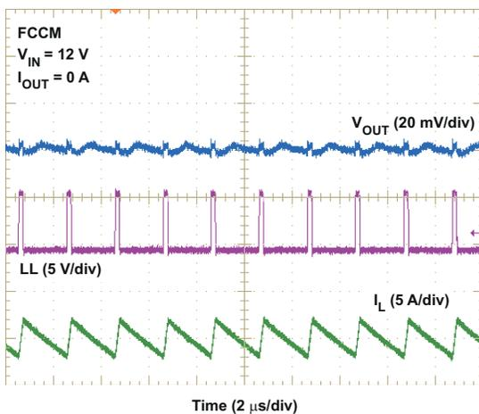
**Figure 6-17. 1.1-V Output FCCM Mode Steady-State Operation**
