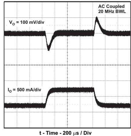
**Figure 18. Transient Response,  $I_O$  Step 0.25 to 0.75 A**
