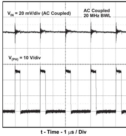
Figure 25. Output Voltage Ripple and PH Node,  $I_o = 1$  A
