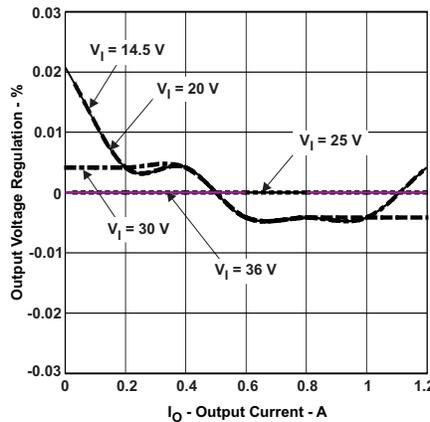
**Figure 14. Output Voltage Regulation % vs. Output Current**
