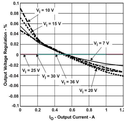
Figure 22. Output Voltage Regulation % vs. Output Current
