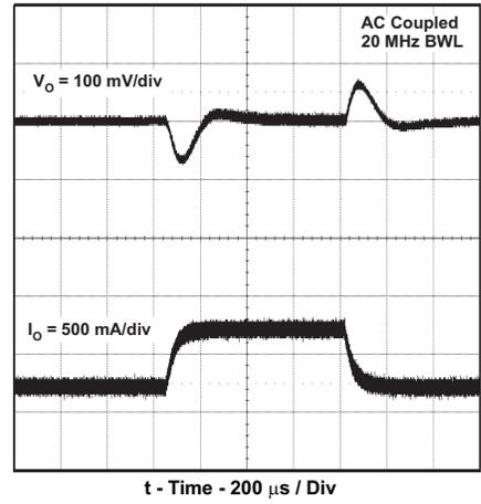
Figure 26. Transient Response,  $I_o$  Step 0.25 to 0.75 A
