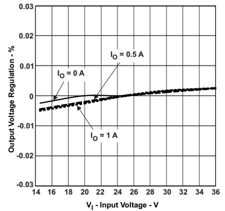
**Figure 15. Output Voltage Regulation % vs. Input Voltage**
