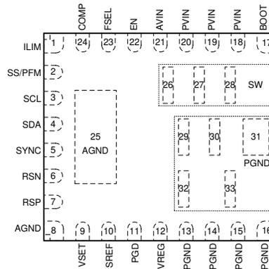
**Figure 5-1. 33-Pin VQFN RJM Package (Top View)**
