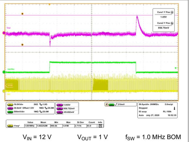
Figure 6-26. Load Transient 2 A to 12 A to 2 A at 20 A/µs
