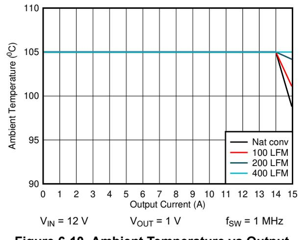
**Figure 6-10. Ambient Temperature vs Output Current**
