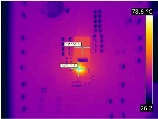
$V_{IN} = 12\text{ V}$      $V_{OUT} = 1\text{ V}$      $f_{SW} = 1\text{ MHz}$
