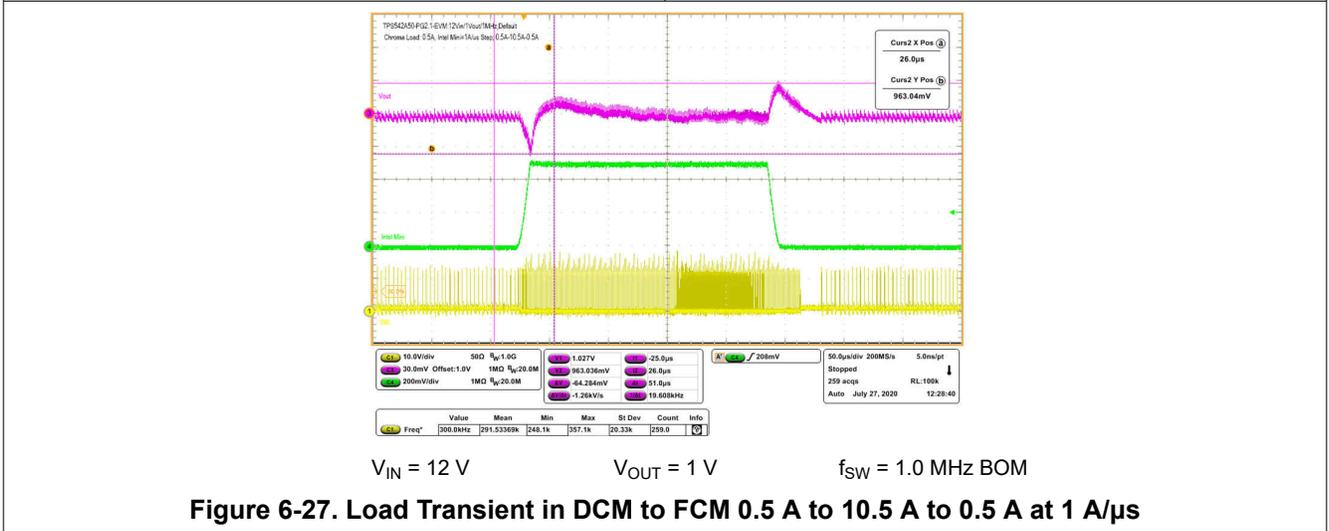
Figure 6-27. Load Transient in DCM to FCM 0.5 A to 10.5 A to 0.5 A at 1 A/µs
