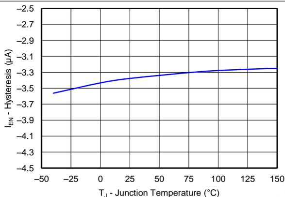
Figure 13. EN Terminal Current Hysteresis vs Junction Temperature
