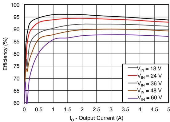
Figure 48. Efficiency vs Output Current
