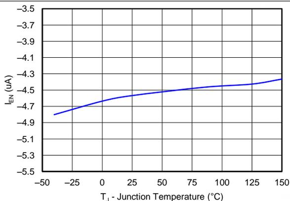
Figure 11. EN Terminal Current vs Junction Temperature
