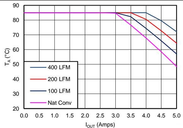
**Figure 55. Air Flow Conditions
