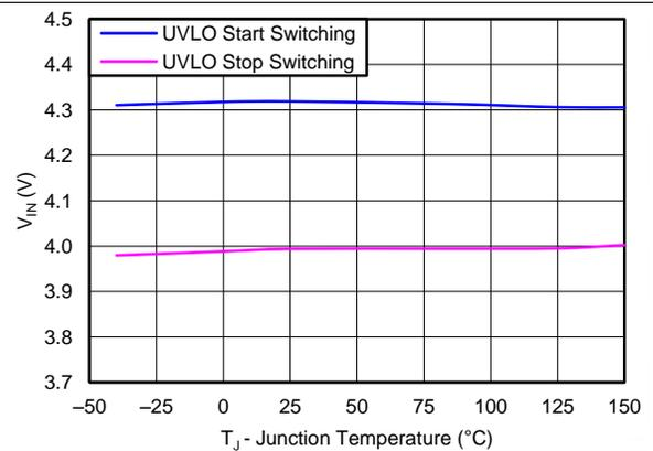
Figure 20. Input Voltage UVLO vs Junction Temperature
