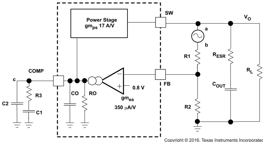
Figure 29. Small Signal Model for Loop Response
