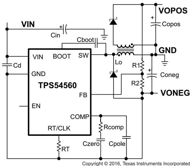
Figure 57. TPS54560 Split Rail Power Supply
