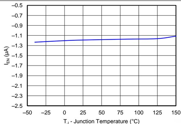
Figure 12. EN Terminal Current vs Junction Temperature
