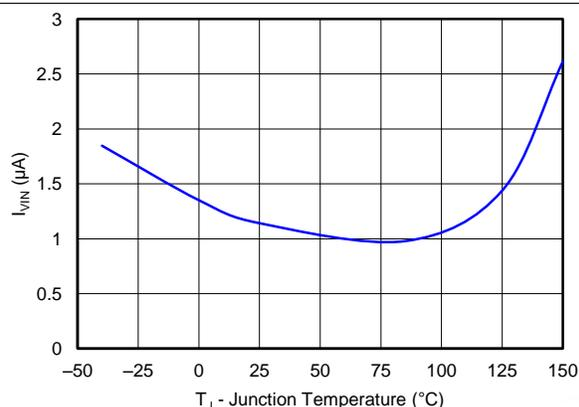
Figure 15. Shutdown Supply Current vs Junction Temperature
