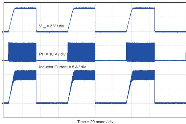
Figure 45. Hiccup Mode Current Limit
