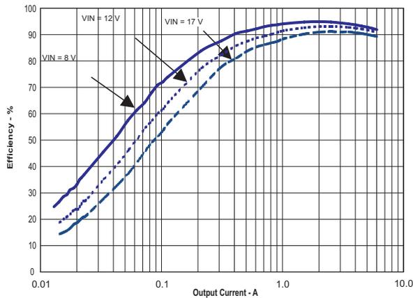
Figure 44. Efficiency vs Load Current
