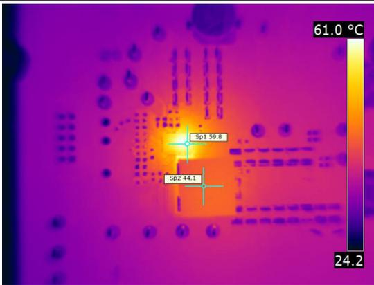
$V_{IN} = 12\text{ V}$   $f_{SW} = 650\text{ kHz}$   $I_{OUT} = 40\text{ A}$
