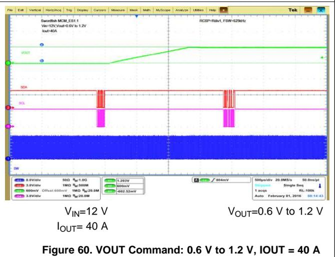
Figure 60. VOUT Command: 0.6 V to 1.2 V, IOUT = 40 A
