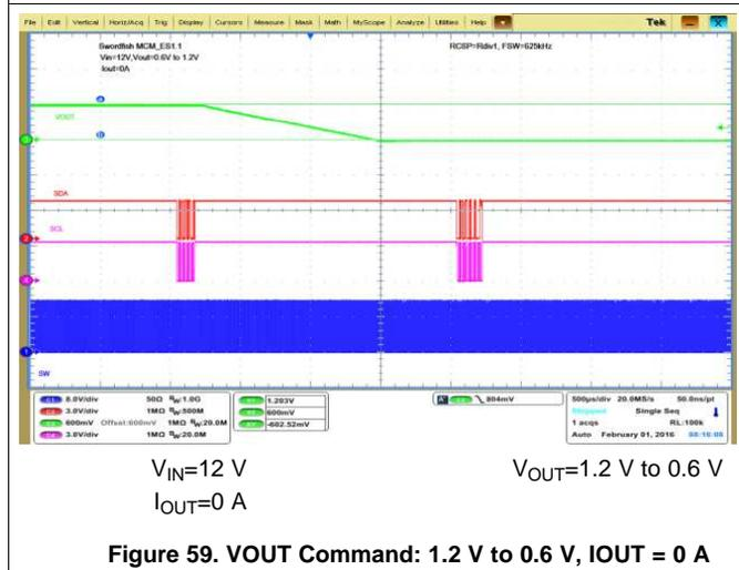
Figure 59. VOUT Command: 1.2 V to 0.6 V, IOUT = 0 A
