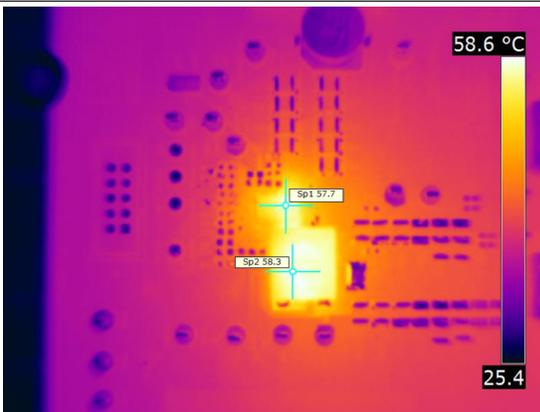
$V_{IN} = 12\text{ V}$   $f_{SW} = 425\text{ kHz}$   $I_{OUT} = 30\text{ A}$
