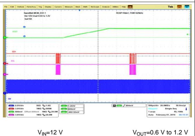
Figure 58. VOUT Command: 0.6 V to 1.2 V, IOUT = 0 A
