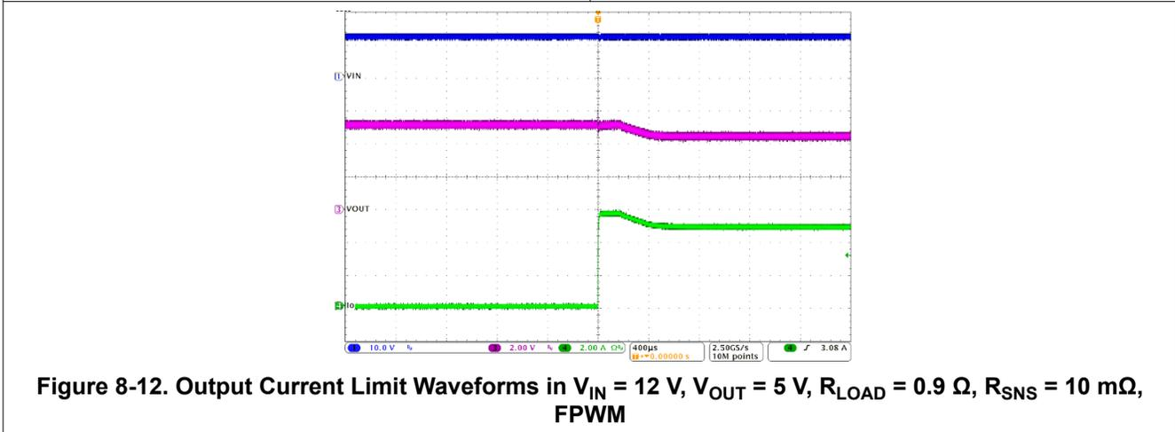
Figure 8-12. Output Current Limit Waveforms in  $V_{IN} = 12\text{ V}$ ,  $V_{OUT} = 5\text{ V}$ ,  $R_{LOAD} = 0.9\ \Omega$ ,  $R_{SNS} = 10\text{ m}\Omega$ , FPWM
