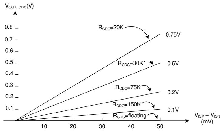
Figure 7-6. Output Voltage Rise versus Output Current
