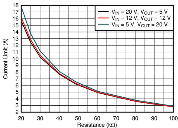
Figure 6-11. Average Inductor Current Limit vs Setting Resistance
