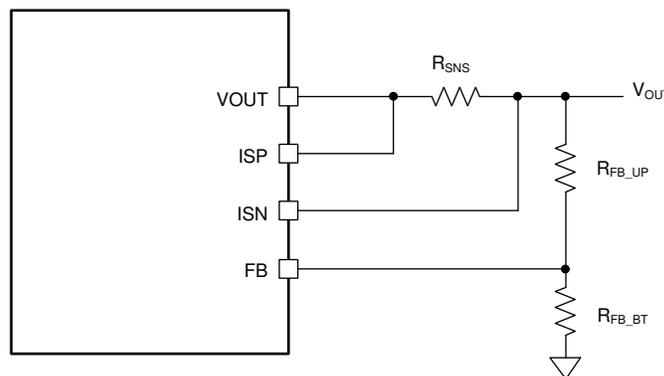
Figure 7-5. Output Voltage Setting by External Resistor Divider
