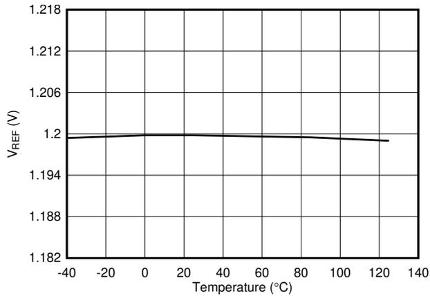
Figure 6-13. Reference Voltage vs Temperature ( $V_{REF} = 1.2\text{ V}$ )
