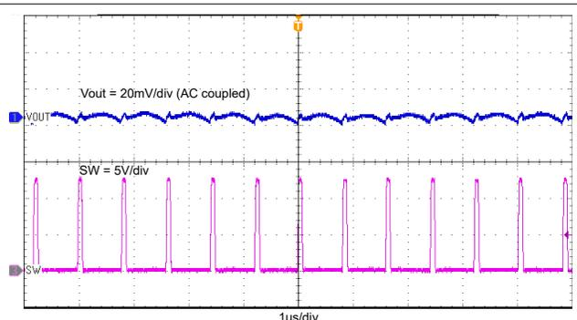
**Figure 8-7. Output Voltage Ripple with 2-A Loading**
