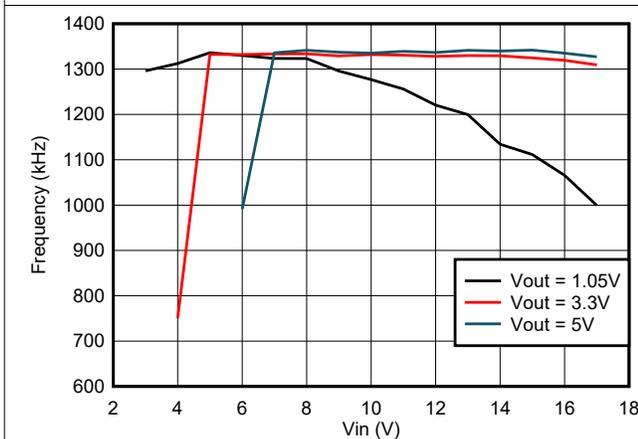
Figure 6-11. Frequency vs Input Voltage,  $I_{OUT} = 2\text{ A}$
