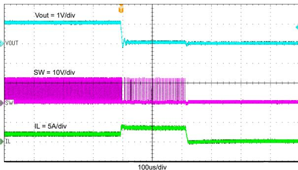
**Figure 8-14. Normal Operation to Output Hard Short**
