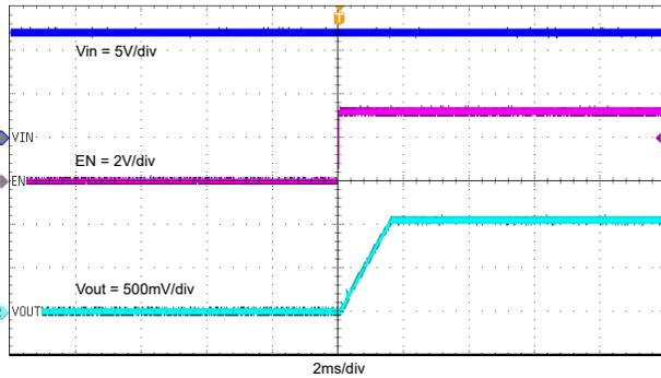
**Figure 8-8. Start-up Through EN,  $I_{OUT} = 2\text{ A}$**
