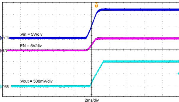
**Figure 8-10. Start-up with  $V_{IN}$  Rising,  $I_{OUT} = 2\text{ A}$**
