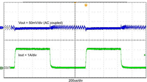
**Figure 8-13. Transient Response with 0.01 A to 2 A**
