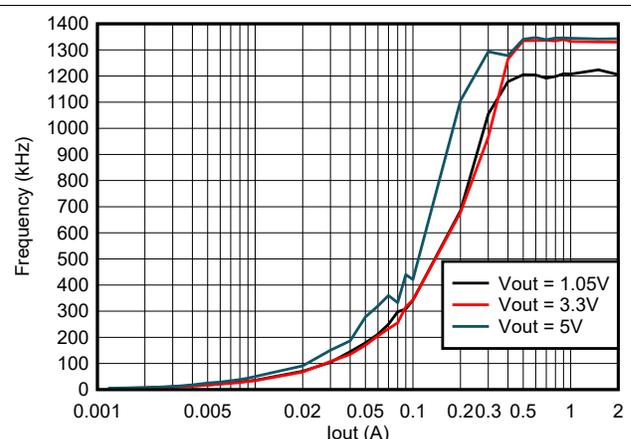
Figure 6-12. Frequency vs Loading,  $V_{IN} = 12\text{ V}$
