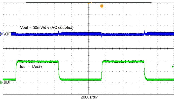
**Figure 8-12. Transient Response with 0.2 A to 1.8 A**
