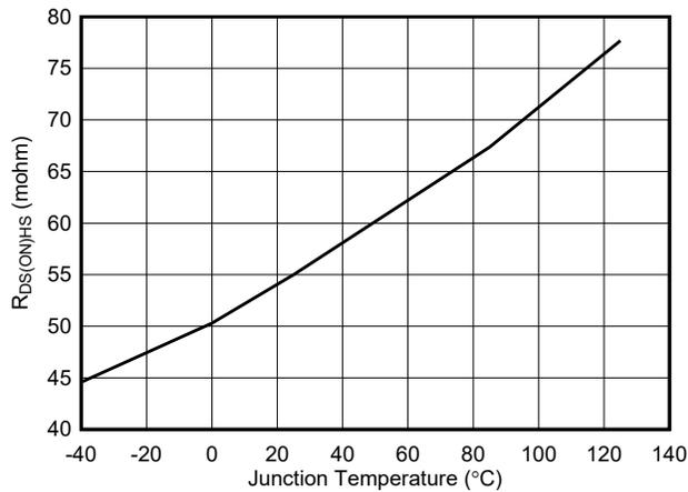
Figure 6-5. High-Side  $R_{DS(on)}$
