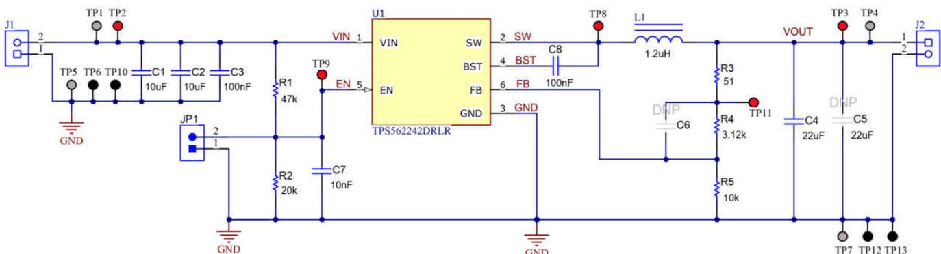
**Figure 8-1. Schematic**
