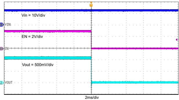
**Figure 8-9. Shutdown Through EN,  $I_{OUT} = 2\text{ A}$**
