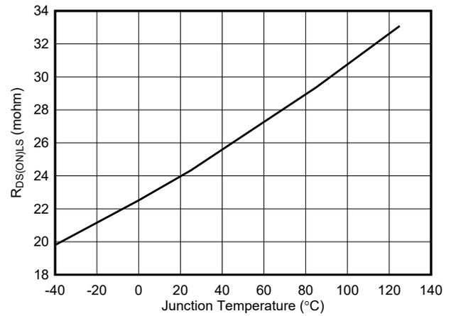
Figure 6-4. Low-Side  $R_{DS(on)}$
