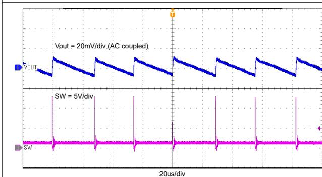
**Figure 8-6. Output Voltage Ripple with 0.01-A Loading**
