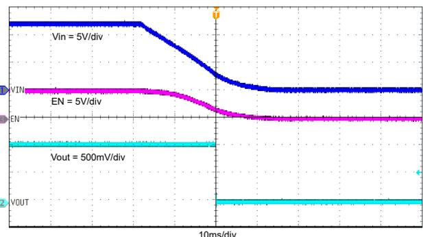
**Figure 8-11. Shutdown with  $V_{IN}$  Falling,  $I_{OUT} = 2\text{ A}$**
