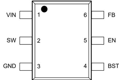
**Figure 5-1. 6-Pin SOT563 DRL Package (Top View)**
