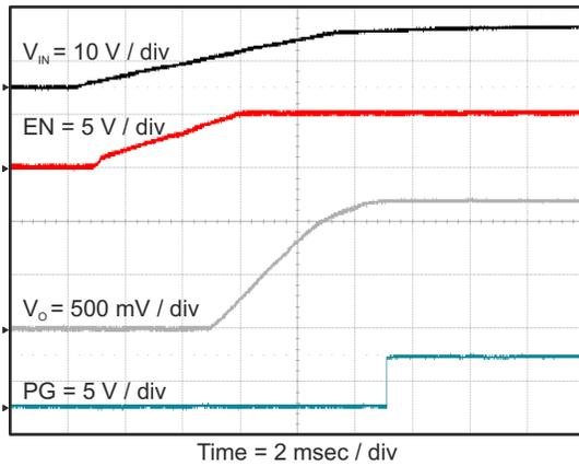
**Figure 8-14. Start Up Relative to  $V_{IN}$  Rising**
