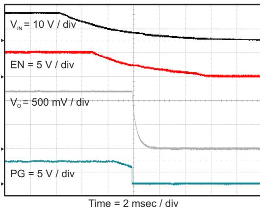
**Figure 8-16. Shut Down Relative to  $V_{IN}$  Falling**
