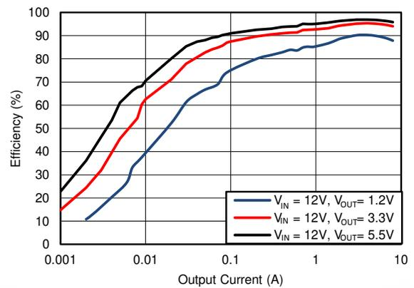
Figure 6-12. Efficiency, Mode = DCM,  $F_{SW} = 400kHz$
