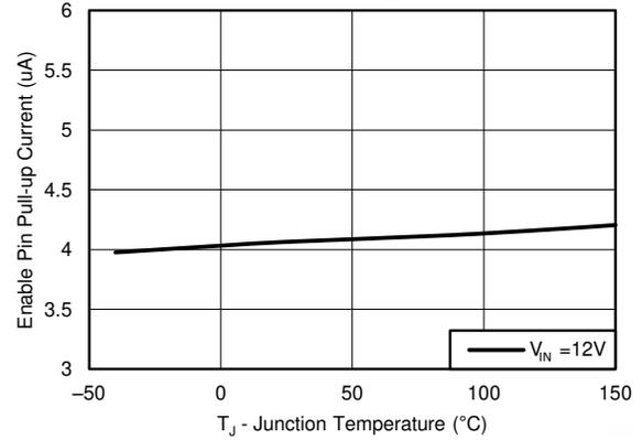
Figure 6-8. Enable Pull-Up Current,  $V_{EN} = 1.3V$
