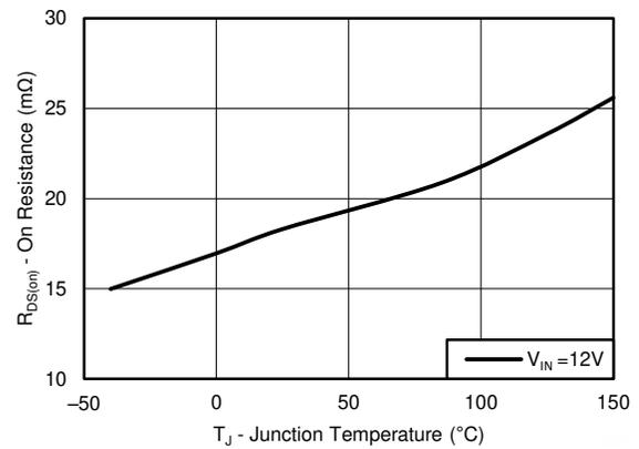
Figure 6-4. High-side R<sub>ds(on)</sub> vs Temperature
