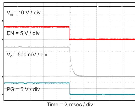
**Figure 8-17. Shut Down Relative to EN Falling**
