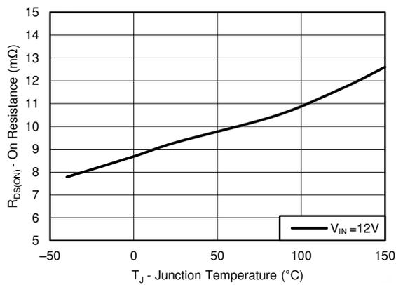
Figure 6-5. Low-side R<sub>ds(on)</sub> vs Temperature
