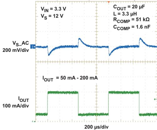
Figure 11. Load Transient Response High Frequency (1.2 MHz)
