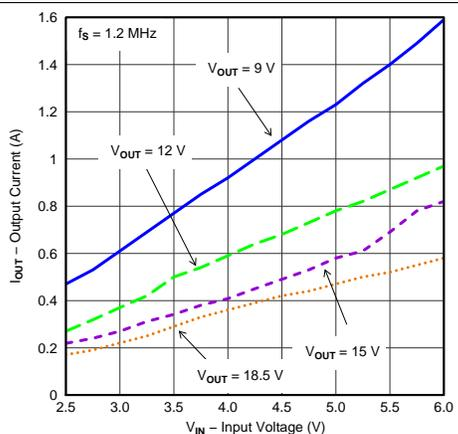
Figure 1. Maximum Load Current vs Input Voltage
