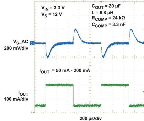
Figure 12. Load Transient Response Low Frequency (650 kHz)
