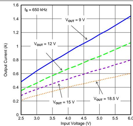
Figure 2. Maximum Load Current vs Input Voltage
