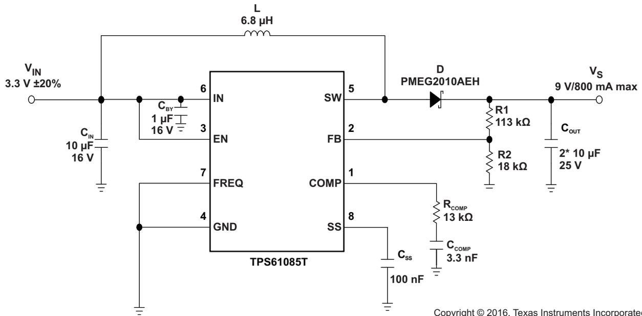
**Figure 16. Typical Application, 3.3 V to 9 V ( $f_{sw} = 650$  kHz)**
