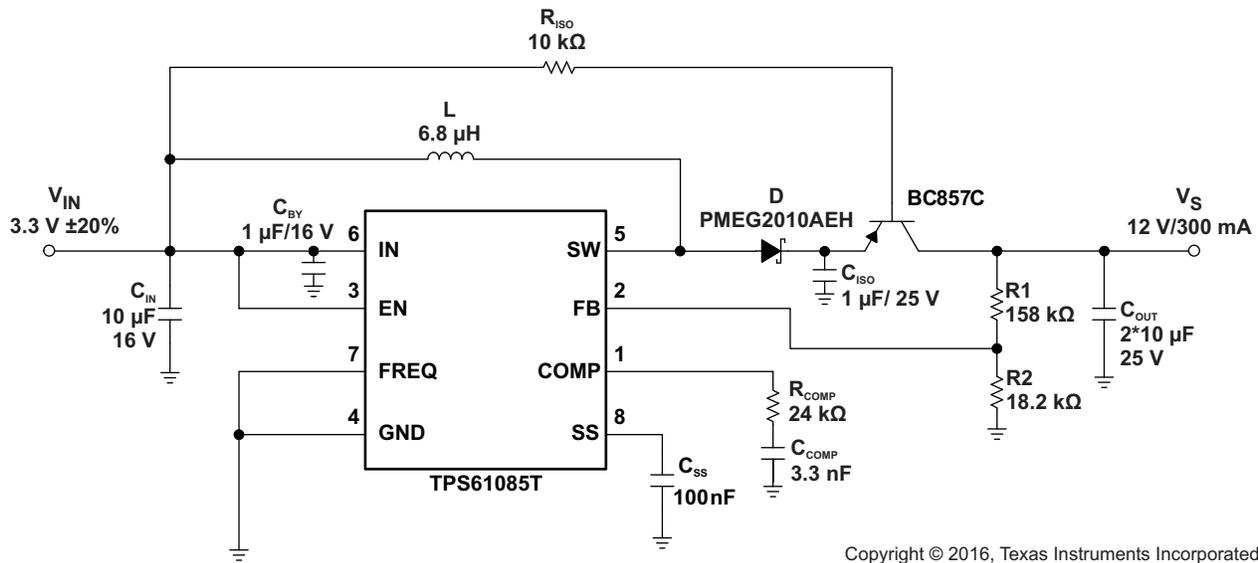
**Figure 17. Typical Application With External Load Disconnect Switch**
