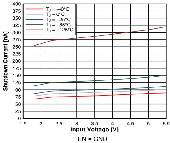
**Figure 6-1. Shutdown Current  $I_{SD}$**
