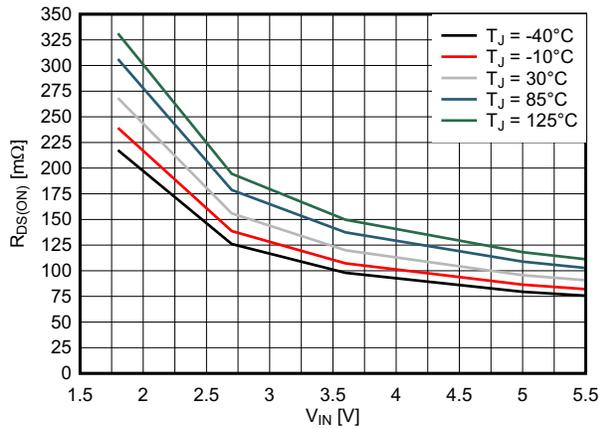
**Figure 6-3. High-side Switch Drain Source Resistance  $R_{DS(ON)}$**
