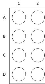
Figure 5-1. 8-Pin DSBGA YCH Package (Top View)
