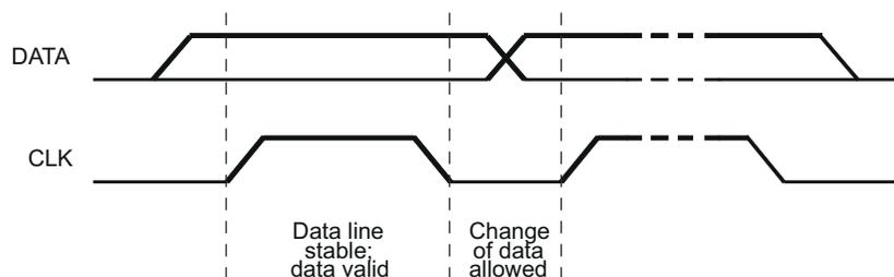
**Figure 7-4. Bit Transfer on the Serial Interface**
