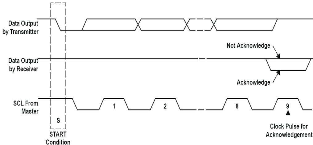
**Figure 7-5. Acknowledge on the I<sup>2</sup>C Bus**
