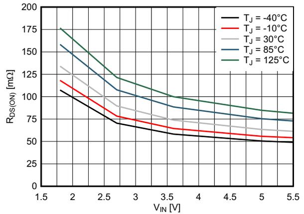
**Figure 6-4. Low-side Switch Drain Source Resistance  $R_{DS(ON)}$**
